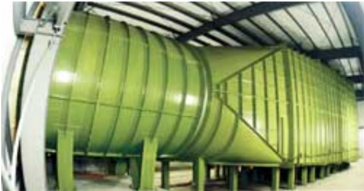
Figure 3.3 – Fire Research Wind Tunnel, used by Building Research Institute, Japan.
