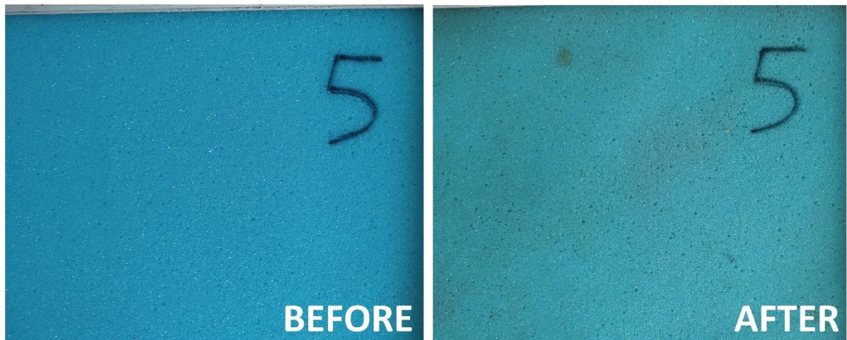
Figure 4.8 – Test run 9 – 5mm thick foam against 600 grams eucalyptus embers.
