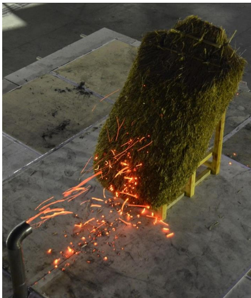
Figure 3.2 – Testing a sample of water reed thatched roof with NIST Fire Brand Generator.
