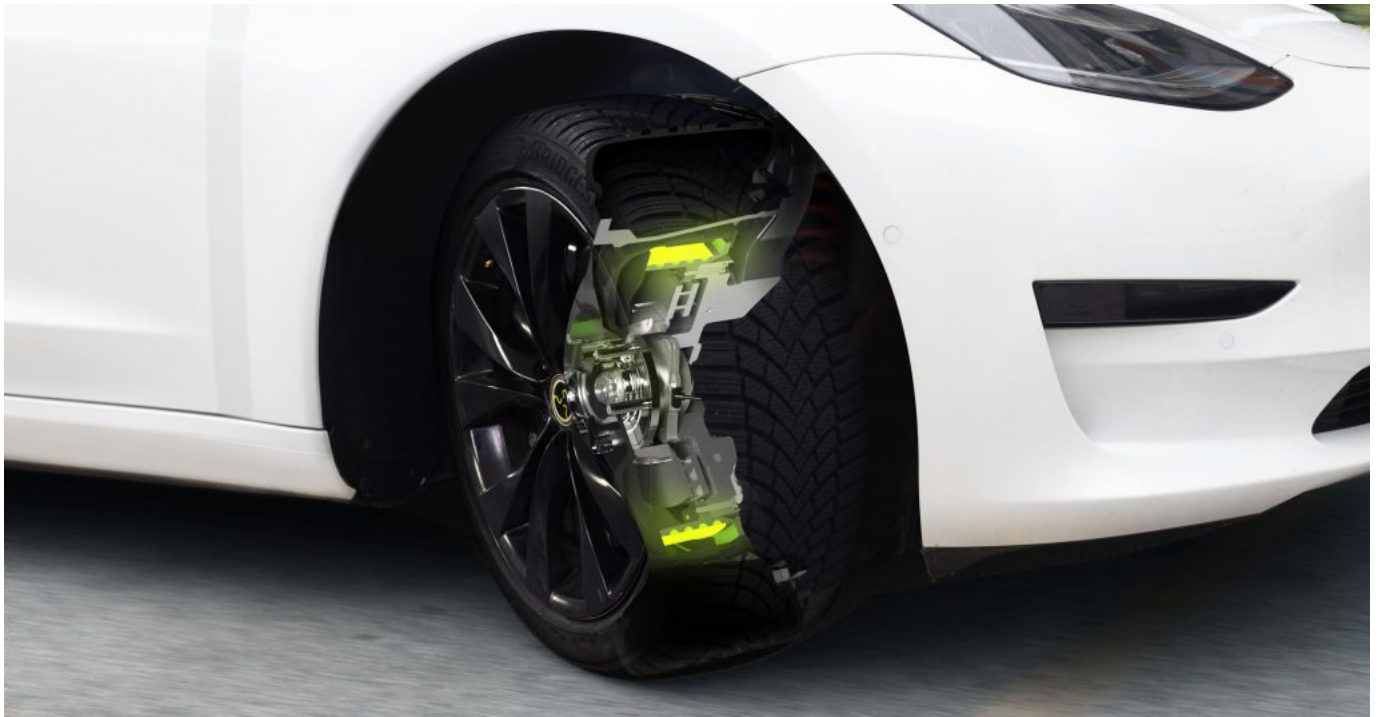
Figure 3: Above is an example of an in-wheel-hub motor would be mounted as shown above (Elaphe, 2023). This is a possible motor / generator that could be used to verify the feasibility of this thesis.
