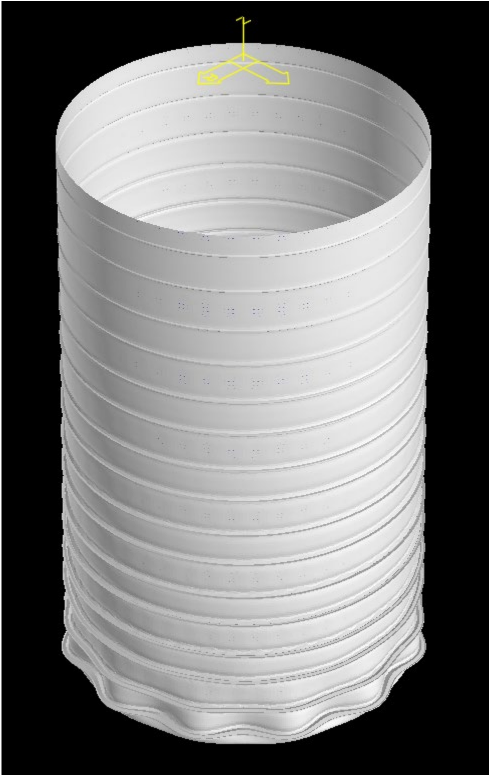
Figure 95: Upper-lower case for 1.2mm thickness, 3.6m diameter meal silo. Isometric View.
