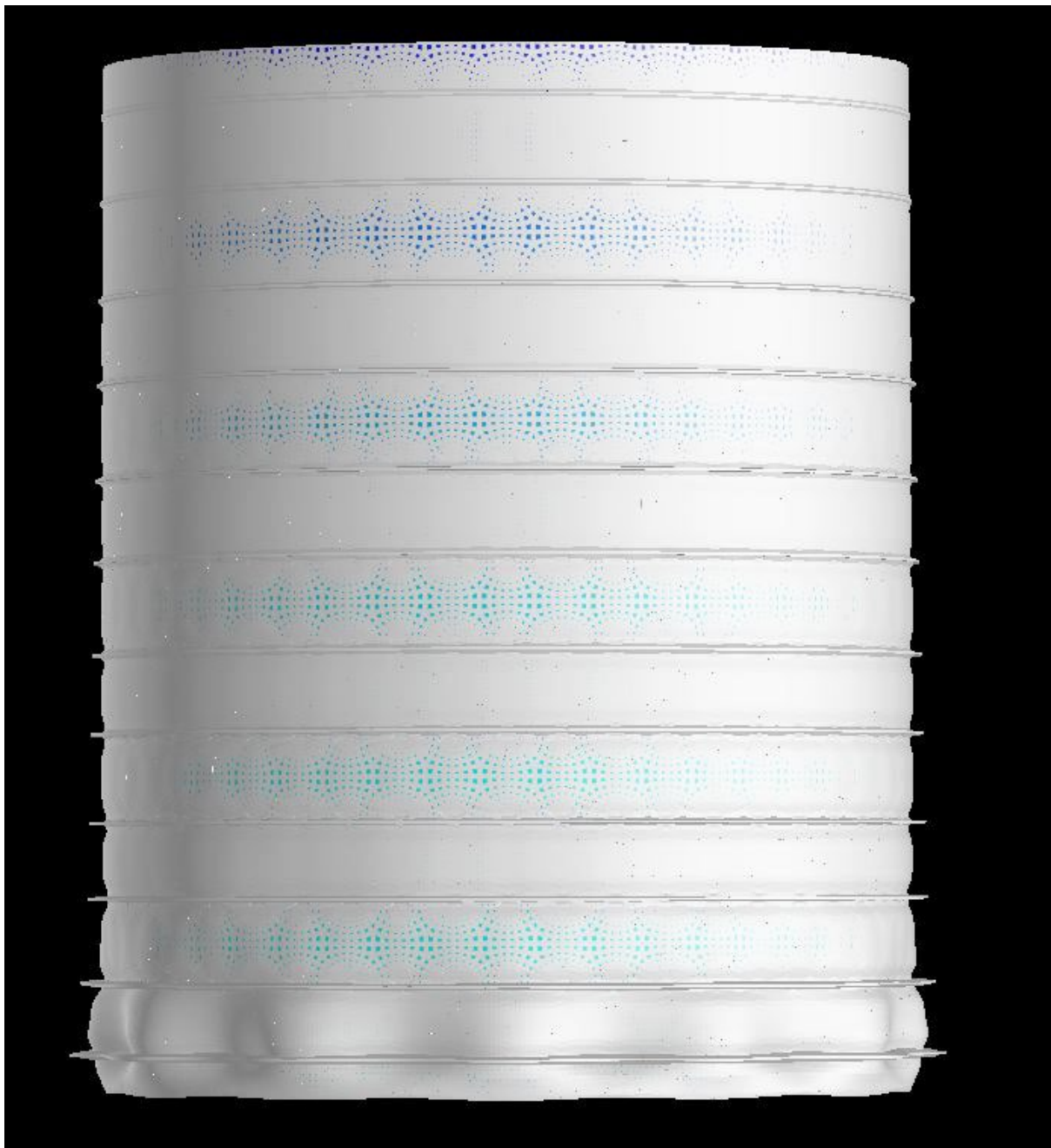
Figure 23: The deflection of the 1.0mm thick, 3.6m diameter wheat silo at 5% scale for the upper-lower case.
