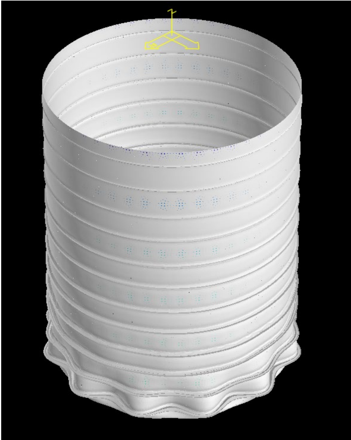
Figure 87: Upper-lower case for 1.35mm thickness, 3.6m diameter wheat silo. Isometric View.
