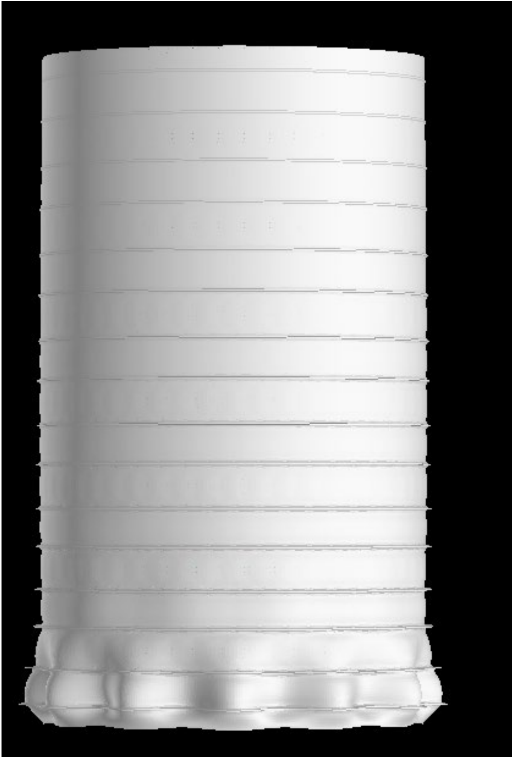
Figure 98: Upper-lower case for 1.5mm thickness, 3.6m diameter meal silo.
