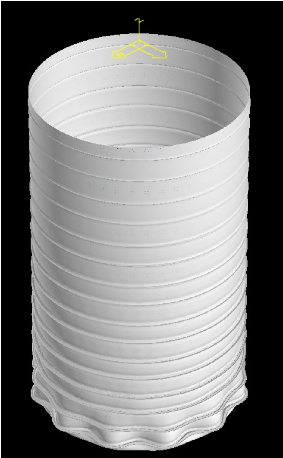
Figure 97: Upper-lower case for 1.4mm thickness, 3.6m diameter meal silo. Isometric View.
