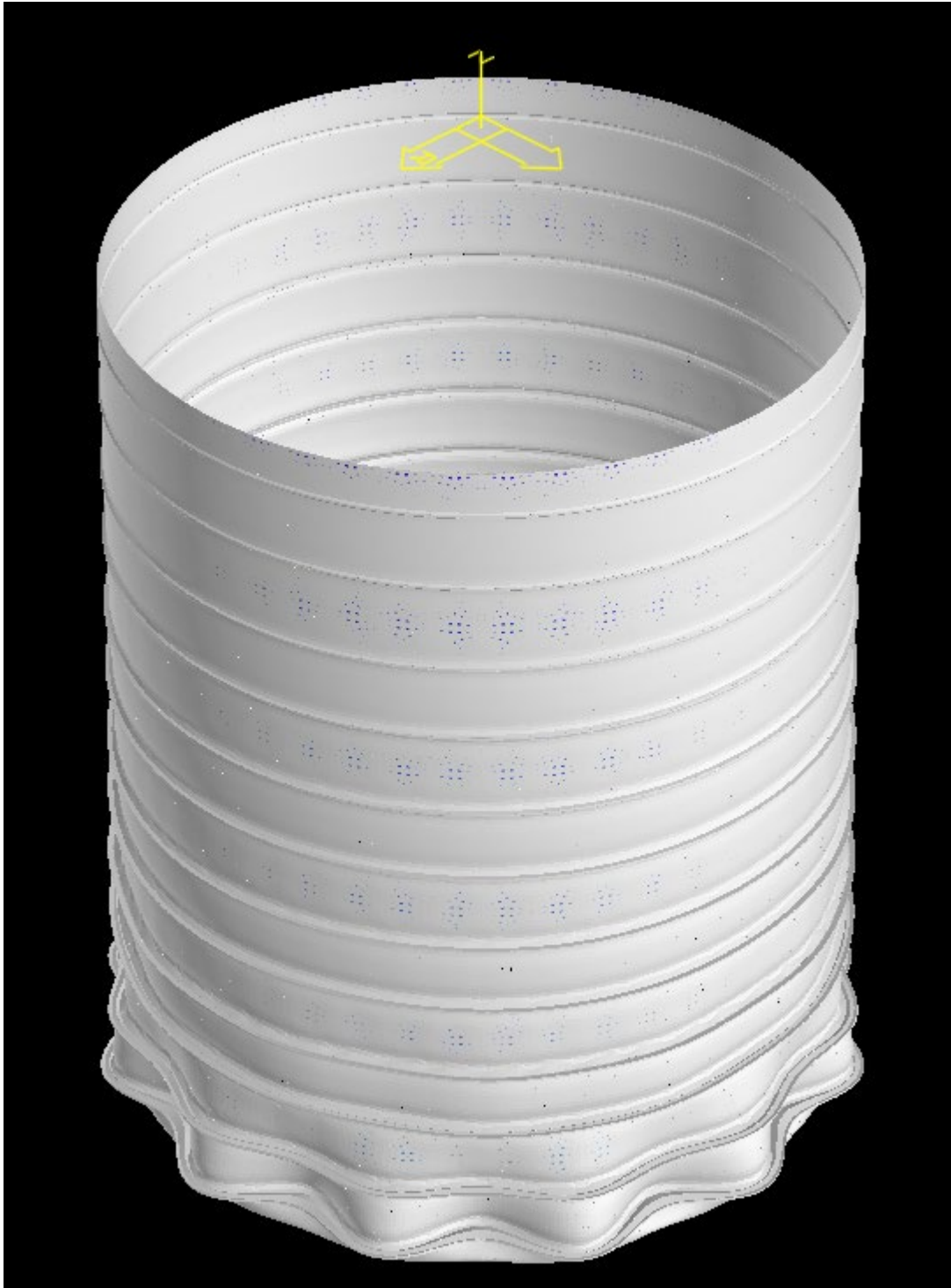
Figure 89: Upper-lower case for 1.4mm thickness, 3.6m diameter wheat silo. Isometric View.
