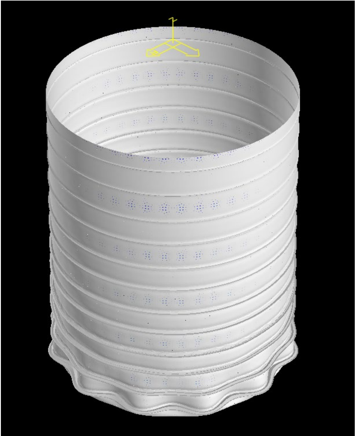
Figure 85: Upper-lower case for 1.2mm thickness, 3.6m diameter wheat silo. Isometric View.
