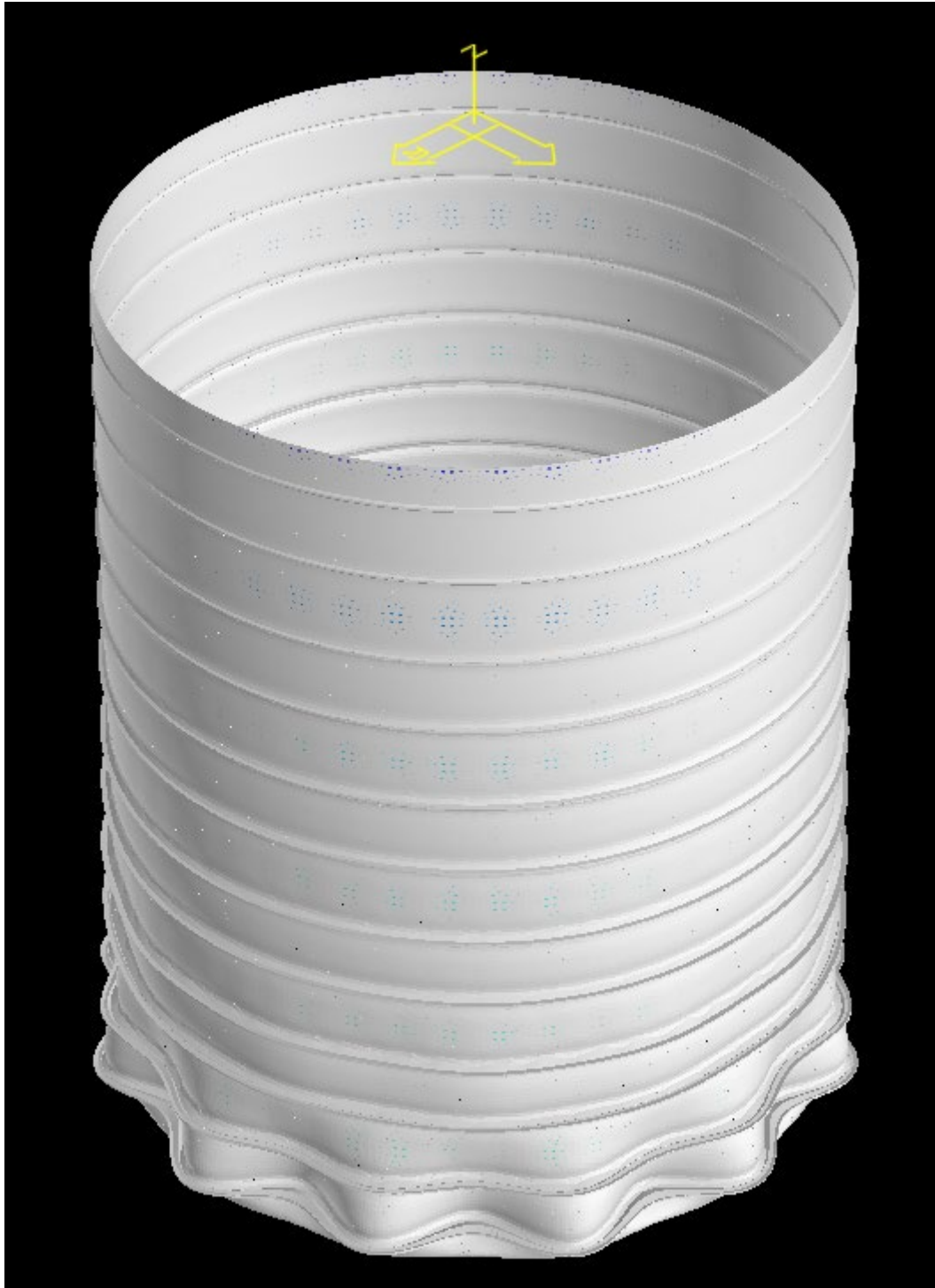
Figure 25: From an isometric view, the deflection of the 1.0mm thick, 3.6m diameter wheat silo at 5% scale for the upper-lower case.
