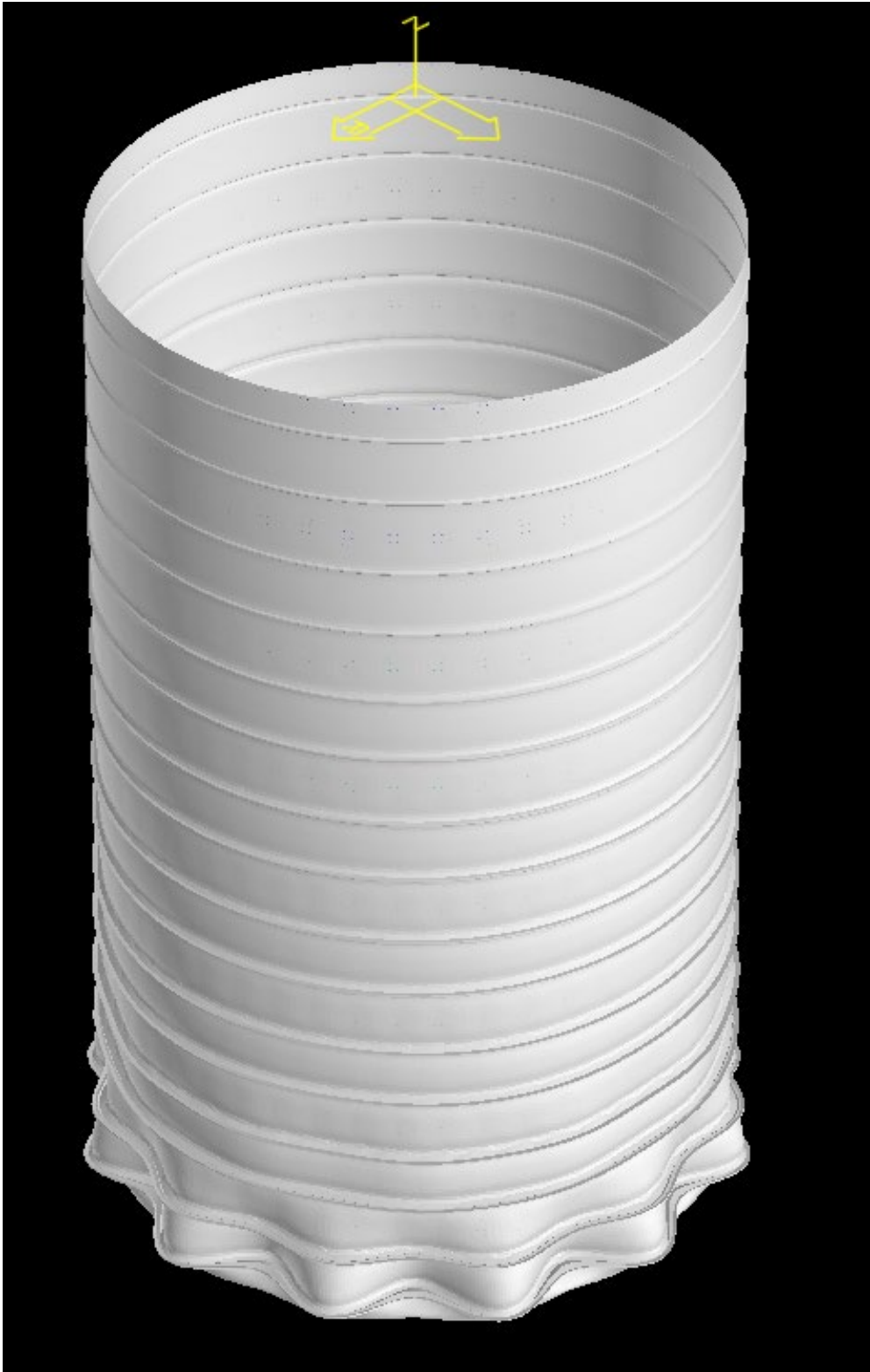
Figure 99: Upper-lower case for 1.5mm thickness, 3.6m diameter meal silo. Isometric View.
