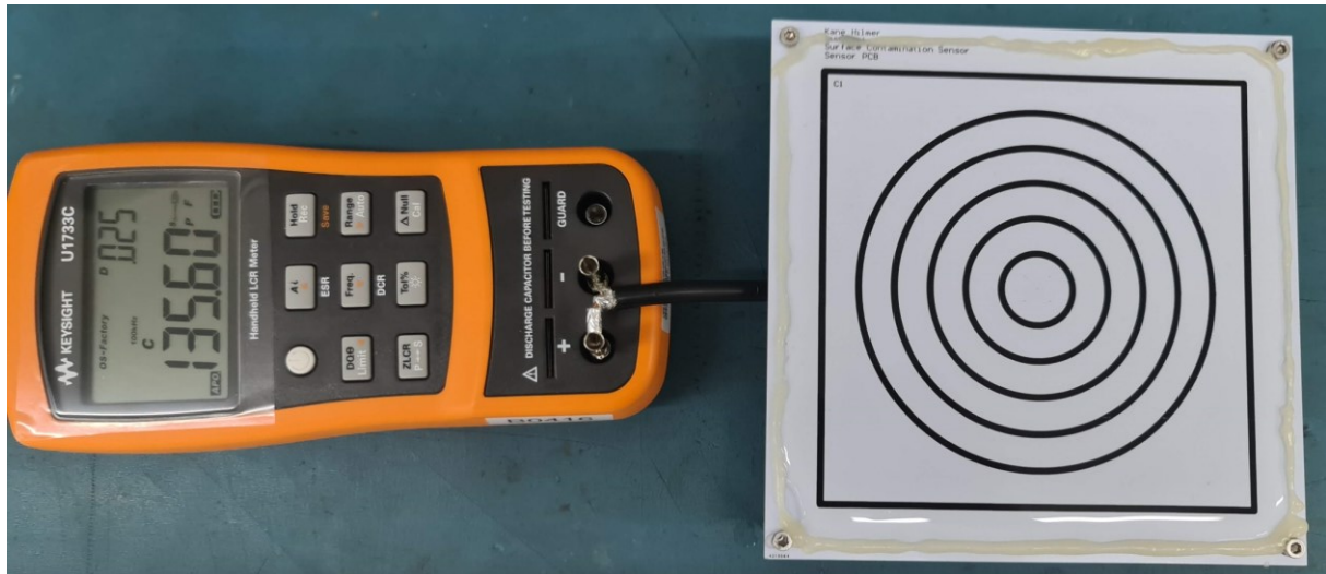
Figure 74 LCR Meter PCB Sensor Wet Capacitance Measurement
