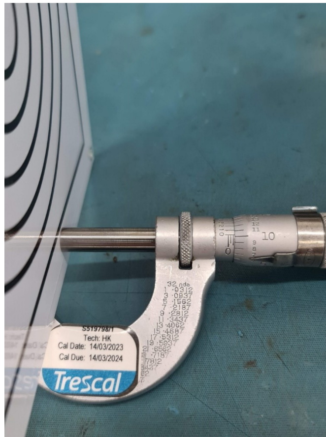
Figure 60 Imperial Micrometre Measurement of PCB
