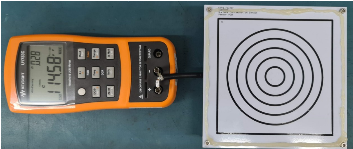
Figure 73 LCR Meter PCB Sensor Dry Capacitance Measurement
