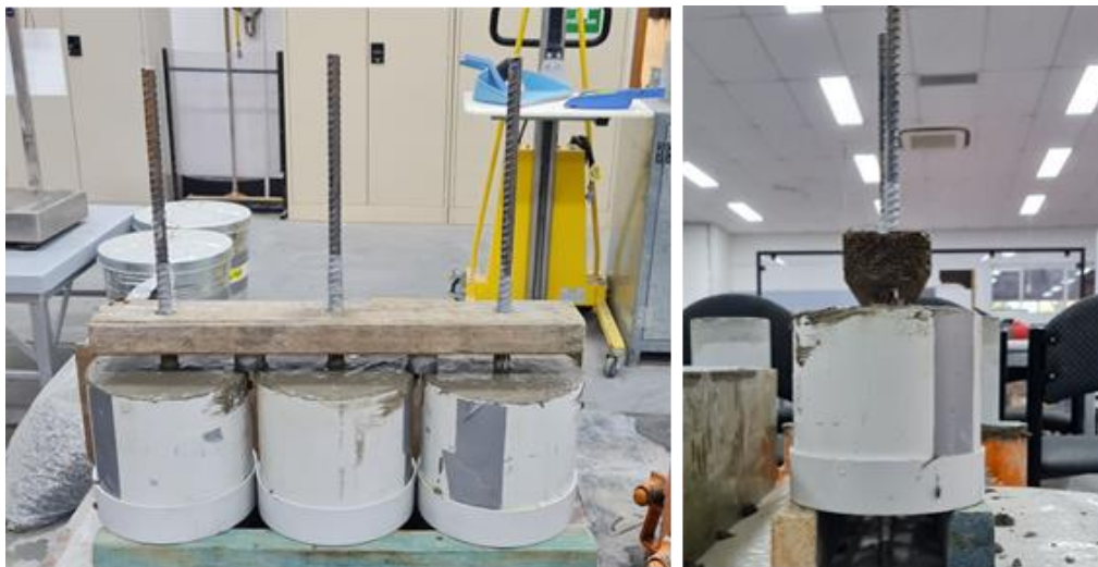
Figure 3.8: Casting of pull-out test samples
