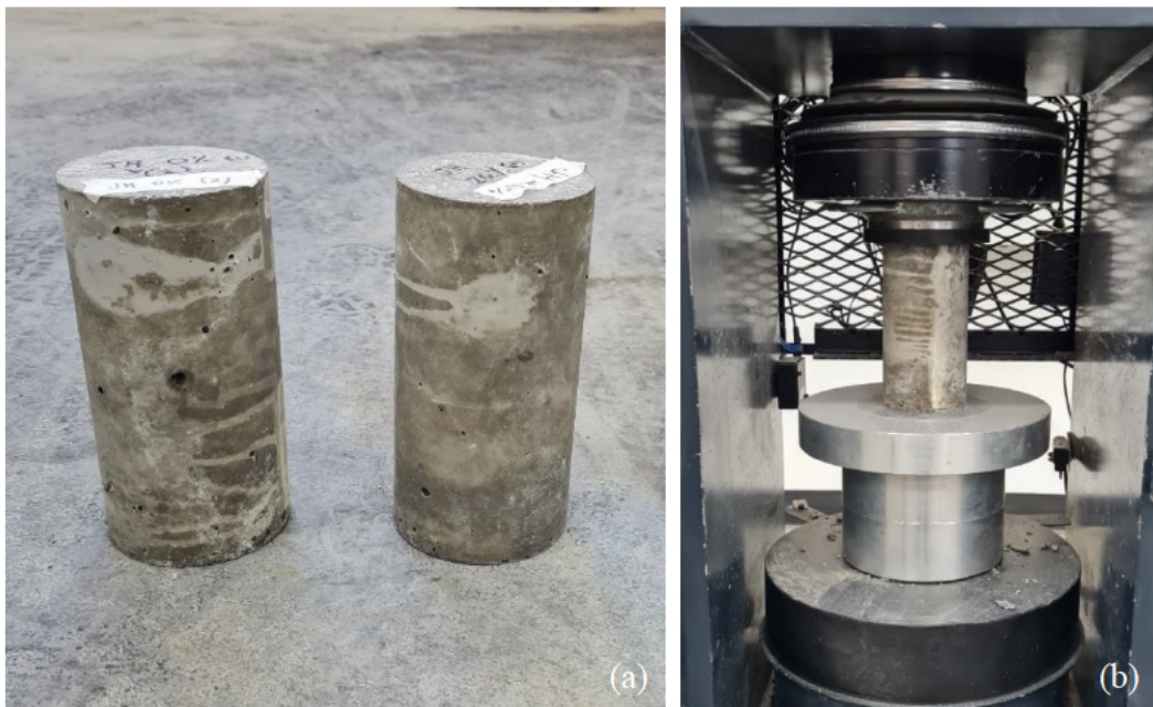
Figure 3.10: (a) concrete compression samples (b) test setup
