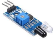
Figure 42: Infrared sensor used in the design of the bee counters.
