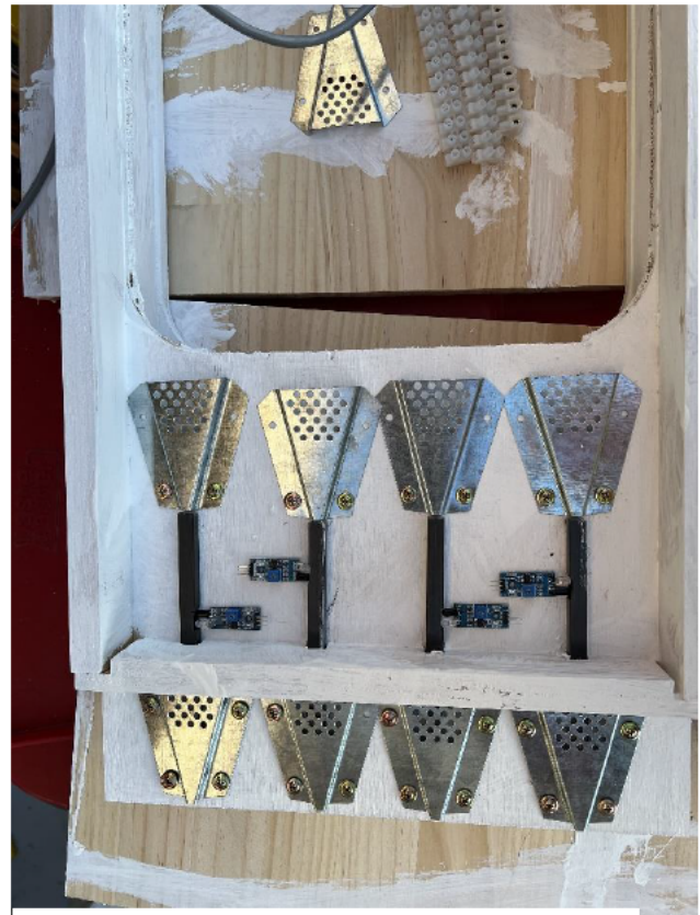
Figure 43: Construction of bee counters Showing IR sensor installed
