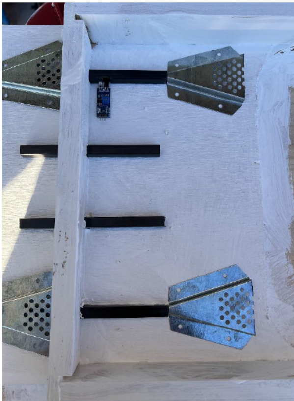
Figure 44: Construction of bee counters Showing the bee escapes and carbon tubes.
