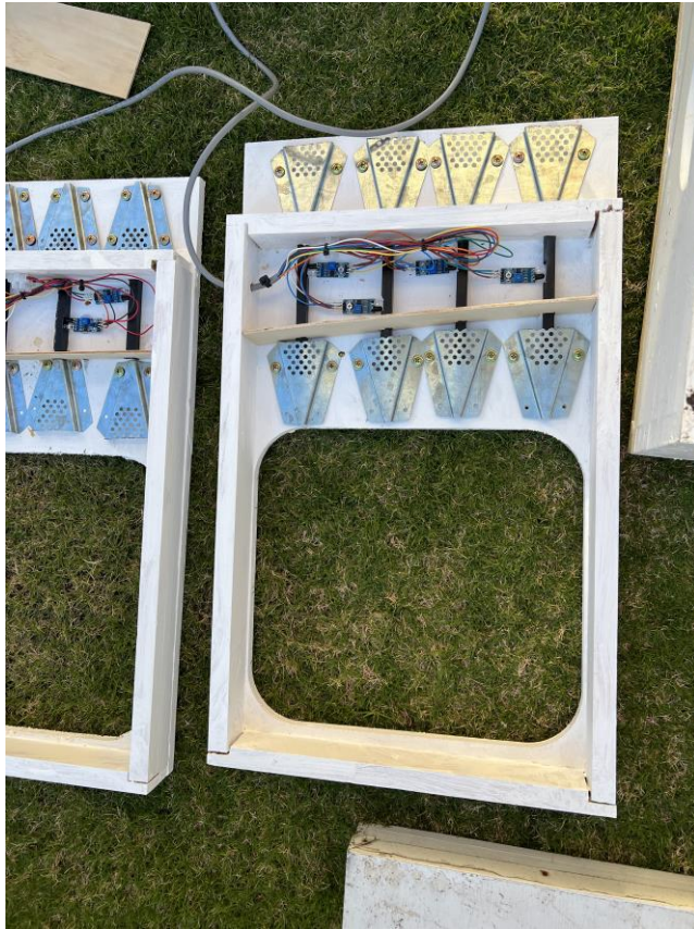
Figure 45: These bee escapes will count bees in the same way. This configuration however, which is different to Figure 36, will count the number of bees exiting the hive.
