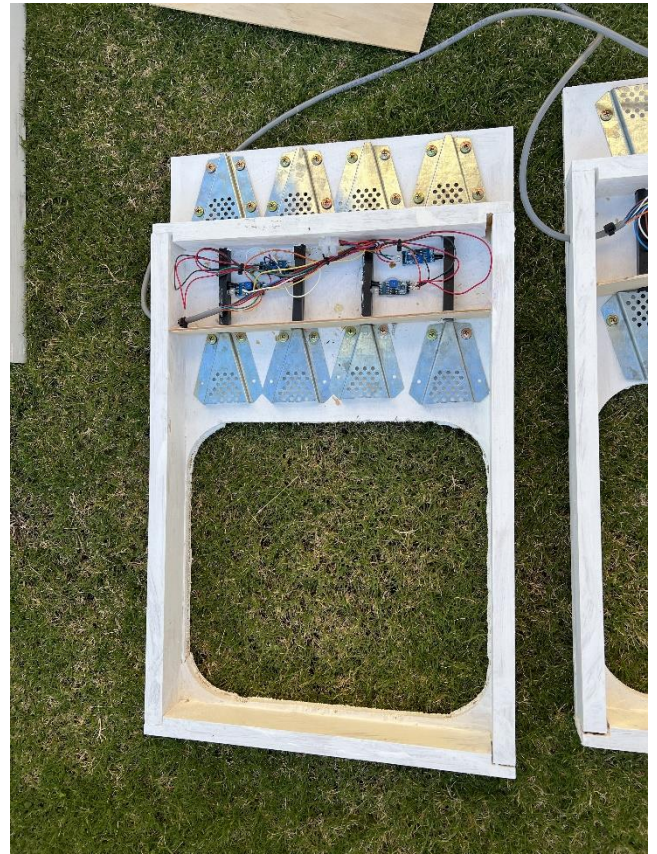
Figure 46: The placement of these bee escapes enables bees to enter the hive. When a bee lands on the top section of the board and starts to crawl through the bee escape towards the inside of the hive, the infrared sensor will send a signal to the micro controller.
