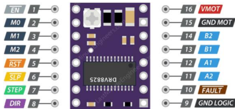
Figure 2.3: Drv8825 Pinout Diagram (Last Minute Engineers, 2018)
