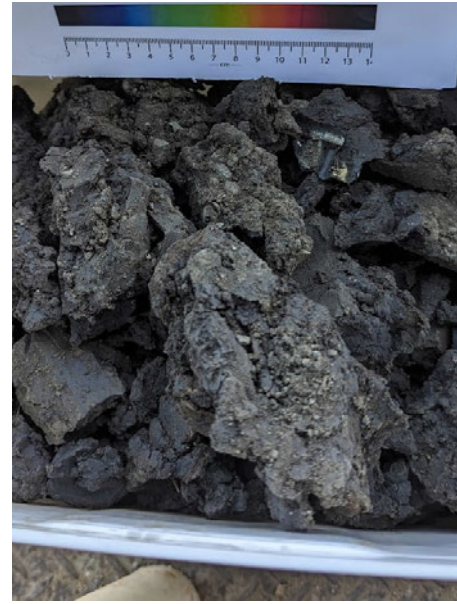
Figure 2.2: Sample of Black Soil displaying peds of varying sizes with slickensides. (R Kashanov 2023, personal photograph, 29 May)
