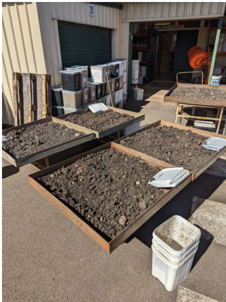
Figure 3.1: Example of a soil being air-dried in metal trays. (R Kashanov 2023, personal photograph, 1 May)
