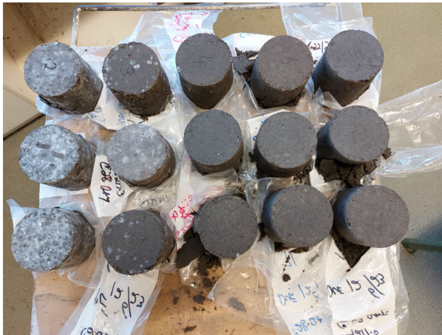
Figure 4.3: UCS cylinders following UCS testing, lined up with cylinders containing 2% lime on the left through to cylinders containing 8% lime on the right. (B Waters 2023, personal photograph, 2 June)
