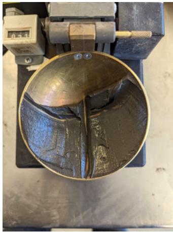
Figure 3.4: Wet soil being spread inside the Casagrande cup to determine the liquid limit as part of Atterberg limits test. (R Kashanov 2023, personal photograph, 1 May)
