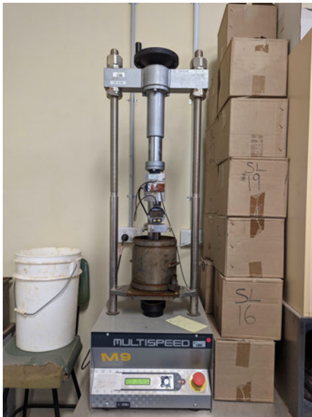
Figure 2.8: Example of a CBR test being performed. (R Kashanov 2023, personal photograph, 6 September)
