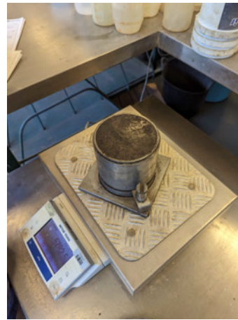
Figure 3.7: Soil compacted into a cylinder mould, being weight as part of MDR testing. (R Kashanov 2023, personal photograph, 1 May)
