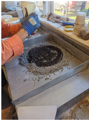
Figure 3.6: Water being added to a mixture of soil and hydrated lime. (R Kashanov 2023, personal photograph, 1 May)
