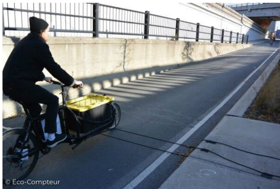
Figure 3 - Pressure Tubes for counting bicycles (Eco-Counter, 2022)
