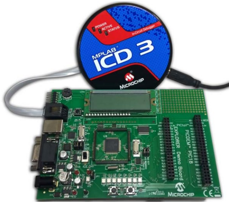
Figure 13 - PIC18 development board with debugger (Microchip, 2023)
