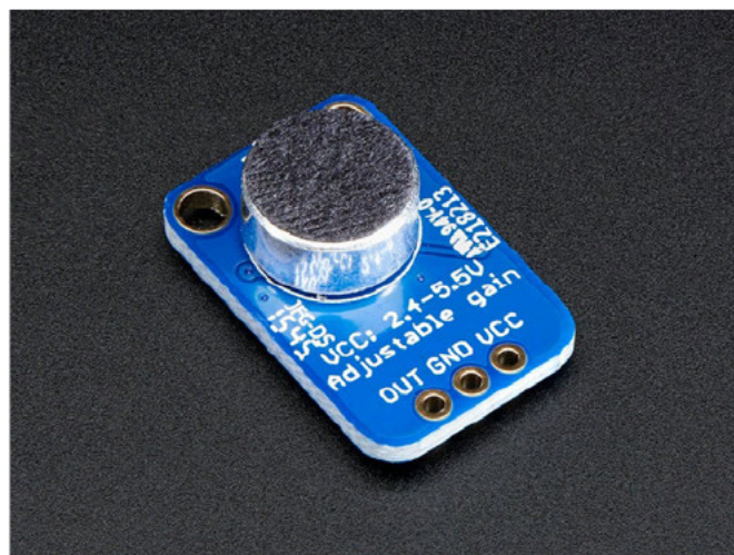
Figure 15 - Electret Microphone with Pre-Amplifier(Adafruit 2023b)
