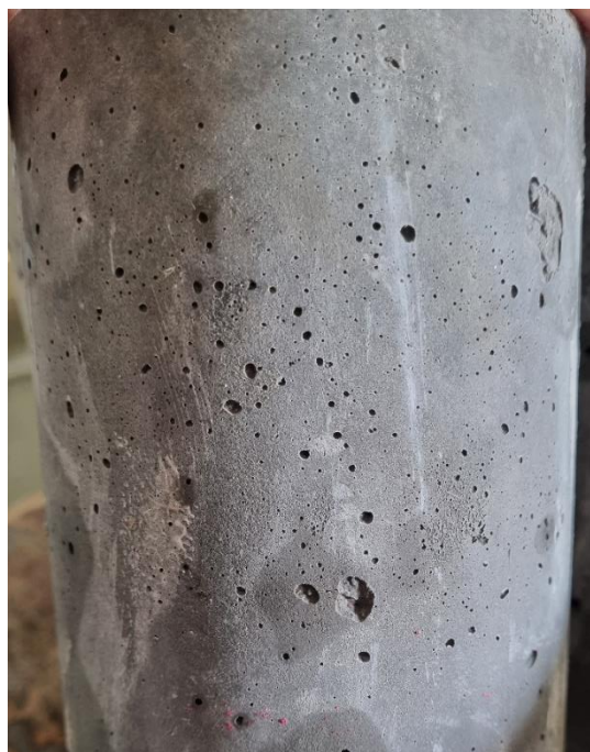
Figure 5.3 – Surface Finish of Typical Cylinder with 30% Pond ash, After 7 Day Testing
