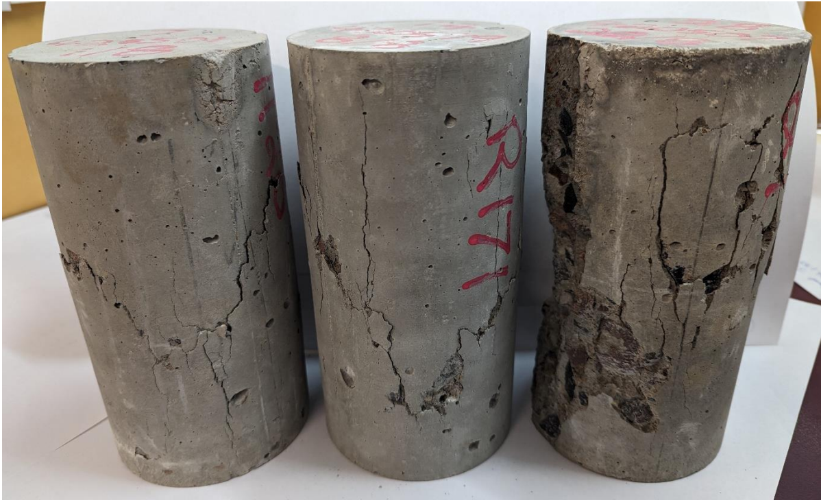
Figure 5.6 – Control Sample Fracture Patterns, Left - 7 Days, Middle - 14 Days, Right - 28 Days
