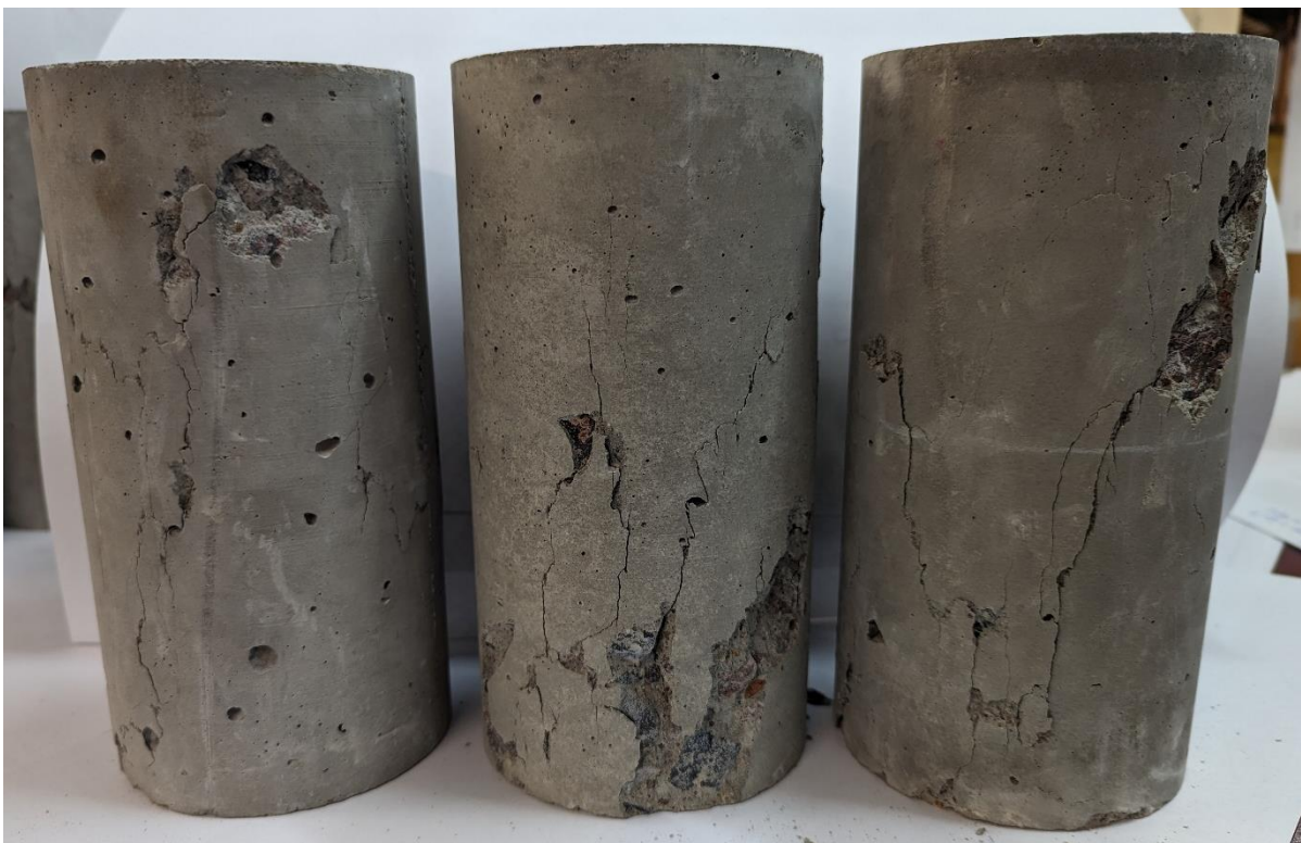
Figure 5.7 – 10% Sample Fracture Patterns, Left - 7 Days, Middle - 14 Days, Right - 28 Days
