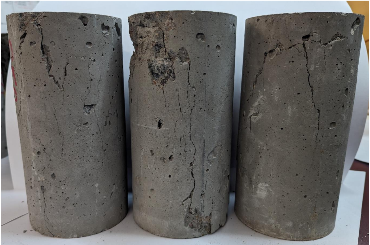
Figure 5.8 – 20% Sample Fracture Patterns, Left - 7 Days, Middle - 14 Days, Right - 28 Days
