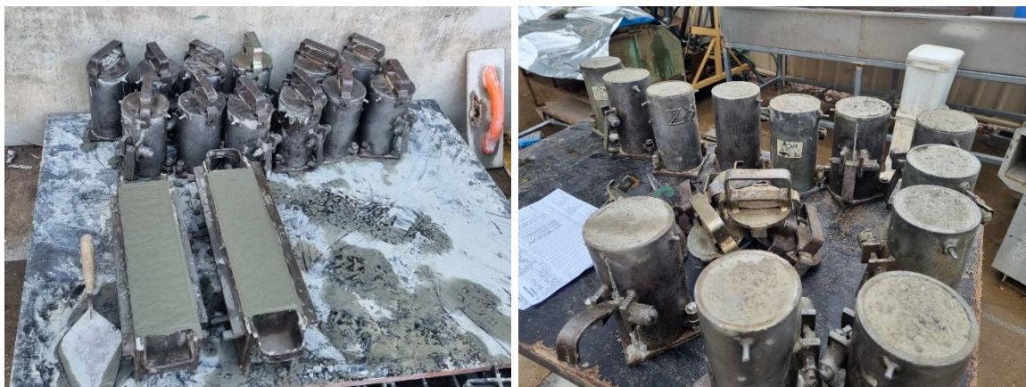
Figure 4.11 – Prepared Samples, Green (Left) and after Approximately 24 Hours (Right)
