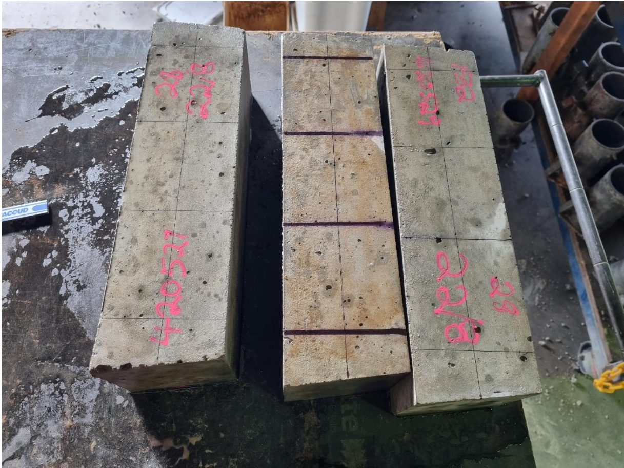
Figure 4.16 – Flexural Samples with Third Points Marked for Testing
