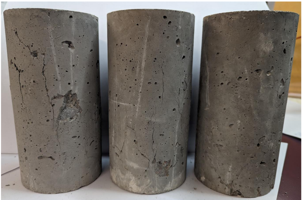
Figure 5.9 – 30% Sample Fracture Patterns, Left - 7 Days, Middle - 14 Days, Right - 28 Days
