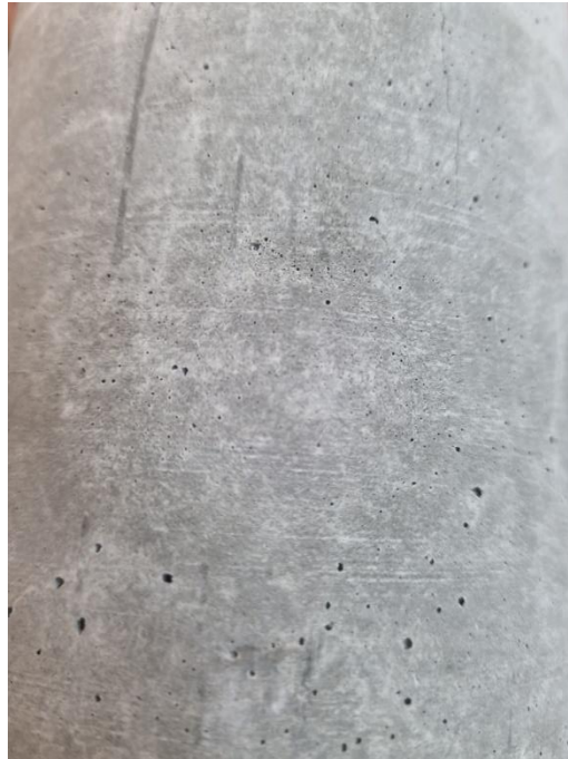
Figure 5.2 – Surface Finish of Typical Control Cylinder, After 7 Day Testing
