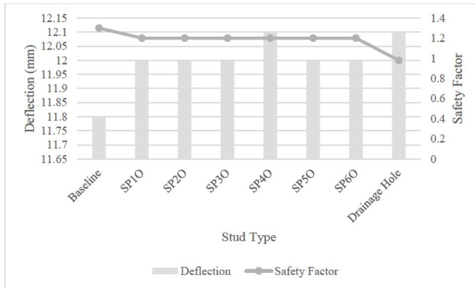
Figure 29 – Deflection and Safety Factor of Web Perforation Variants.
