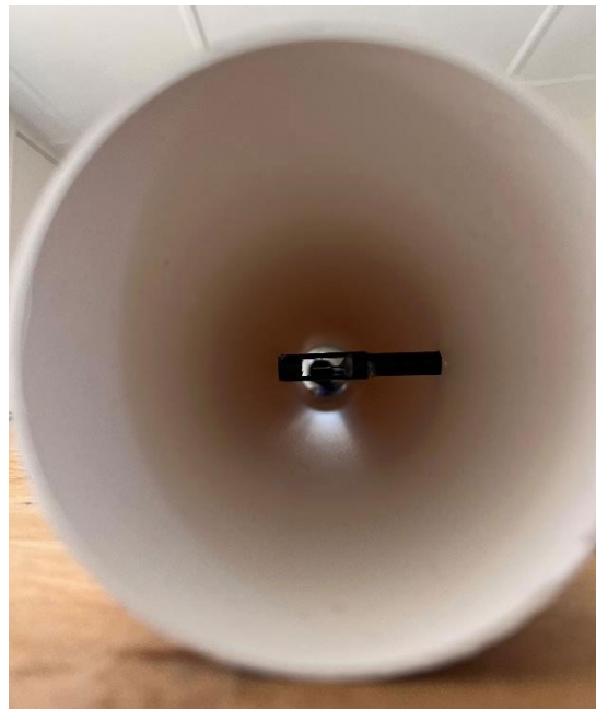
Figure 15 Wind tunnel testing apparatus for CTA sensor calibration
