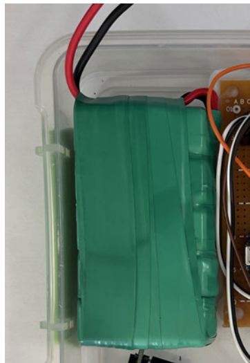
Figure 10 Battery bank - 5 x 9V (Energizer MAX)
