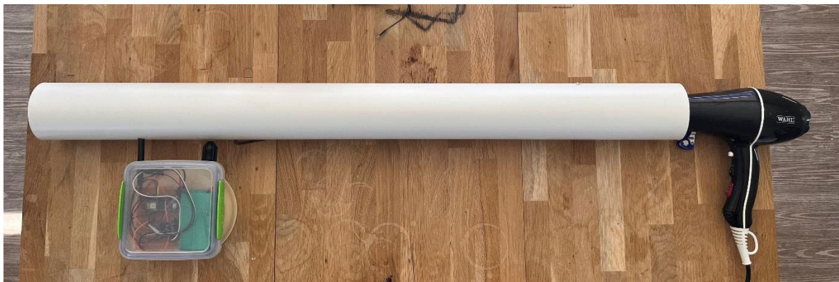
Figure 13 Setup for calibrating the CTA sensor.
