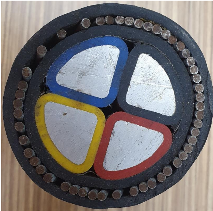
Figure 19 Low Voltage PVC Cable Cross Section
