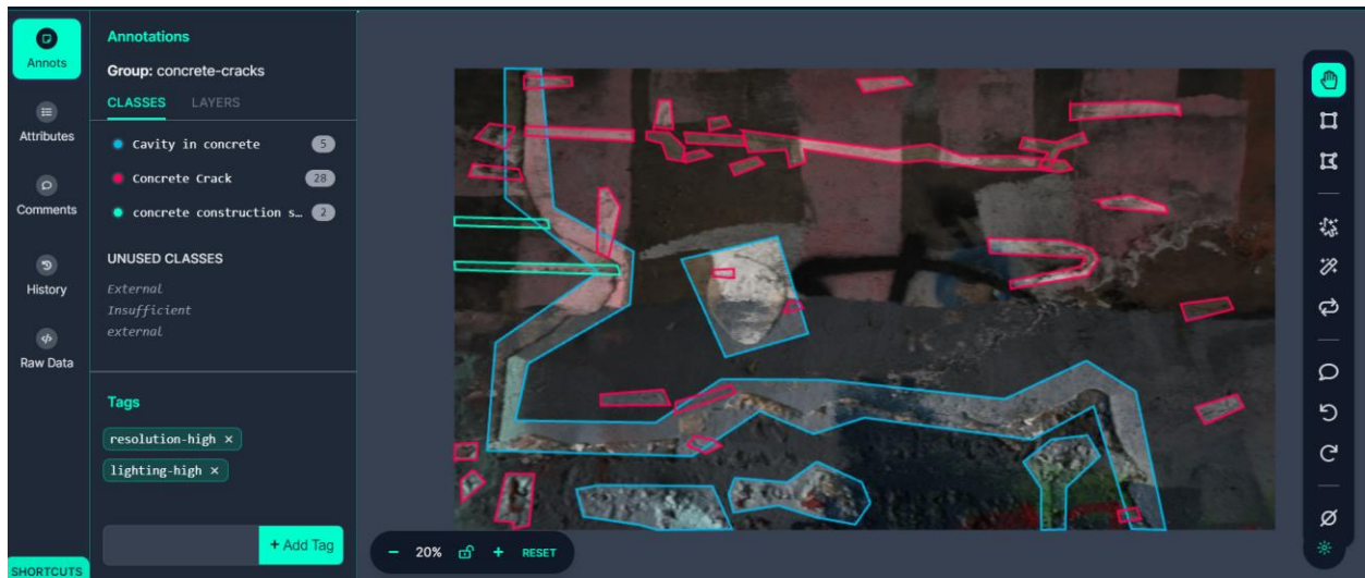
Figure 15. Example of annotated image in Roboflow
