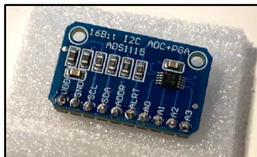
Figure 25 – the 16-bit ADS1115 Analogue-to-Digital converter
