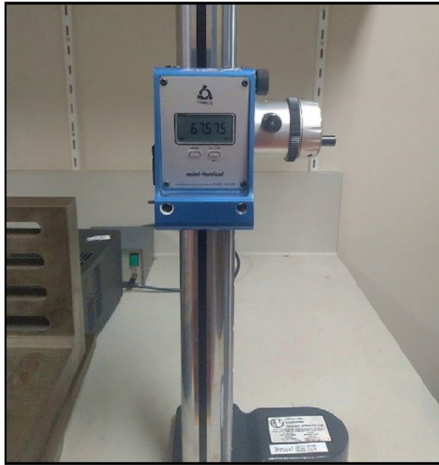
Figure 11 – Image of Trimos height gauge. Used in the calibration of linear position transducers to perform vertical displacement.
