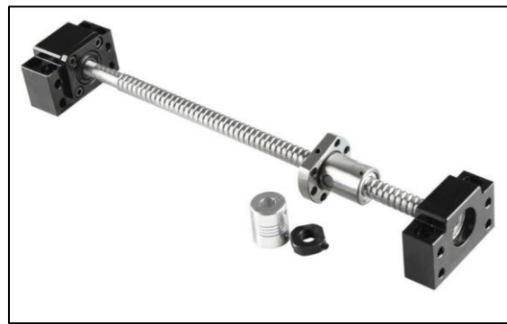
Figure 19 – SFU1204 550 mm ball screw, BK/BF10 bearing blocks, spindle and coupling.
