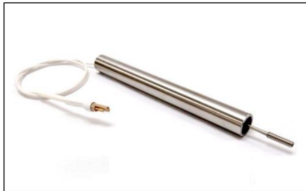
Figure 2 – an LVDT consisting of primary and secondary windings and a linearly displaceable magnetic core rod (Lord Sensing 2022).
