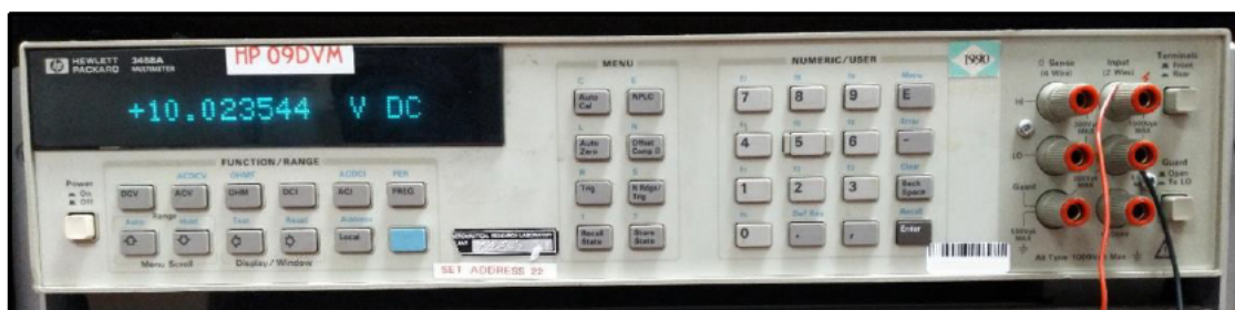
Figure 10 – Image of the HP 3458A Multimeter that is used for voltage measurement in the current FFL LVDT calibration system.
