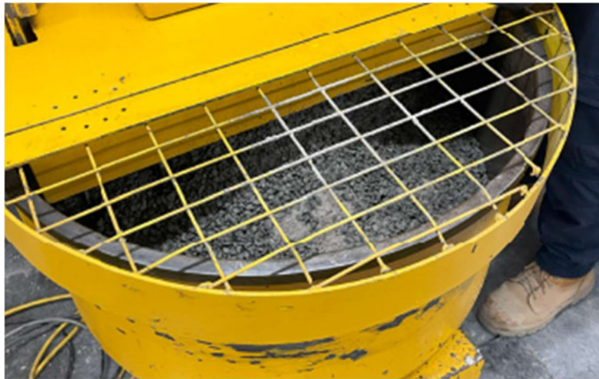
Figure 4.20 Mixer showing viewing opening with dry constituents mixed.
