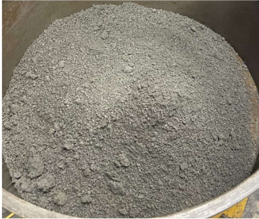
Figure 4.4 Coarse Sand used, Manufactured sand of the same source as the coarse aggregate.
