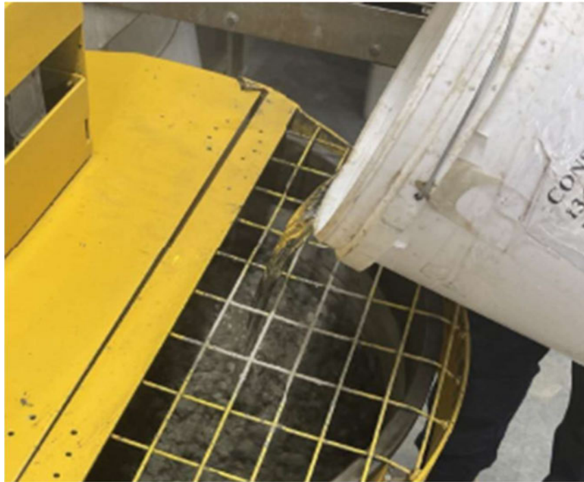
Figure 4.6 Water and admixture being added to mixer.
