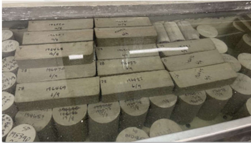
Figure 4.26 Specimens from day 1 after being stripped and placed in curing until crushing / loading to be carried out at correct age in days.
