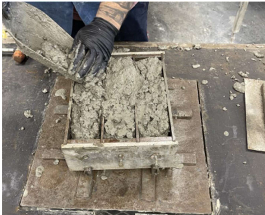
Figure 4.39 Shrinkage mould topping up second layer.
