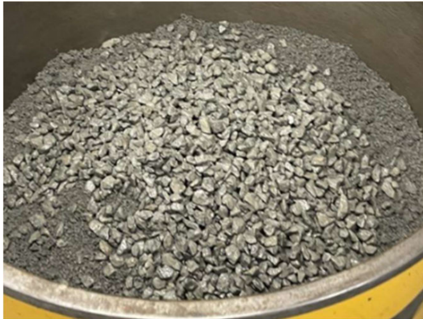
Figure 4.2 Coarse aggregate used, 20mm maximum.
