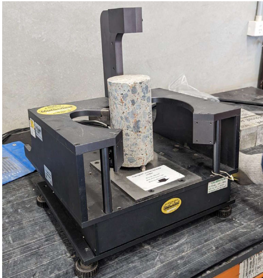
Figure 4.31 Cylinder being weighed and dimensioned.
