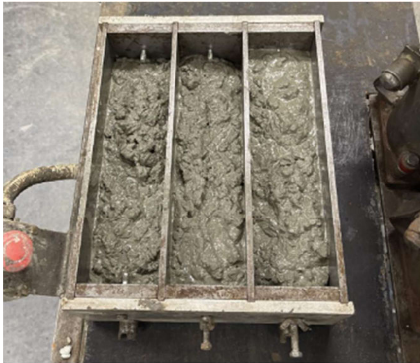
Figure 4.38 Shrinkage mould half filled.
