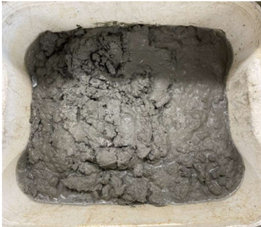
Figure 4.24 Concrete with higher amount of bleed, pooling in corners and indentations.
