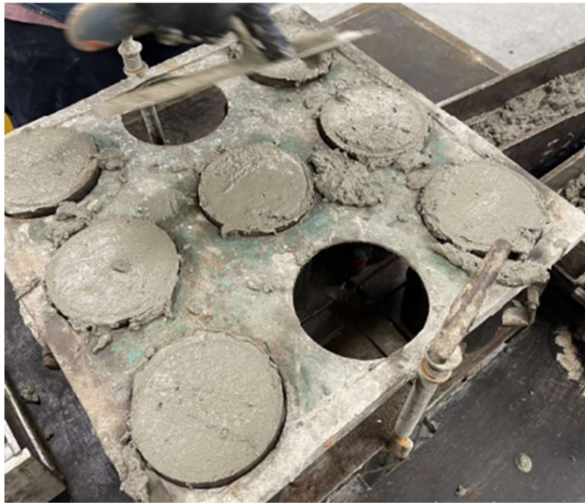
Figure 4.29 Cylinders trowelled off.
