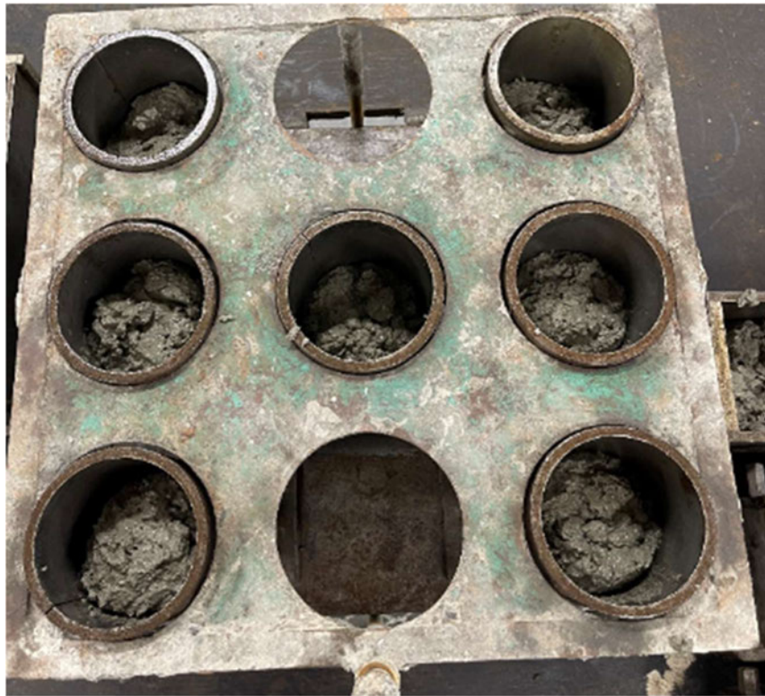
Figure 4.27 Cylinders in hold down jig filled in first layer before vibration.
