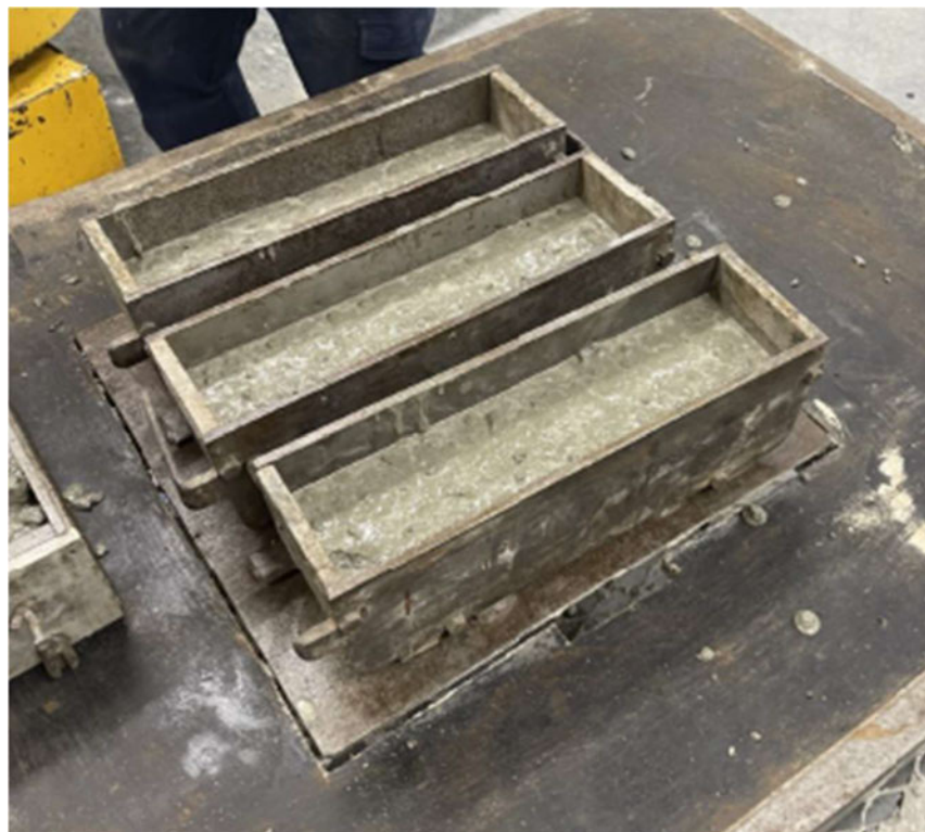
Figure 4.35 Vibrated after half filling.
