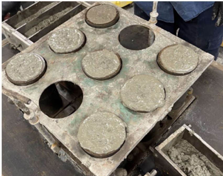
Figure 4.28 Cylinders full and completely vibrated.
