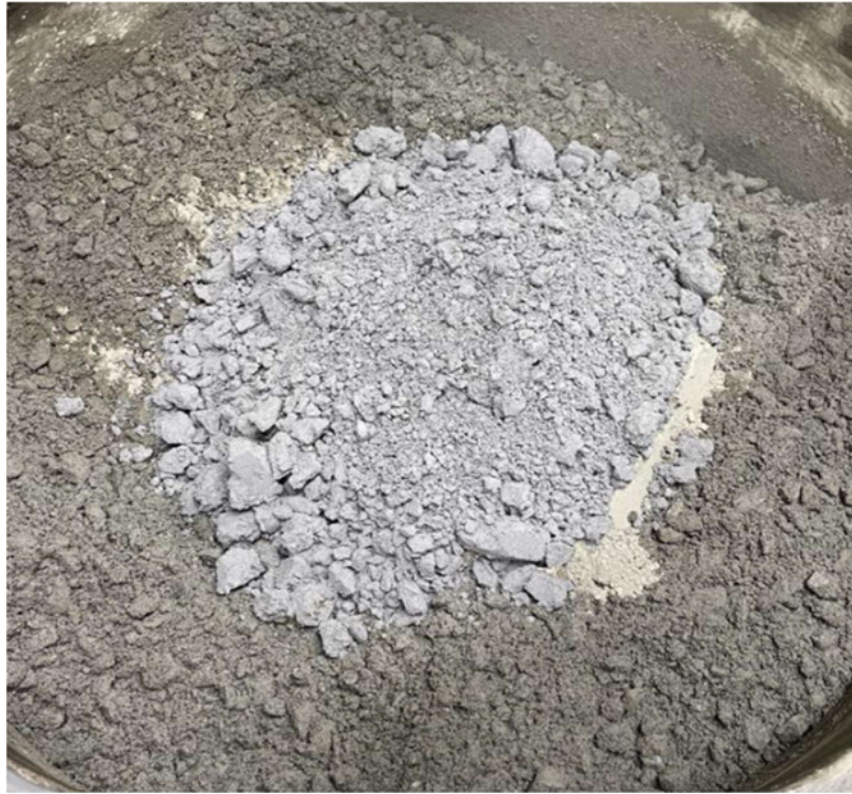
Figure 4.9 Harvested Ash in the mixer.
