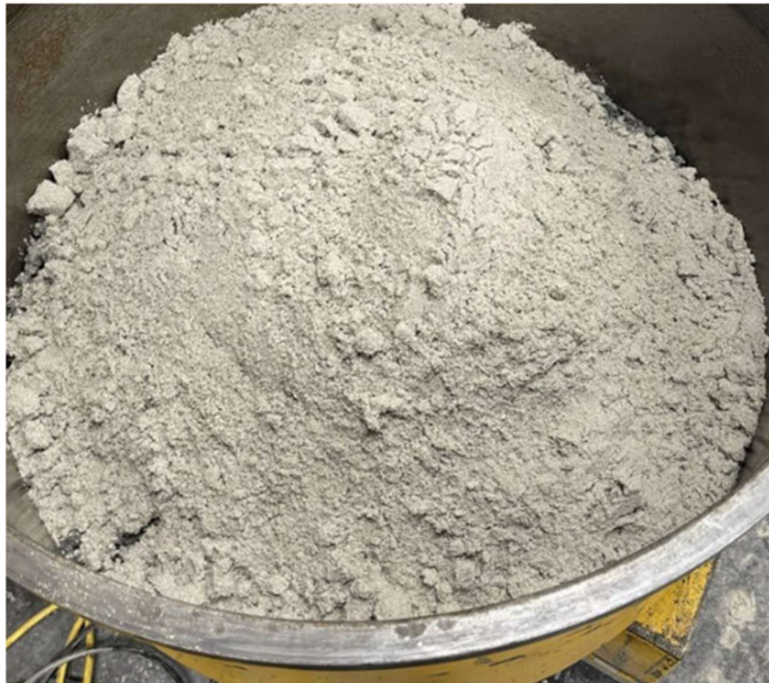
Figure 4.5 Fine sand used; natural sand sourced from Moreton Bay.
