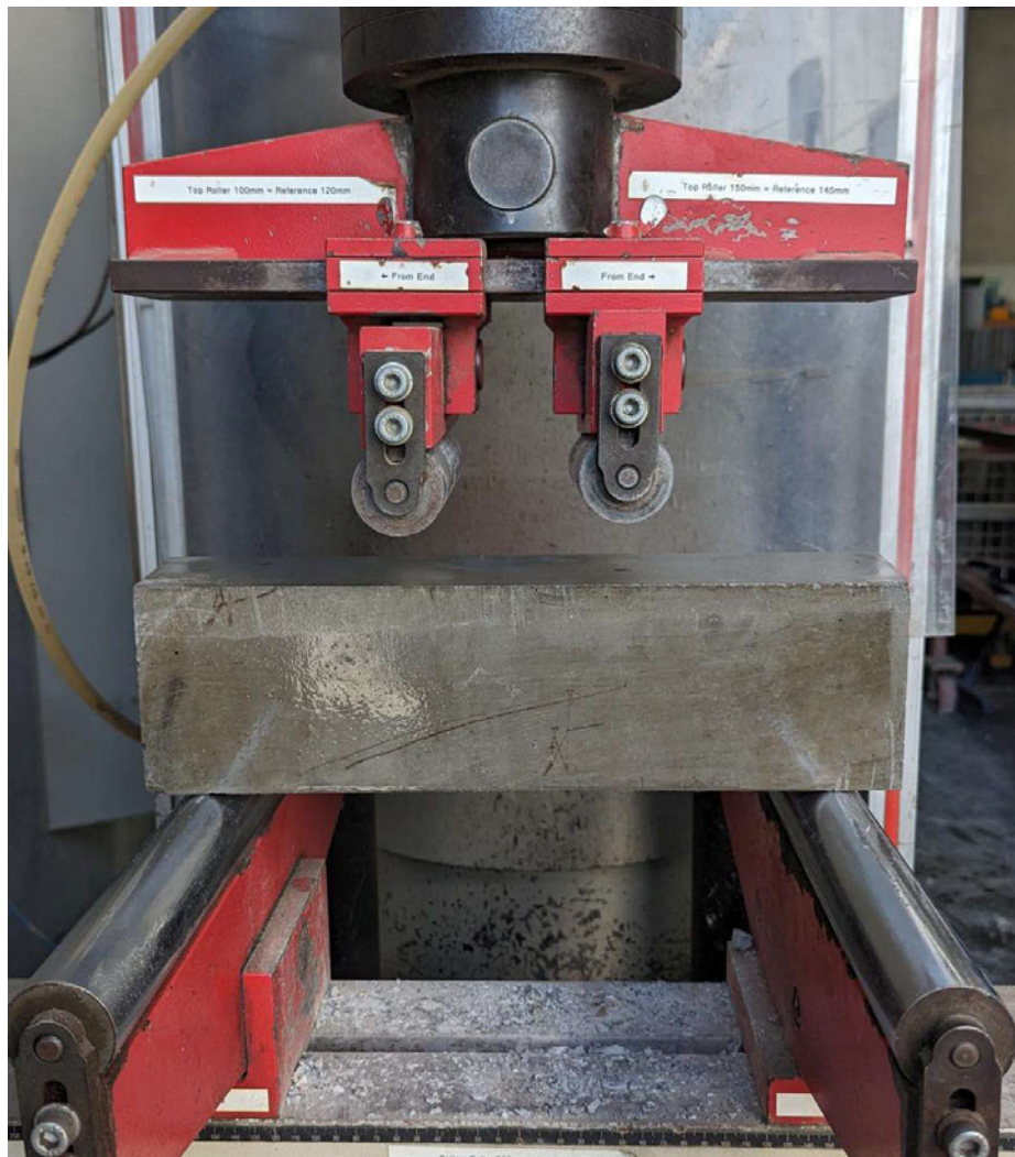
Figure 4.37 Flex beam in jig to be crushed in four points bending to determine flexural tensile strength.
