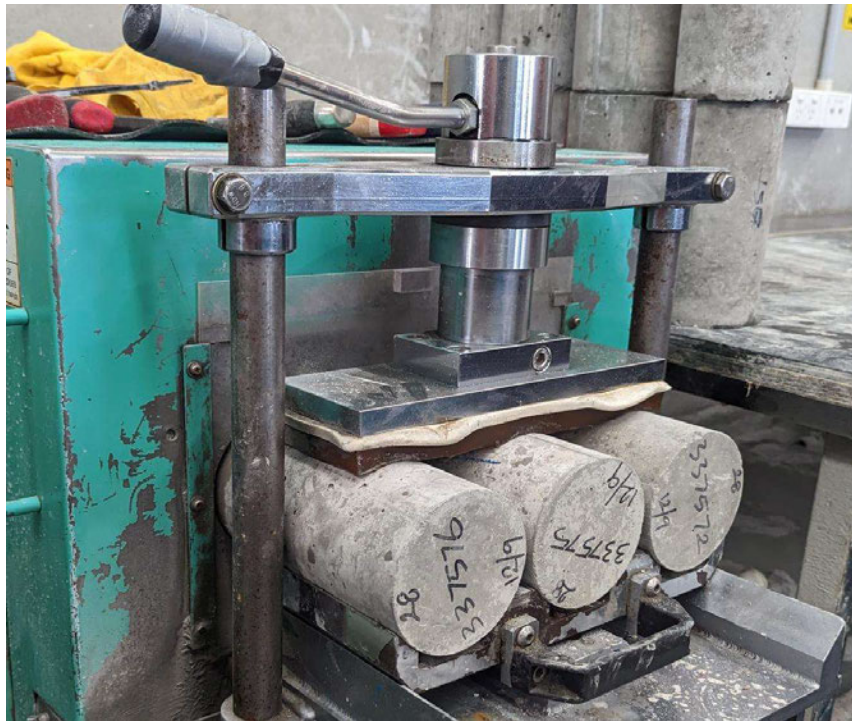
Figure 4.30 Cylinders having their trowelled end ground to be flat.
