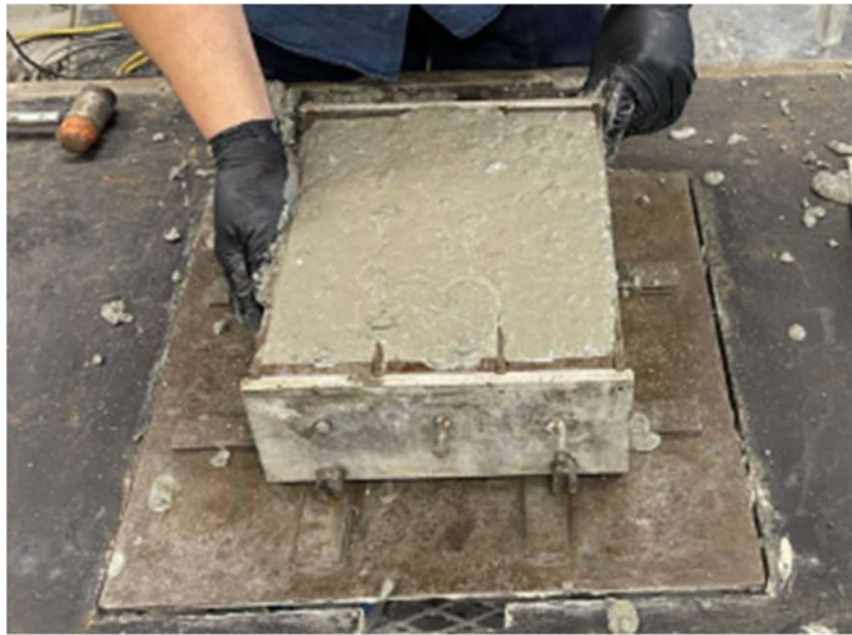
Figure 4.40 Shrinkage vibrated after filling.
