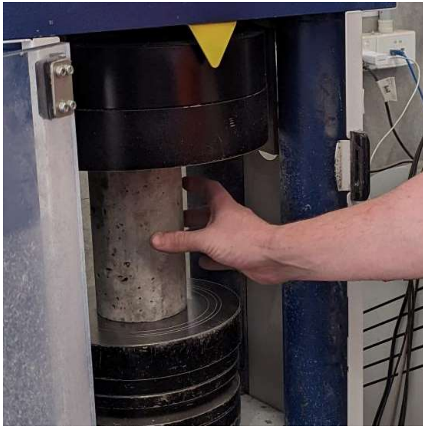
Figure 4.32 Cylinder being crushed.
