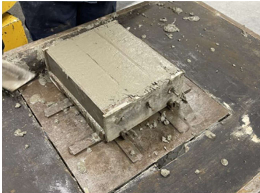
Figure 4.41 Shrinkage sample trowelled off.
