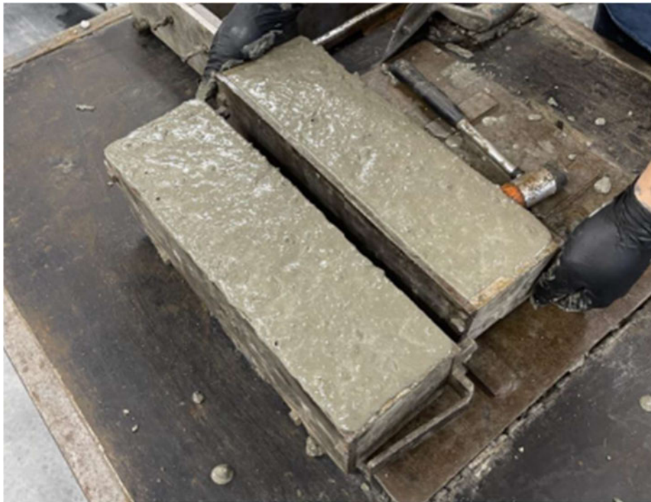
Figure 4.36 Filled and vibrated before being trowelled off.
