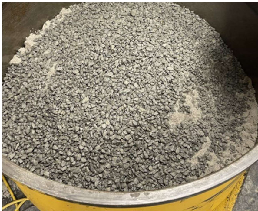
Figure 4.3 Coarse aggregate used, 10mm maximum.
