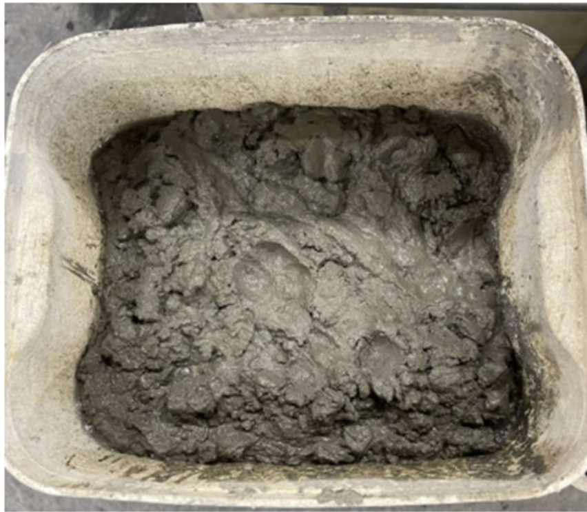
Figure 4.22 Concrete with minimal to no visible bleed
