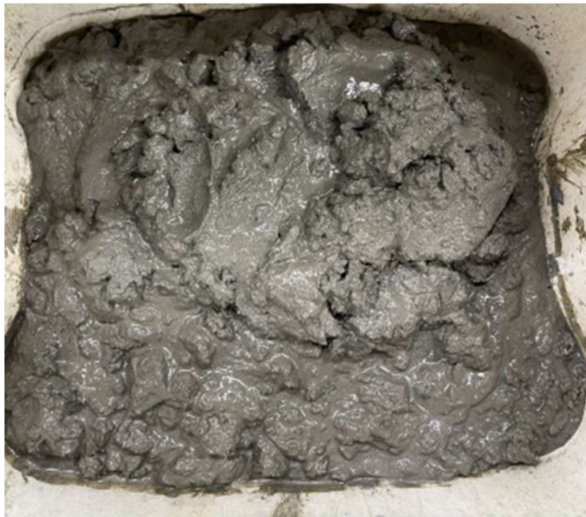
Figure 4.23 Concrete with some visible bleed, sheen across the top surface
