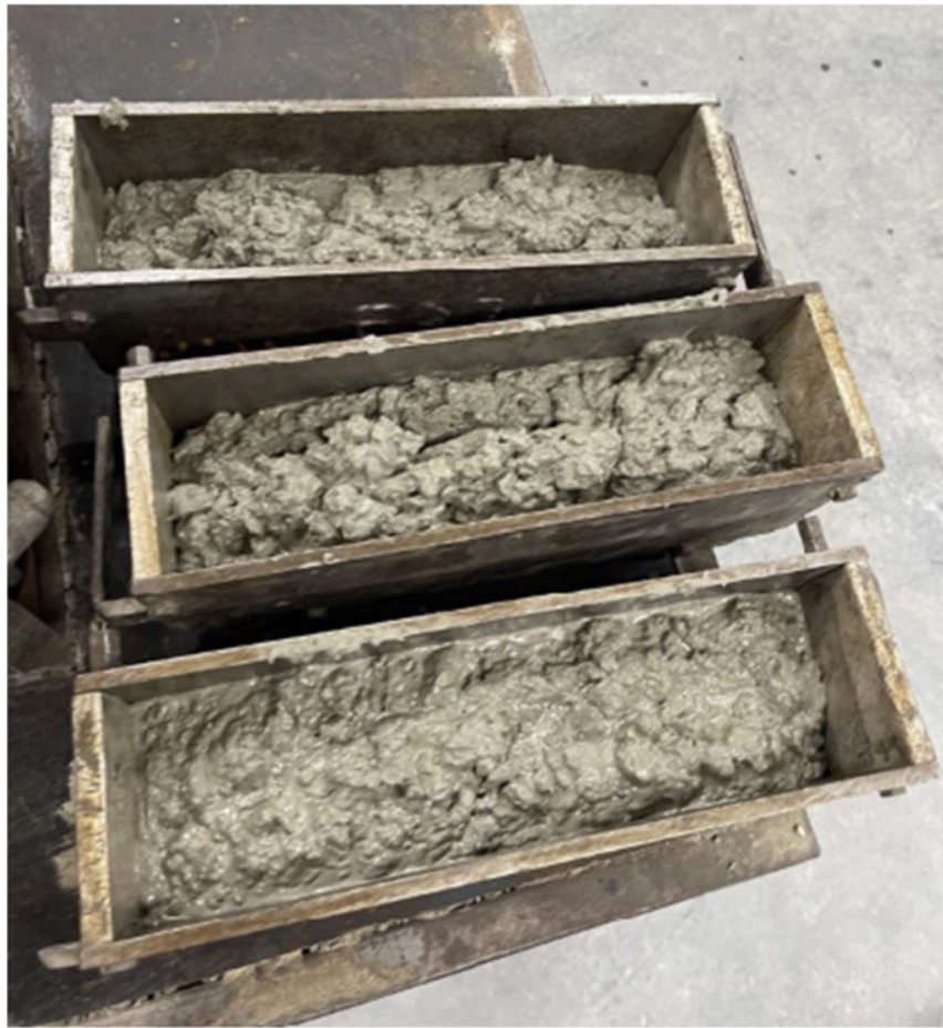
Figure 4.34 Half-filled flex beams.
