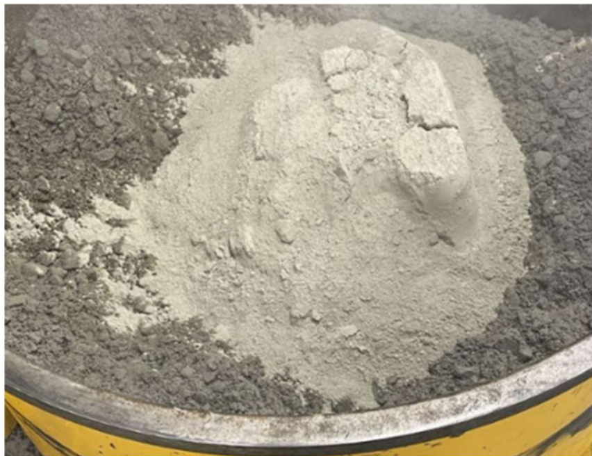
Figure 4.1 Cement used, Sunstate General Purpose Cement
