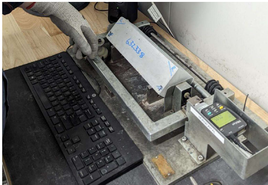
Figure 4.42 Shrinkage prism being measured.
