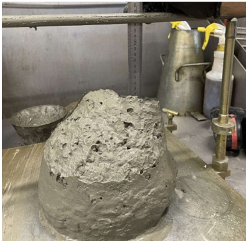
Figure 4.19 Example of slump being measured.
