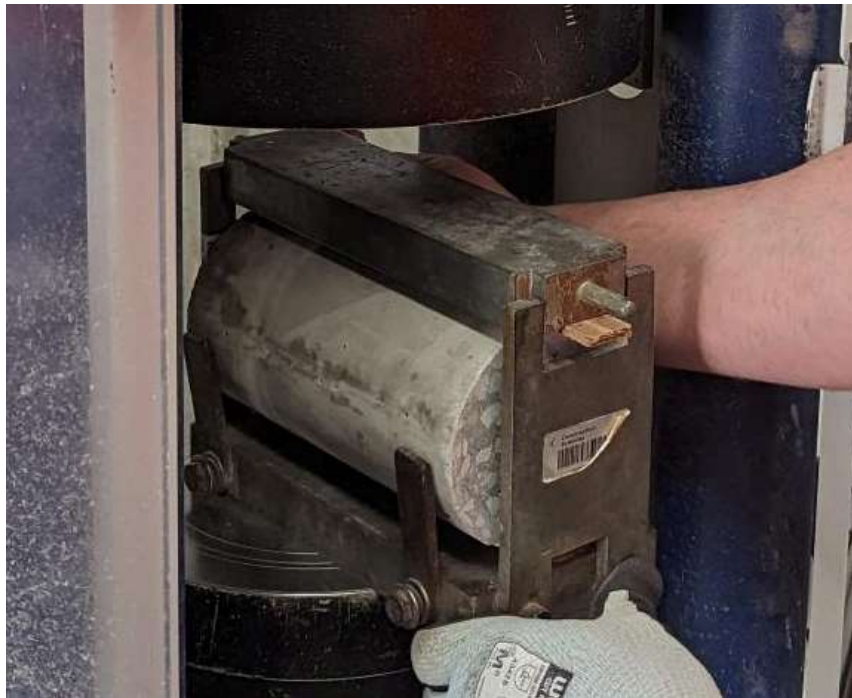
Figure 4.33 Cylinder in jig being crushed to determine the 'splitting tensile' or indirect tensile strength.
