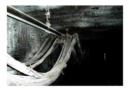
Figure 2.5: A longwall monorail system supported by underground roof bolts (Macquarie Manufacturing 2023).
