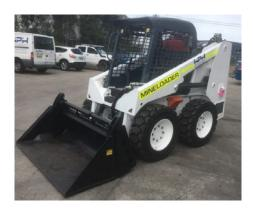
Figure 2.3: Typical skid steer loader used in an underground coal mine (shown with hydraulic bucket attachment) (Hunter Plant Hire 2023).
