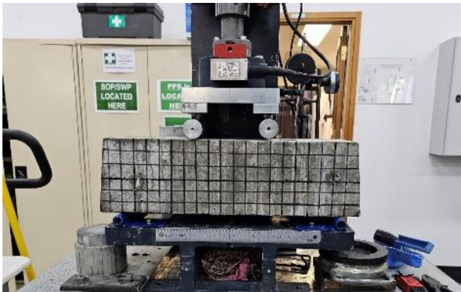
Figure 29: Concrete Beam with Grid on 4-Point Test Rig
