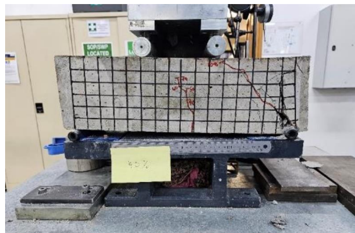
Figure 36: 40% RCG sample 1 at failure
