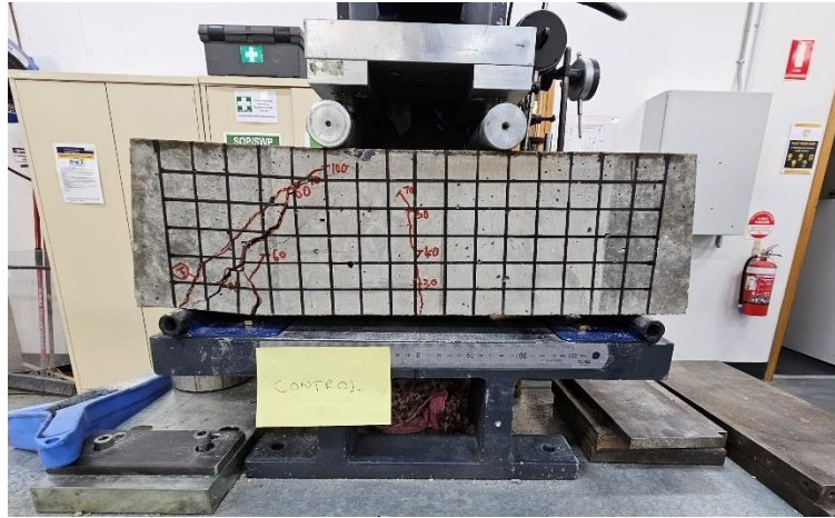
Figure 32: Control sample 1 at failure
