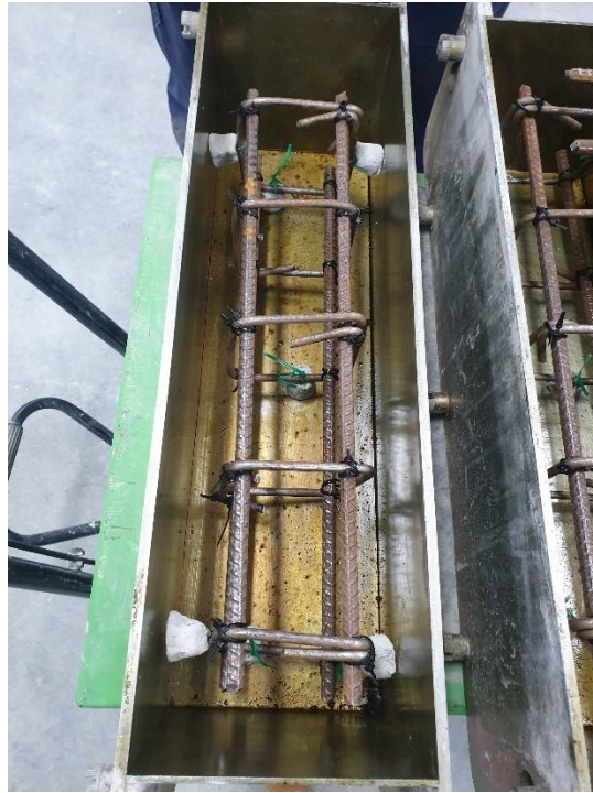
Figure 14: Concrete Beam Reinforcement in Mould
