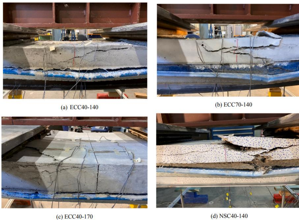
Figure 2.1 Comparison of Failure Modes. Source: (Nguyen & Lee 2021)
