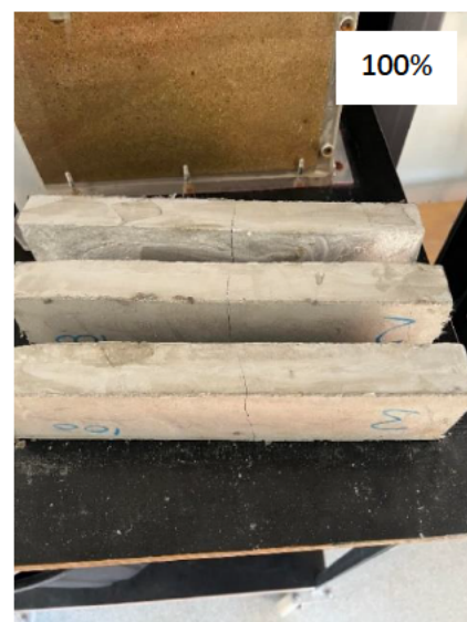
Figure 5.9 Failure of All Beams Undergoing Flexural Testing
