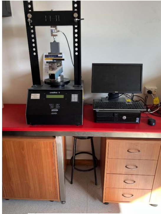
Figure 4.13 Flexural Test Set Up
