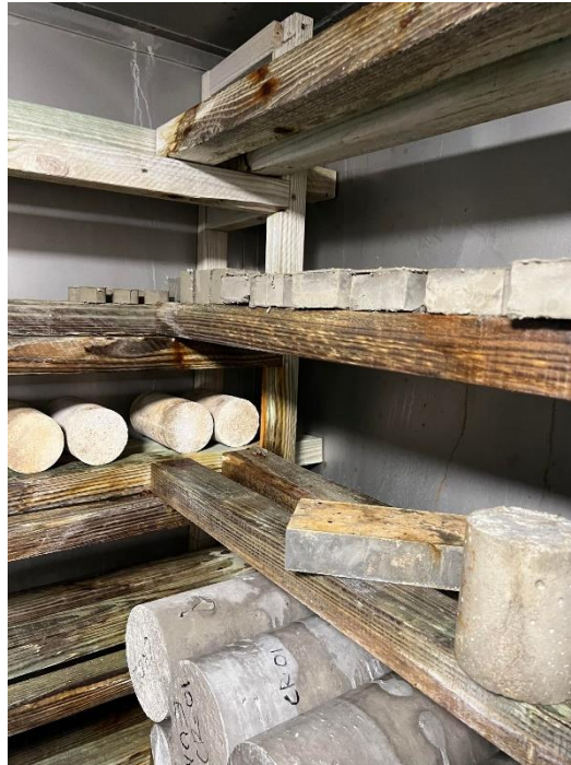
Figure 4.11 Samples Stored in Curing Room
