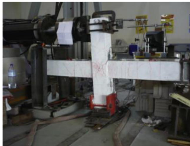
Figure 2.2 Test Set Up with Hydraulic Actuator. Source: (Qudah & Maalej 2014)
