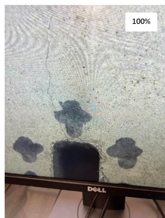
Figure 5.20 Crack Initiation from Top of Notch for Samples
