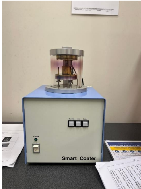
Figure 4.22 Machine Used to Apply Gold Sputter Coating
