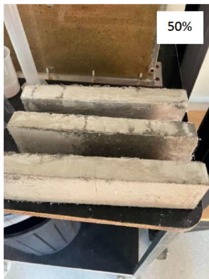
Figure 5.9 Failure of All Beams Undergoing Flexural Testing
