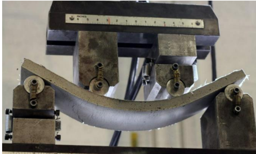
Figure 1.2 ECC Under an Applied Load. Source: (Yuva Engineers 2011)
