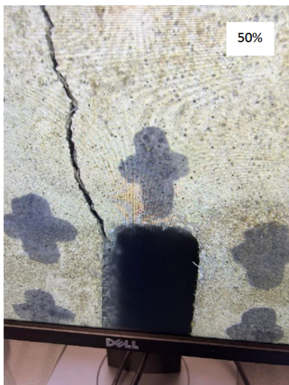
Figure 5.20 Crack Initiation from Top of Notch for Samples
