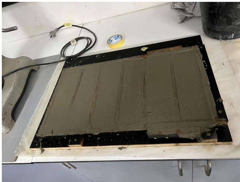
Figure 4.10 Mixture Added to the Custom Moulds
