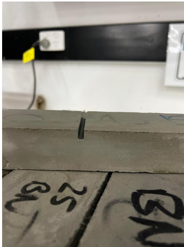
Figure 4.16 10mm Notch in Beams
