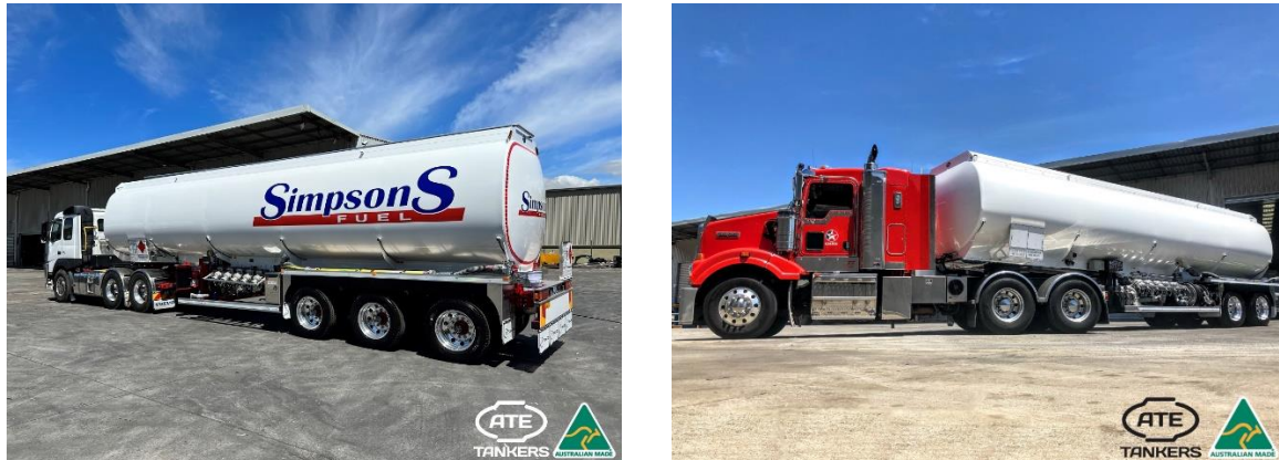
Figure 3.4-46: Tri-axle, 5-compartment semitrailer tanker (ATE_Tankers 2023)
