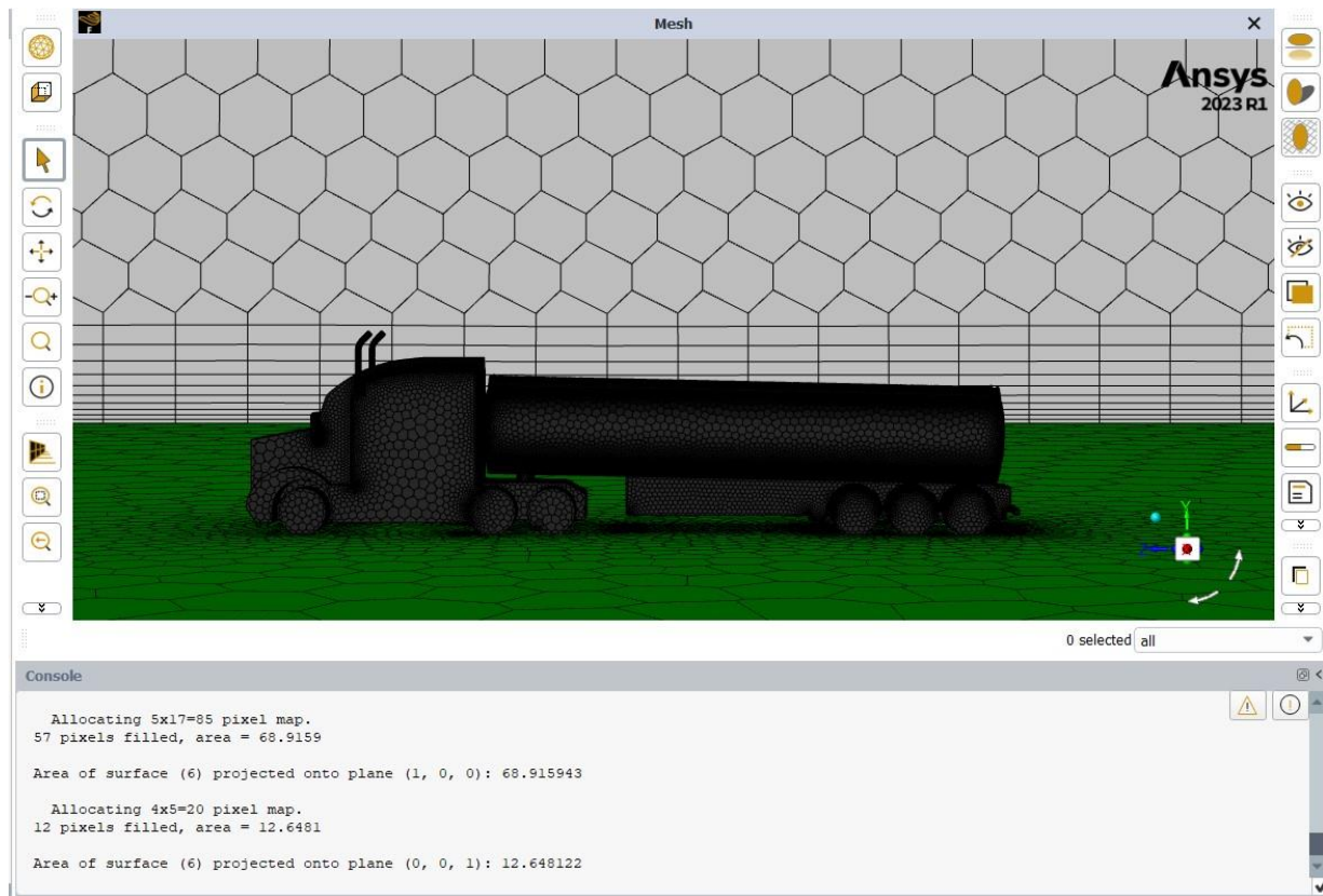
Figure 4.1-64: Aerodynamic Model Final Volume Mesh.
