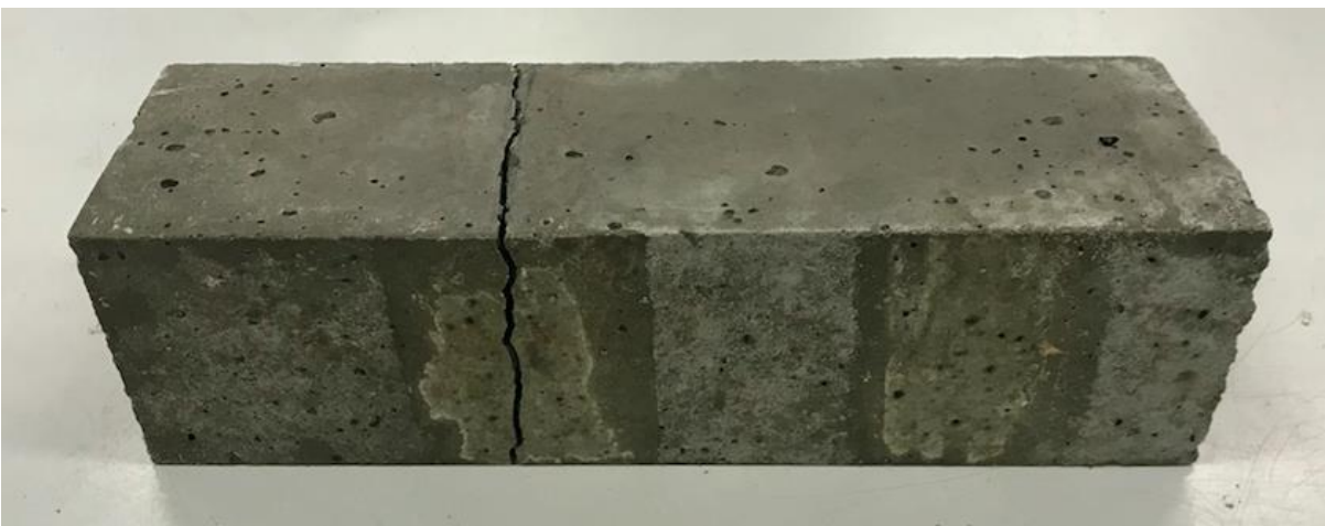
Figure 5-18. Fractured flexural strength specimen from the 50% HA mix.
