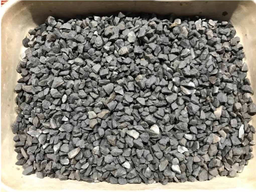
Figure 4-1. 10 mm basalt aggregate used for this research project.
