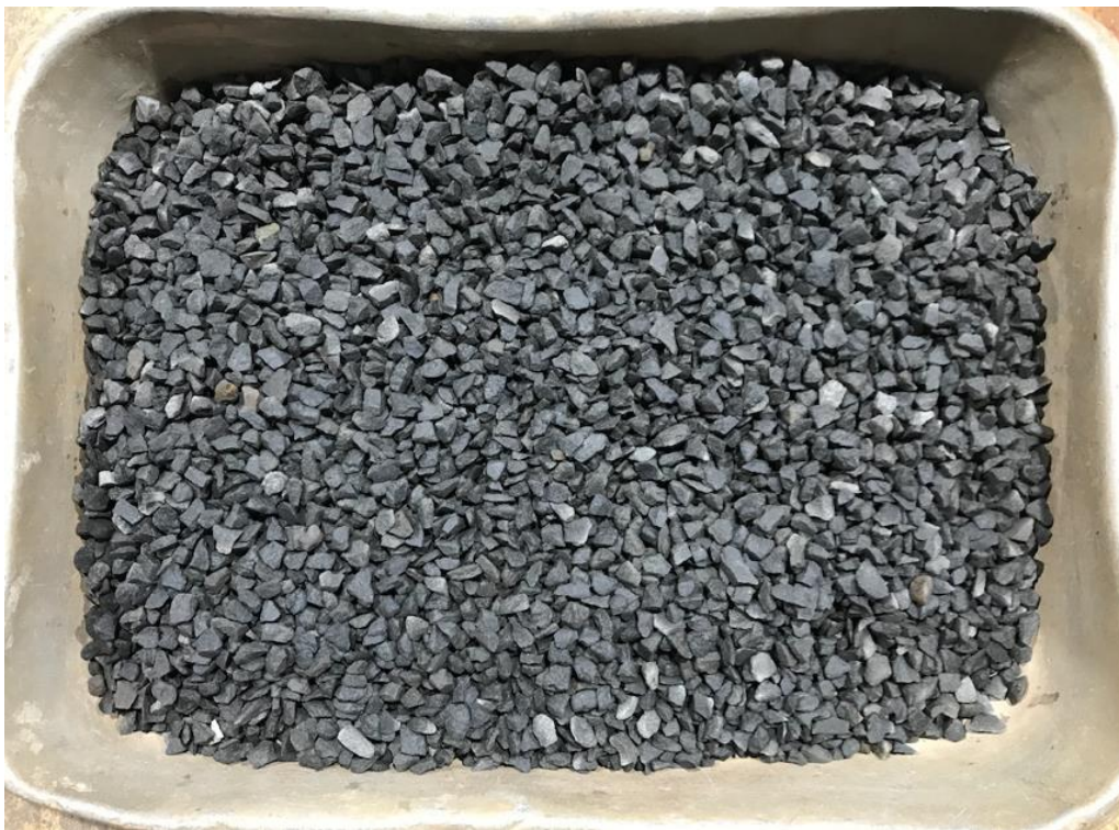
Figure 4-2. 7 mm basalt aggregate used in this research project.
