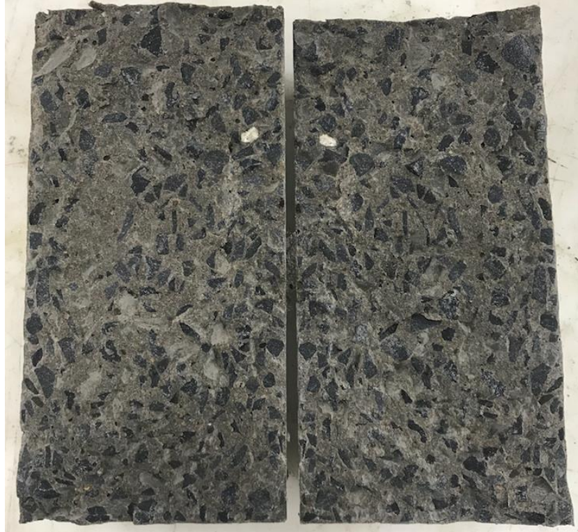
Figure 5-12. Control mix tensile strength specimen after testing.
