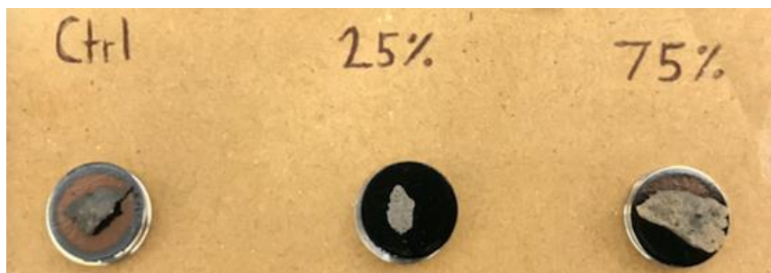
Figure 3-5. Mounted and gold sputter coated specimens ready for SEM analysis.
