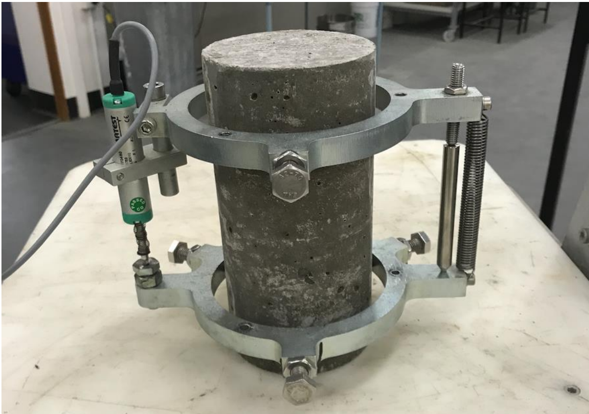
Figure 5-21. 12.5% HA test specimen with displacement measuring device attached.
