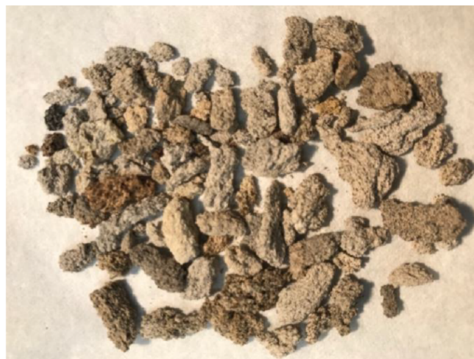
Figure 5-4. Photo of washed HA particles showing rough and angular surface texture.
