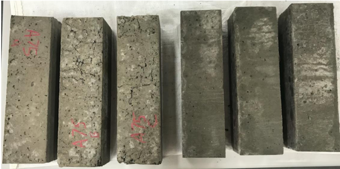
Figure 4-19. Flexural strength beam specimens from the 75% (left) and 12.5% (right) HA concrete mixes.
