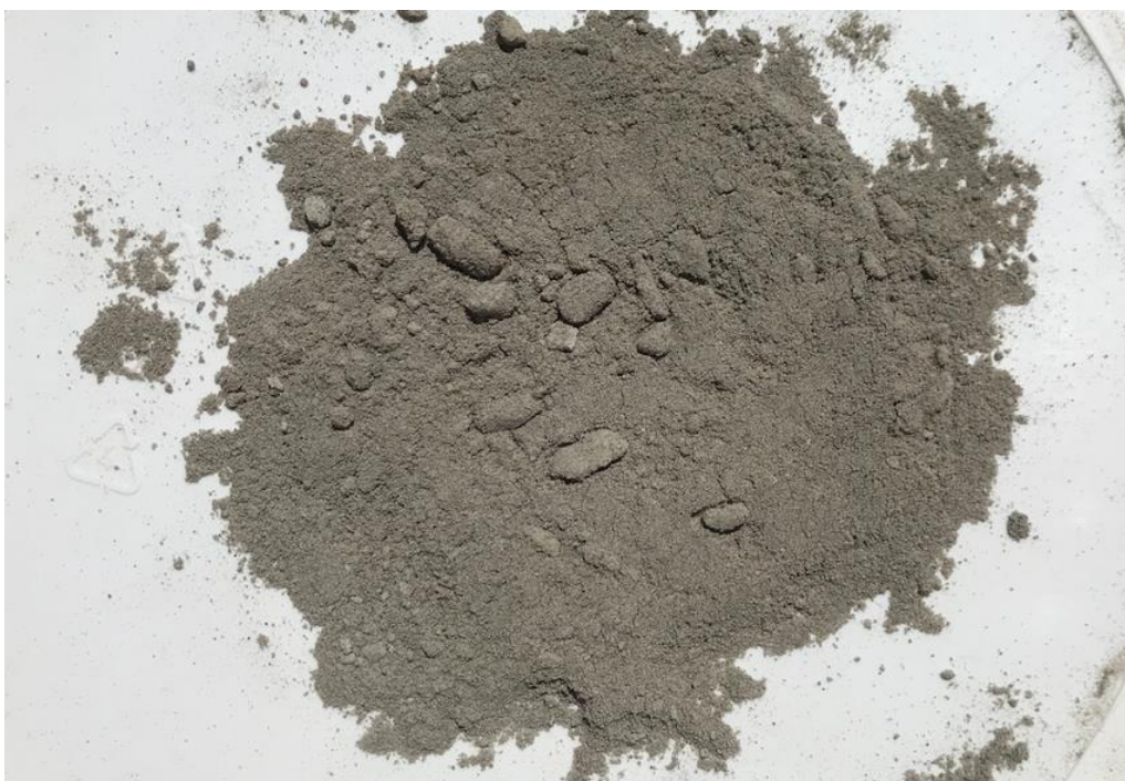
Figure 4-4. Harvested ash from Millmerran power station used in this research project.
