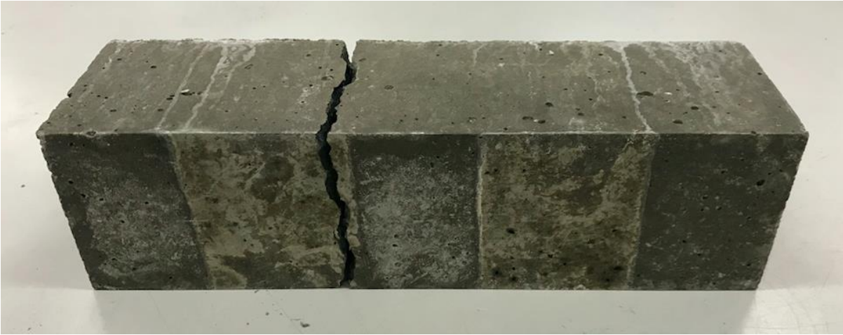
Figure 5-17. Fractured flexural strength specimen from the 25% HA mix.
