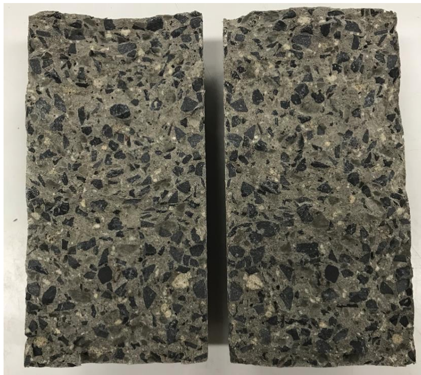
Figure 5-13. 75% HA replacement mix tensile strength specimen after testing.
