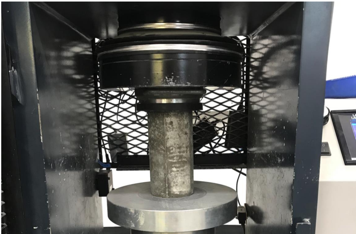
Figure 5-7. Compression test specimen from control batch in compression machine ready for testing.
