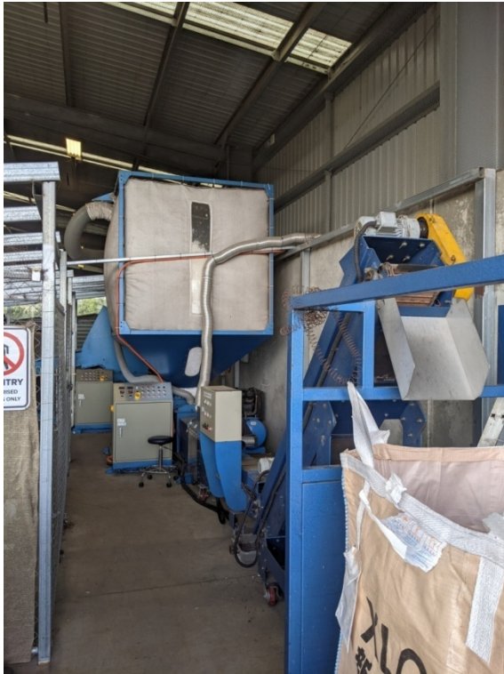
Figure 29 – Polystyrene compactor control unit, hopper and collection bin
