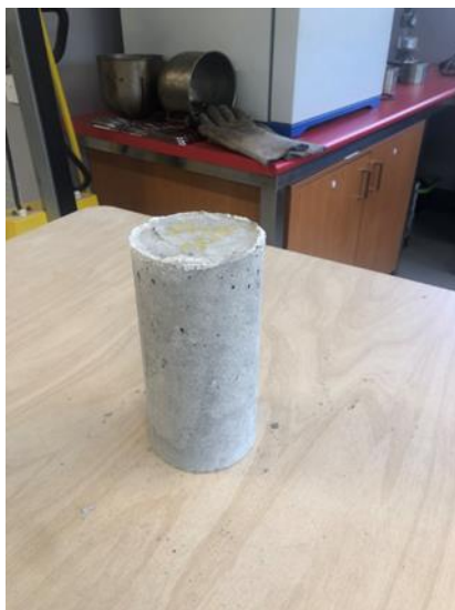
Figure 10: Photo of 15% LSS and 70/30 Fly Ash to Sand geopolymer specimen from current investigation.
