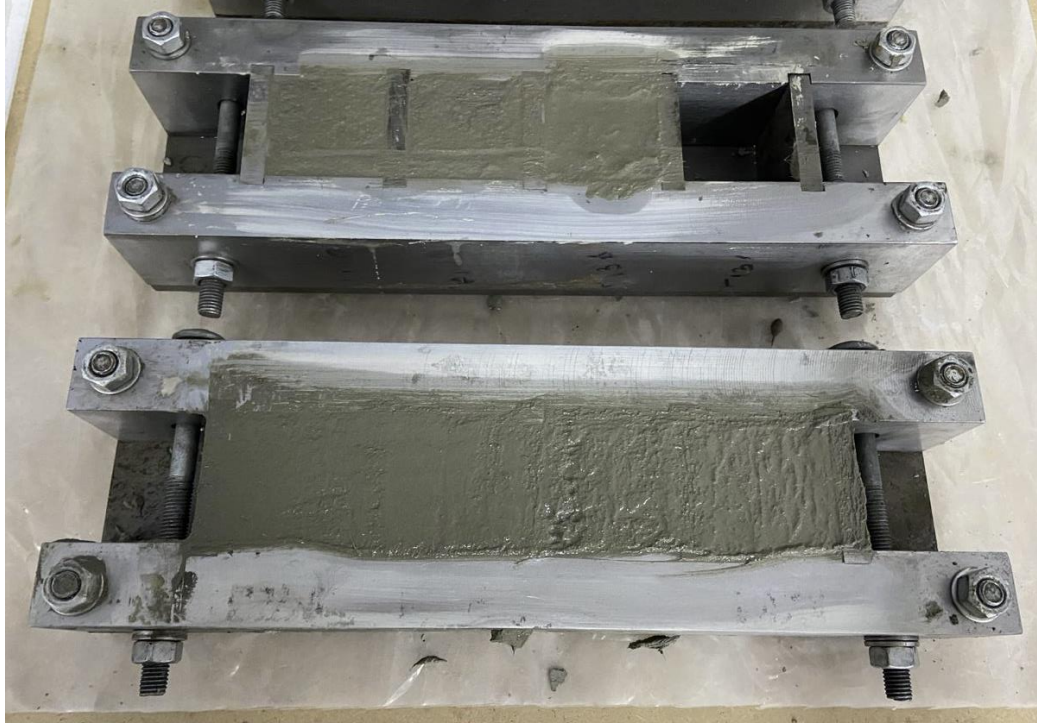
Figure 4-8 Compressive specimens cast in steel moulds
