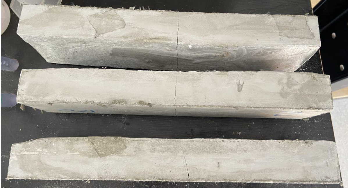
Figure 5-25 Flexural specimen failure patterns (100% Replacement)
