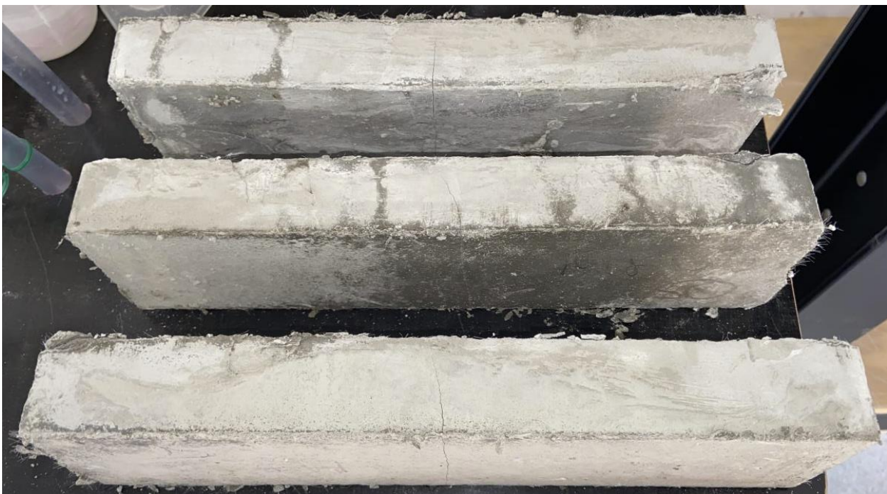
Figure 5-24 Flexural specimen failure patterns (50% Replacement)
