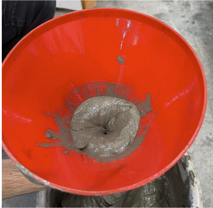
Figure 5-2 Control ECC mortar stuck in flow cone
