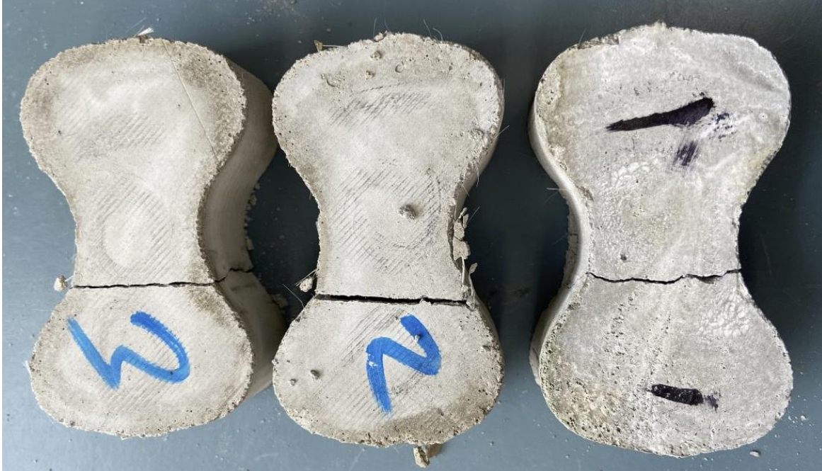
Figure 5-19 Tensile specimen failure patterns (100% Replacement)
