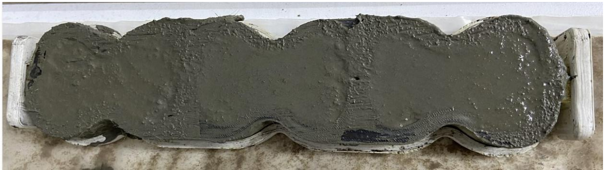
Figure 4-9 Tensile specimens cast in 3D printed gang mould
