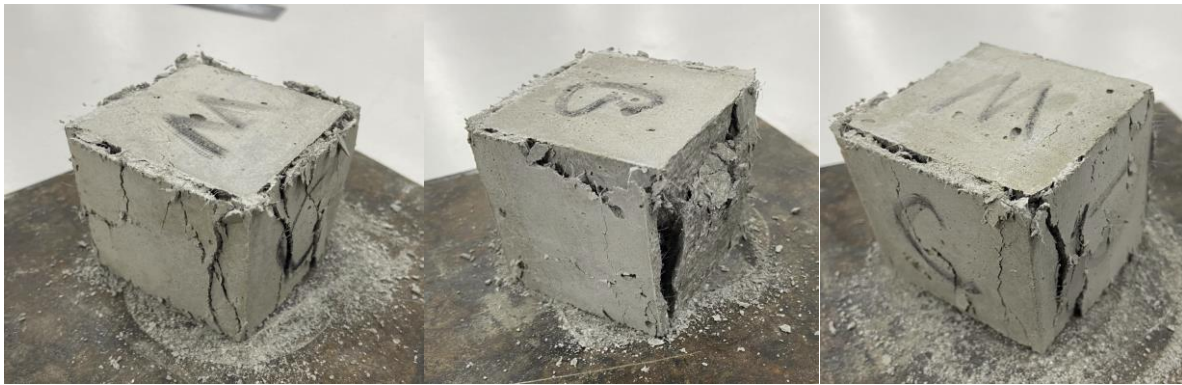
Figure 5-6 7-day compressive specimen failure patterns (Control)
