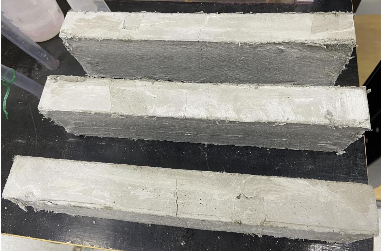
Figure 5-23 Flexural specimen failure patterns (25% Replacement)
