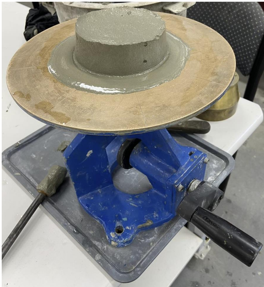
Figure 4-6 Mortar mini slump flow test: Control
