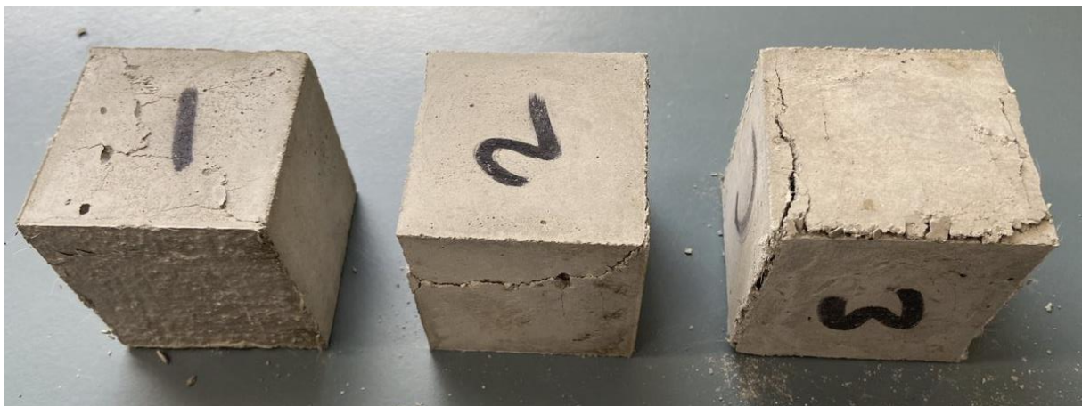
Figure 5-10 28-day compressive specimen failure patterns (Control)
