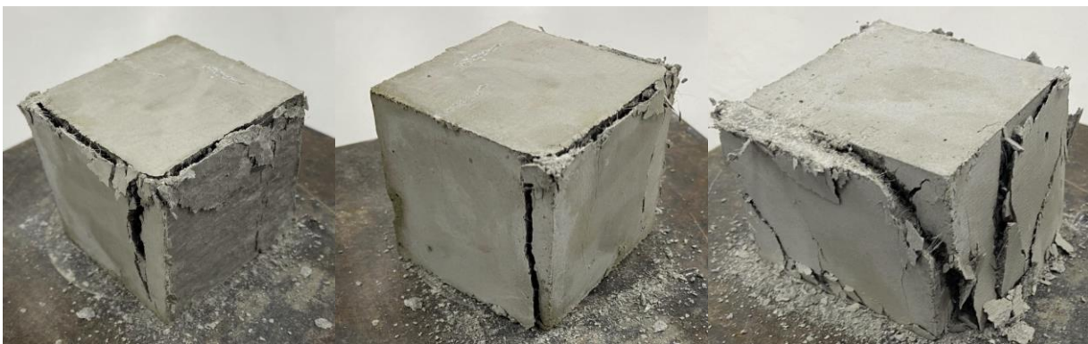
Figure 5-7 7-day compressive specimen failure patterns (25% replacement)
