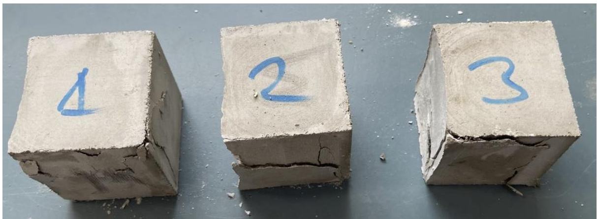
Figure 5-13 28-day compressive specimen failure patterns (100% replacement)
