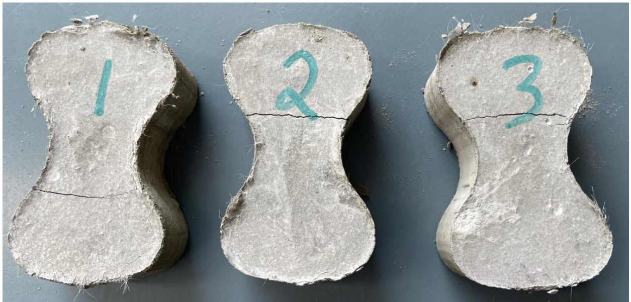
Figure 5-18 Tensile specimen failure patterns (25% Replacement)
