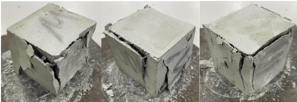
Figure 5-9 7-day compressive specimen failure patterns (100% replacement)
