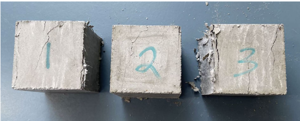
Figure 5-12 28-day compressive specimen failure patterns (50% replacement)
