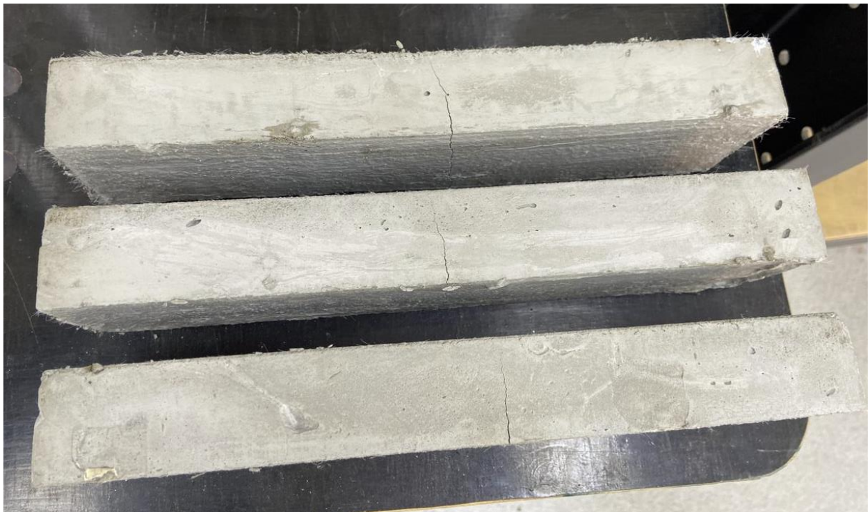
Figure 5-22 Flexural specimen failure patterns (Control)
