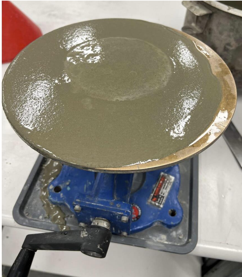
Figure 4-7 Mortar mini slump flow test: 100% Pond ash replacement
