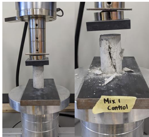
Fig. 27 (left) the compression testing machine prior to testing mix 1, and Fig. 28 (right) mix 1 after testing.
