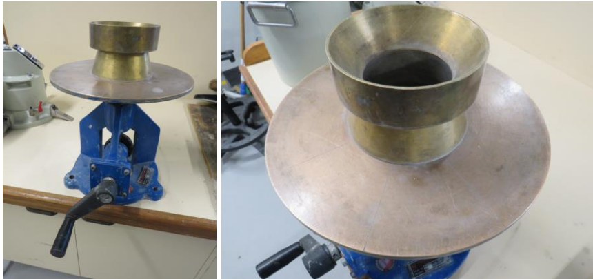
Fig. 17 (left) and 18 (right), illustrating the flow table apparatus and correct setup.
