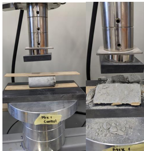
Fig. 29 (left) the indirect tensile testing machine prior to testing mix 1, and Fig. 30 (right) mix 1 after testing.
