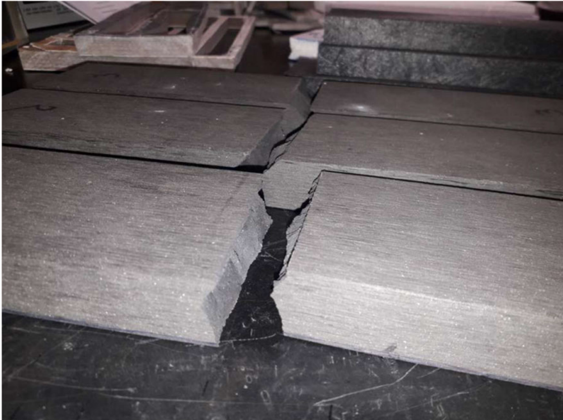
Figure 21: Failure of all three wood composite specimens.
