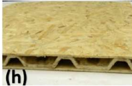
Figure 12: Composite wood sandwich panel structure by Mohammadabadi. (Mohammadabadi et al. 2020)
