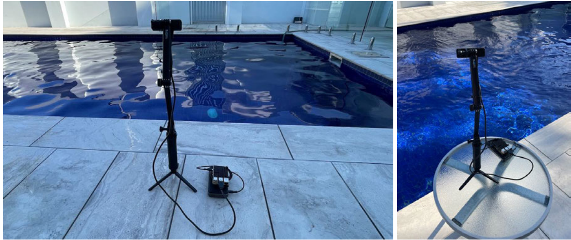
Figures 23a and b: The experimental setup with the Oak-D Lite, Raspberry Pi and power bank.
