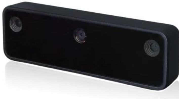
Figure 10: The Oak-D Lite edge AI camera. In the centre is the colour camera with two stereo cameras either side (Luxonis, 2023).
