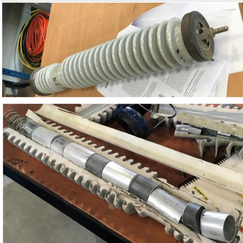
Figure 7 - 6: 33kV Gapless surge diverter with pressure relief and sectioned view EQL (2019).
