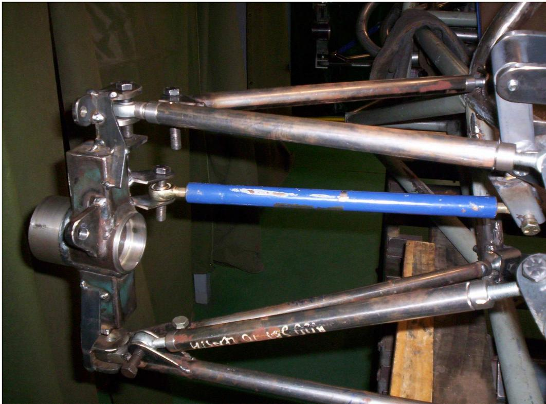
**Figure 2E Front Right Suspension Assembly**
