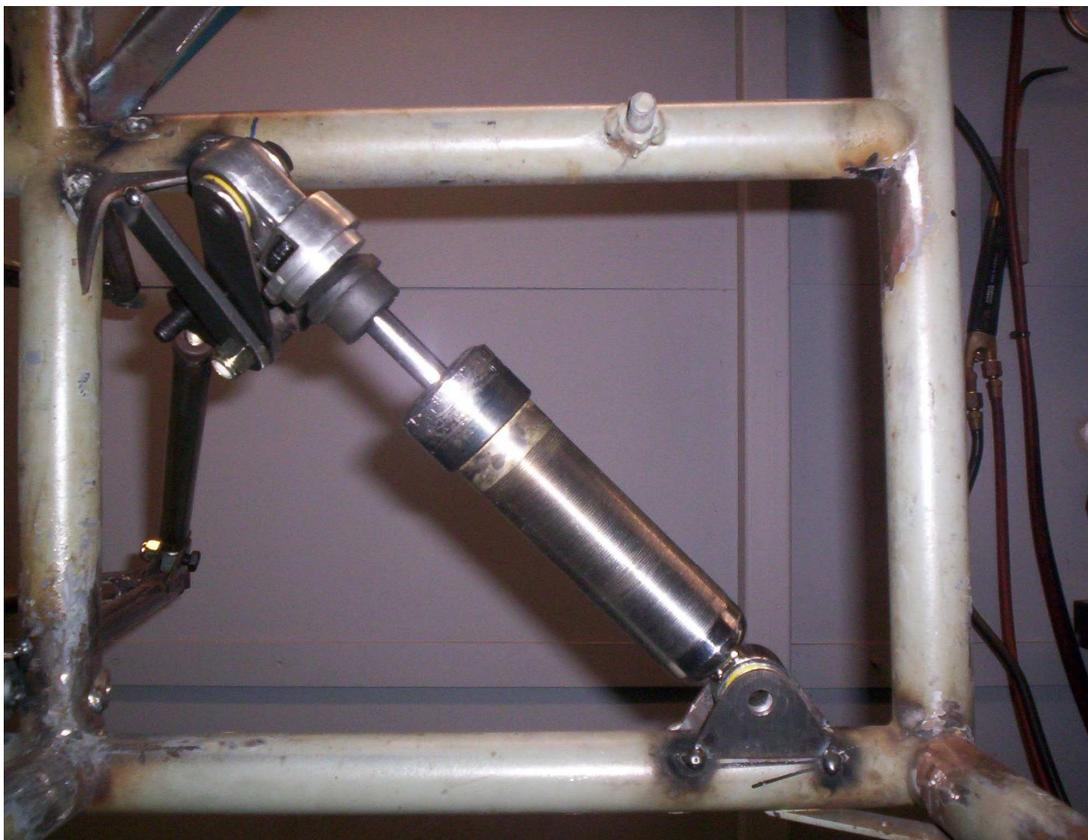
**Figure 5E Mounting Position of the Rear Shock Absorber on the Chassis**
