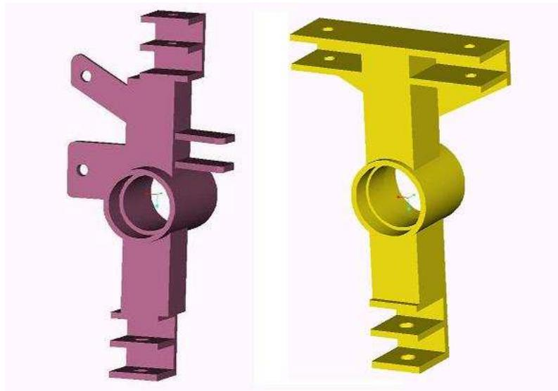
**Figure 34 2005 Front and rear final design**
