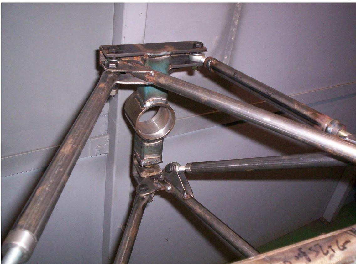
**Figure 3E Rear Suspension Assembly**
