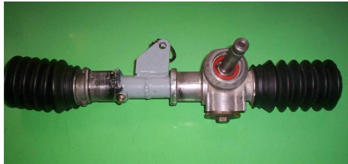
**Figure 28 Modified steering box assembly**
