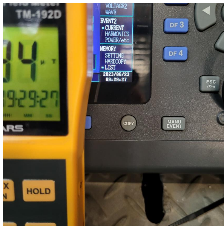
Figure 4.4.0.2 Confirmation of meter time synchronisation.
