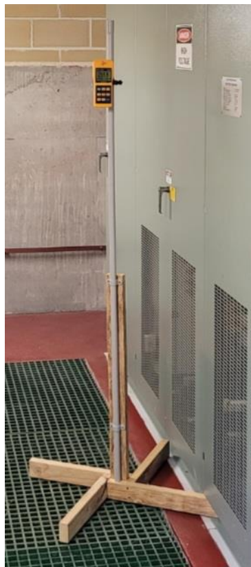
Figure 3.5.1 Adjustable Non-Conductive Stand for Magnetic Field Meter.
