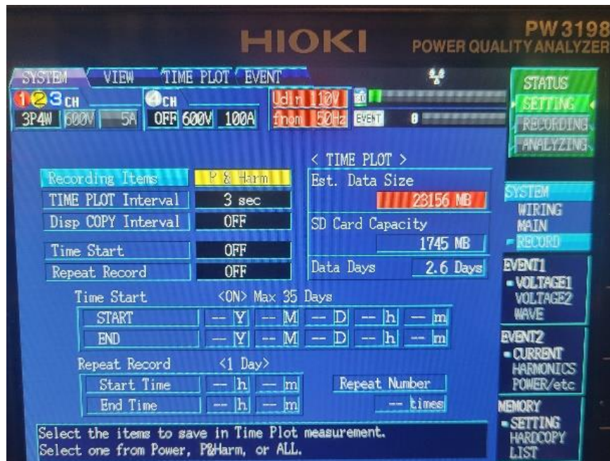
Figure 4.1.1b Power Analyser set for 3 second recording intervals.
