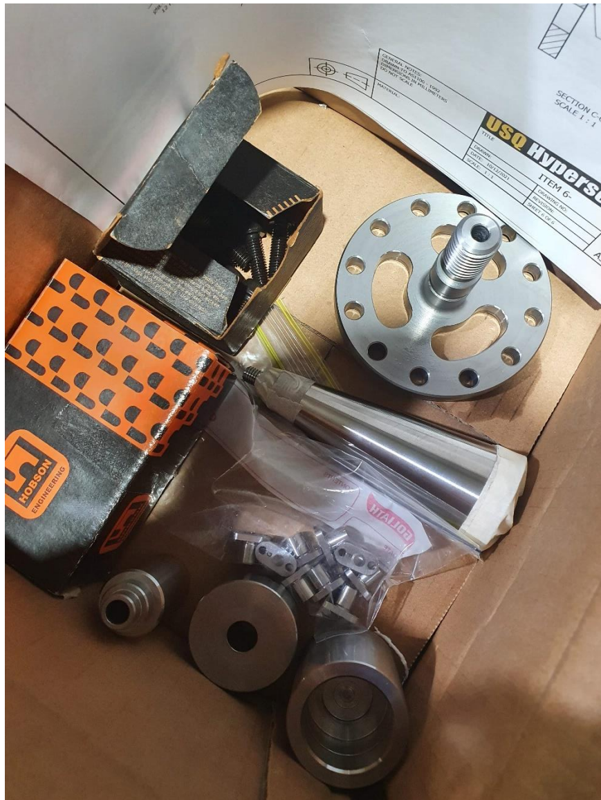
Figure F 4. Manufacturing process photo including intermediate frustrum, sting mount, upper rear frustrum inserts and fixture components.
