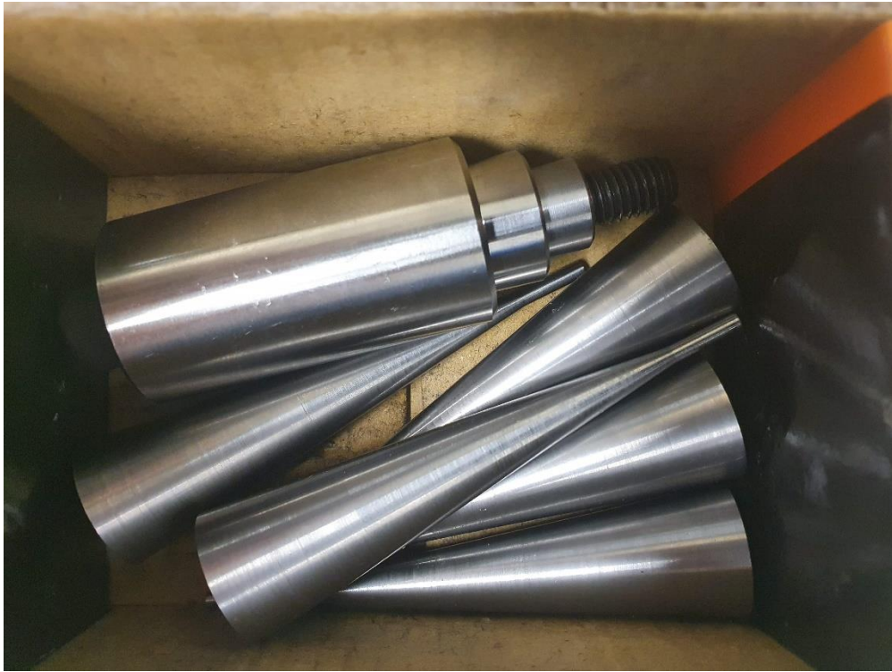
Figure I 1. Rough turned Nosetips prior to finish grinding including manufactured Nosetip fixture.
