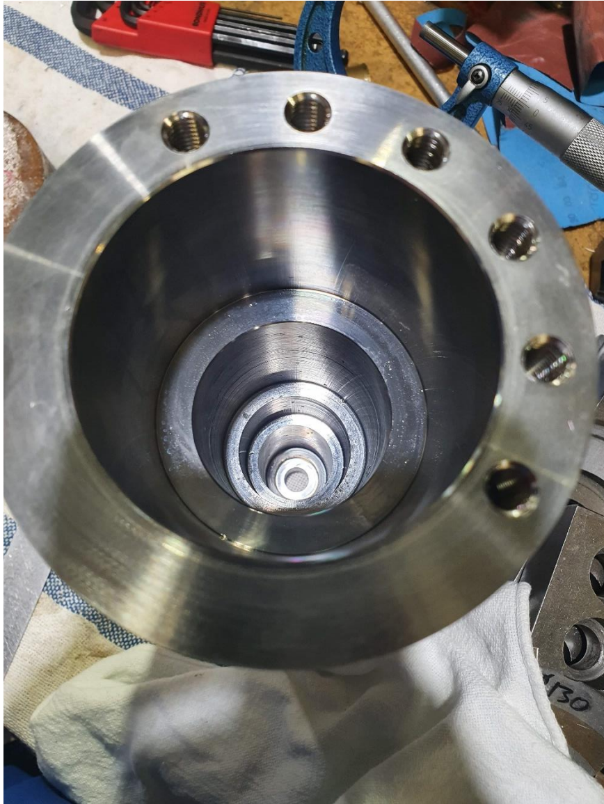
Figure F 5. In process photo of the upper rear frustrum prior to machining in half.
