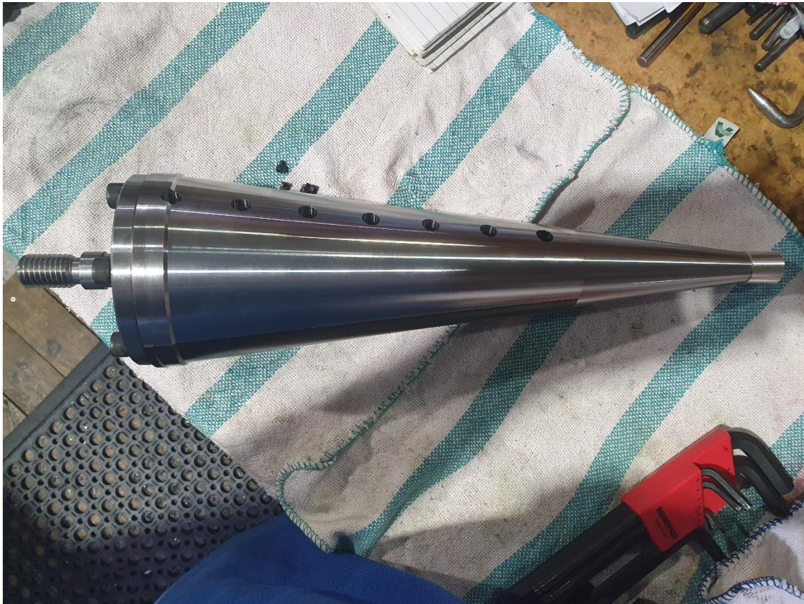
Figure F 7. Assembled rear frustums and intermediate frustum fitted with turning centre for 7 degree finish turning
