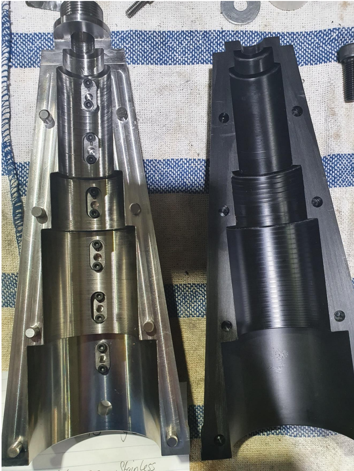
Figure F 6. Upper rear frustum with assembled inserts and dowel pins (left) Lower rear frustum machined from Acetal (right)
