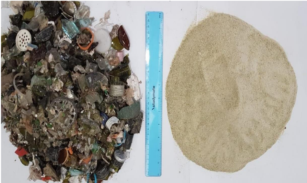
Figure 17 – Contaminated Glass Transformed into Recycled Glass Sand (iQRenew n.d.)
