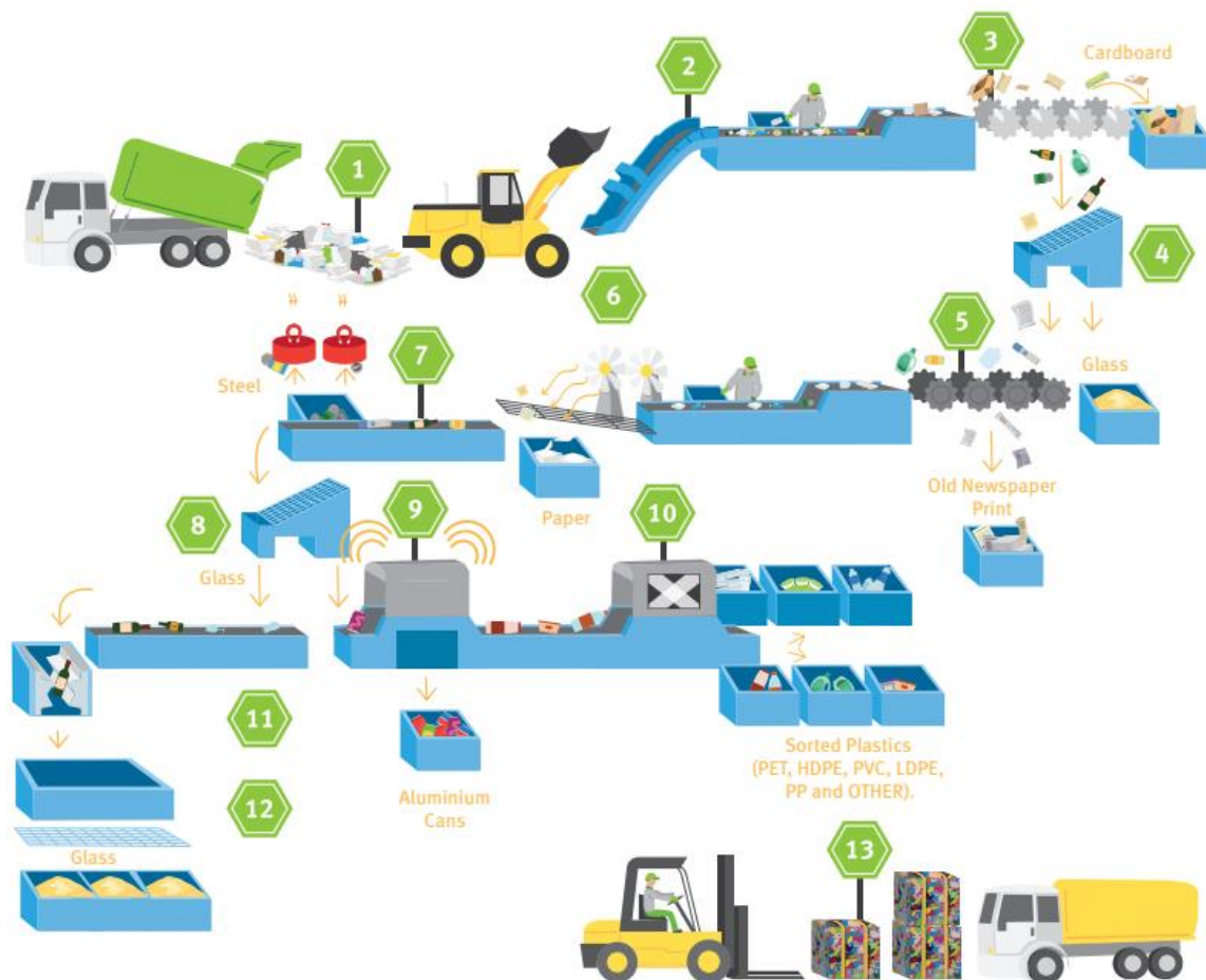
Figure 13 – Townsville MRF Recycling Process (Townsville City Council 2018)
