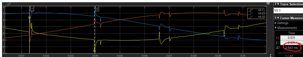
Figure 19. Travelling waveforms for the single-phase open circuit fault on the symmetric model. Time interval between first and second wave groups ( \Delta T ) displayed on right (2.643 ms).
