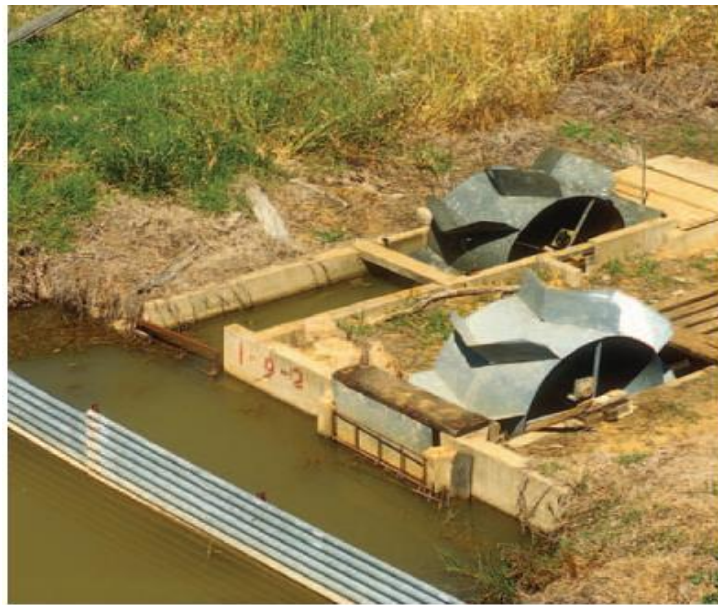
Dethridge wheel measuring irrigation water consumption, Griffith, New South Wales. Photo: Bill van Aken, CSIRO.
