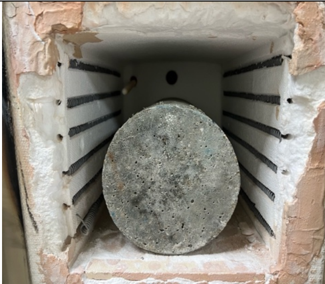
Figure 3.42: Sample Placed in Furnace for Fire Testing.
