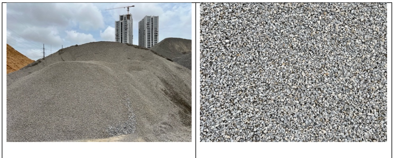
Figure 3.3: Coarse Aggregate 10mm, supplied by D-Mix, Karachi, Pakistan.
