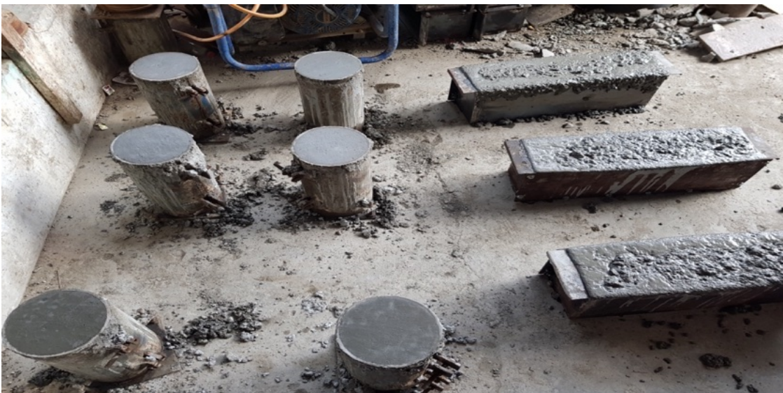
Figure 3.11: Moulds Being Poured with Concrete to prepare Samples
