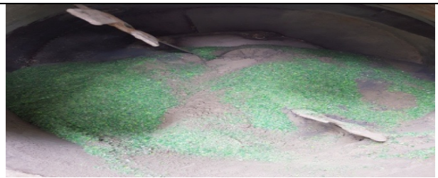
Figure 3.27: Plastic inside the concrete mixer being used as aggregate.
