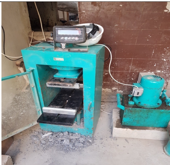
Figure 3.17: CTM setup for Flexural Strength Testing.
