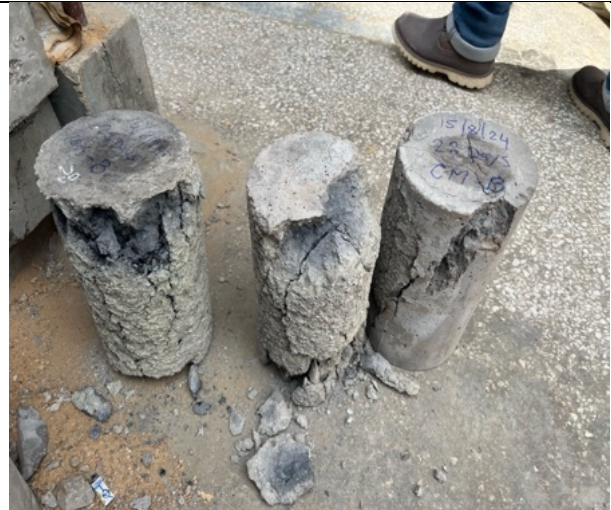
Figure 3.45: After Compressive Strength Testing.
