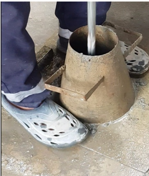
Figure 3.33: Slump Test Being Conducted.
