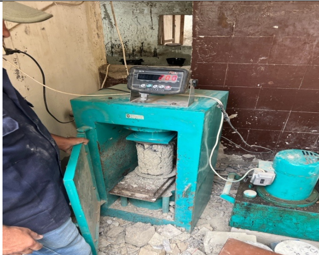
Figure 3.44: Compressive Strength Testing after removing from Furnace.
