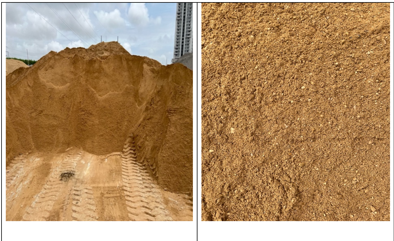
Figure 3.4: Bolari River Sand used as fine Aggregate, supplied by D-Mix, Karachi, Pakistan.
