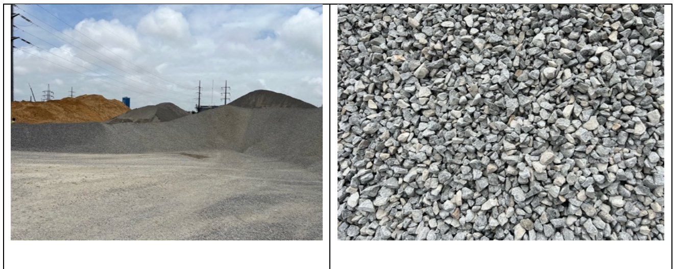
Figure 3.2: Coarse Aggregate 19mm, supplied by D-Mix, Karachi, Pakistan.
