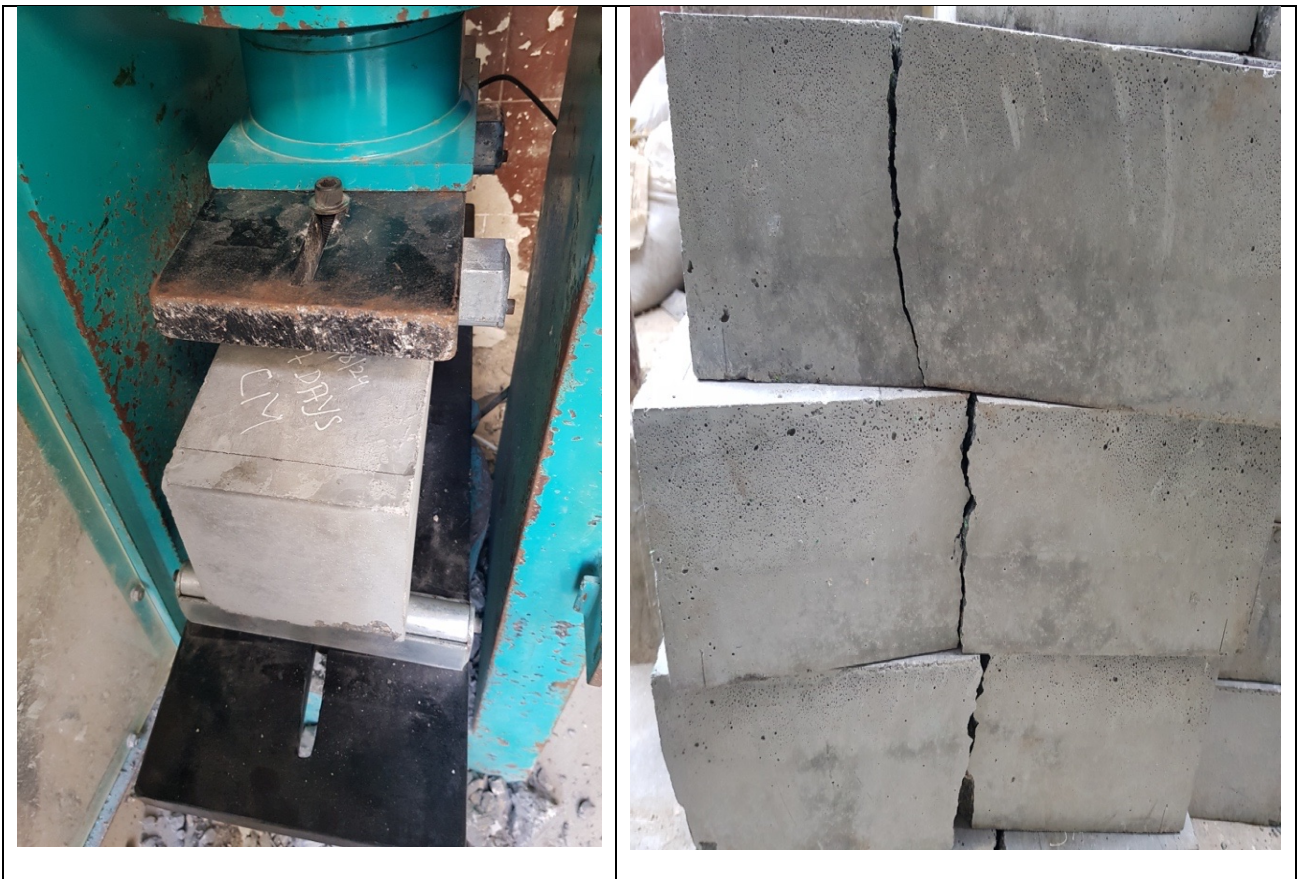
Figure 3.40: Flexural Strength Testing.
