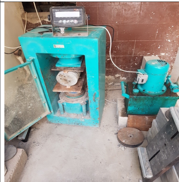
Figure 3.16: CTM setup for Split Tensile Strength.
