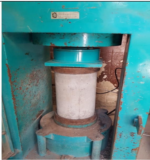
Figure 3.15: CTM setup for Compressive Strength.
