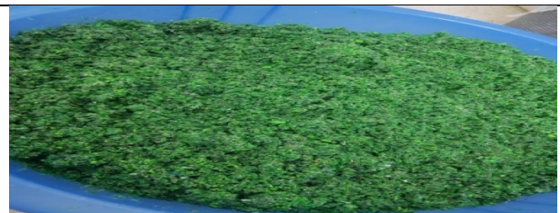
Figure 3.25: Plastic after Washing with water.
