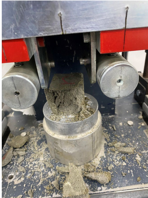
Figure 32 Sample C after compression testing
