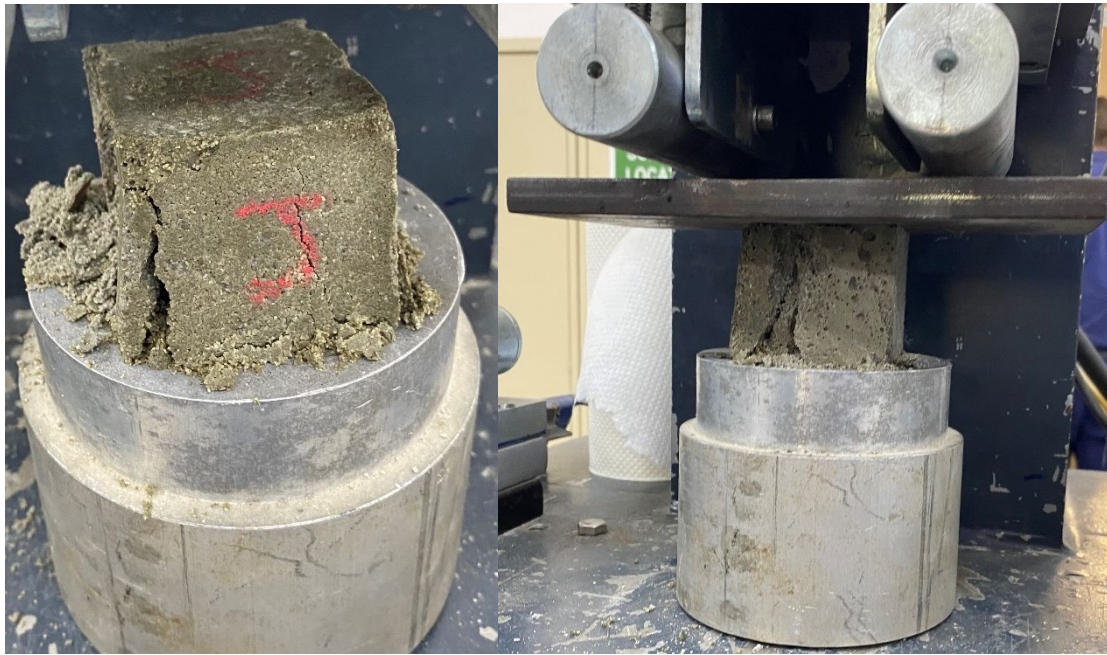
Figure 15 Cubic moulds after compression testing
