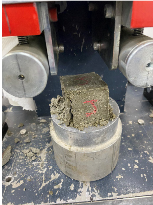
Figure 30 Sample A after compression testing
