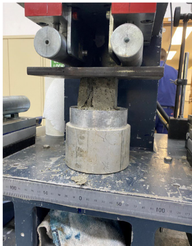
Figure 31 Sample B after compression testing
