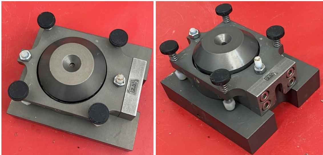
Figure 16 Shear box with a sample inside before being placed in ShearTrac2 machine
