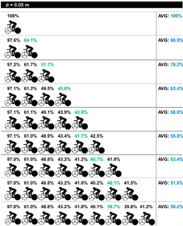
Fig. 9. Drag of every rider in pacelines of 2 up to 9 riders, as a percentage of the drag of an isolated rider. Wheel-to-wheel distance d = 0.05 m. Right column gives average drag percentage for the whole paceline.
