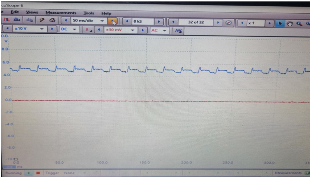
Figure D.12: Unsatisfactory PWM signal displayed on Picoscope.
