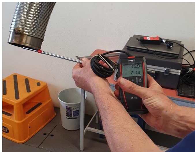
Figure 20 - Testing the airflow rate of the exhaust extraction system
