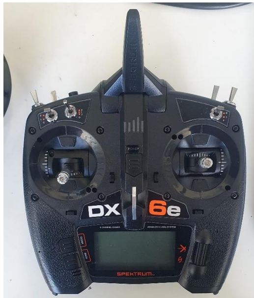
Figure 25 – Spektrum 6-Channel Transmitter; utilised for K60TPG4 engine control.
