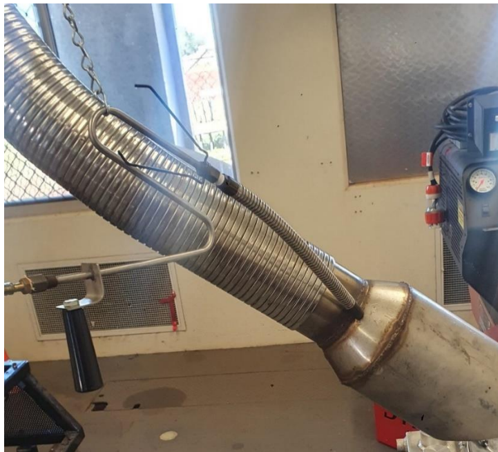
Figure 22 - Emissions sample probe placement
