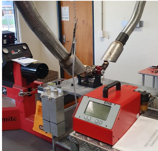
Figure 33 - EMS Model 5002 exhaust gas analyser connected to exhaust extraction duct
