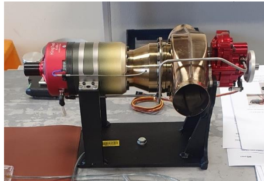
Figure 18 - K60TPG4 attached to support stand on test bench
