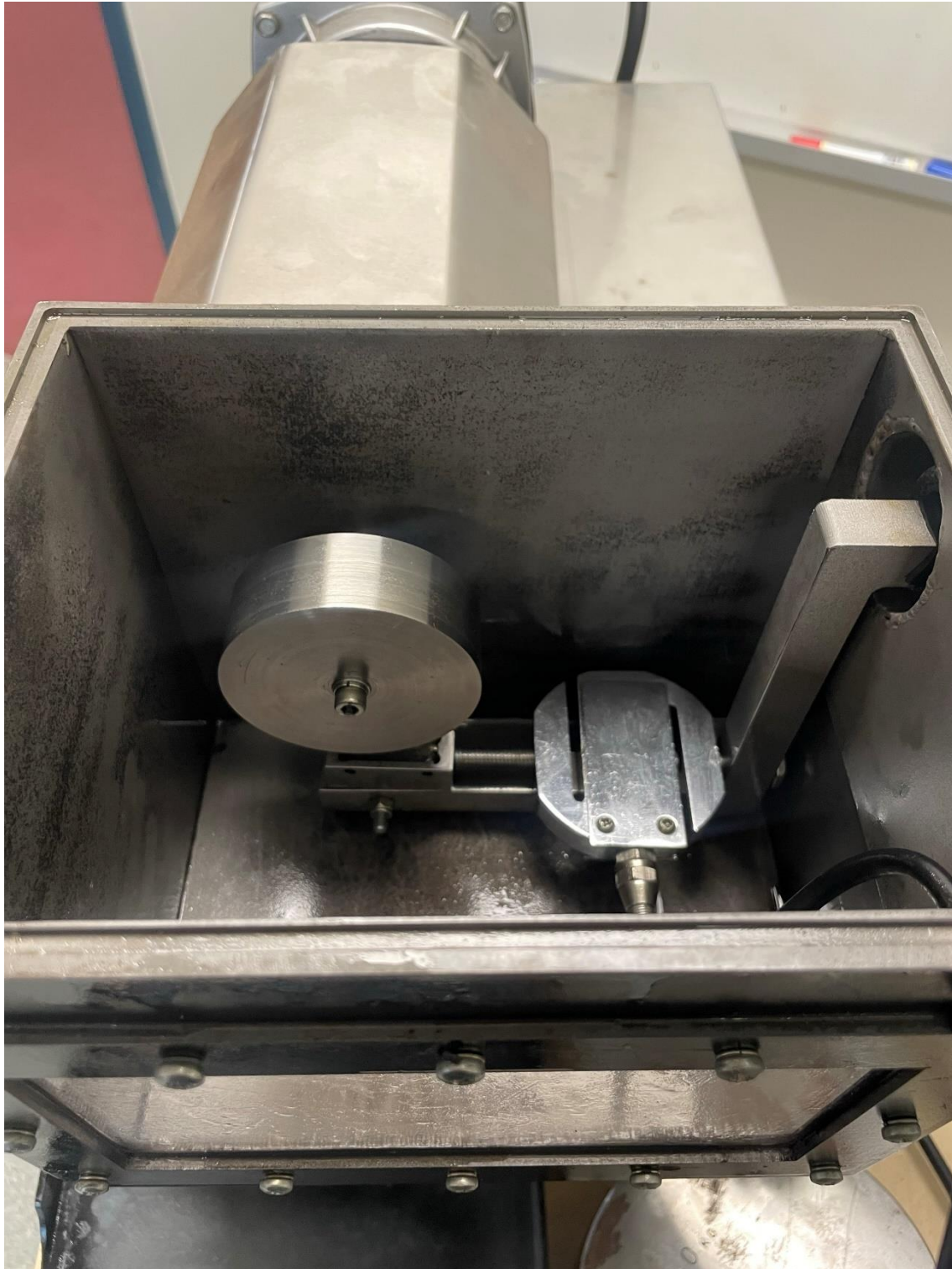
Figure 44: The countersurface, load cell and sample holder inside the tribology machine
