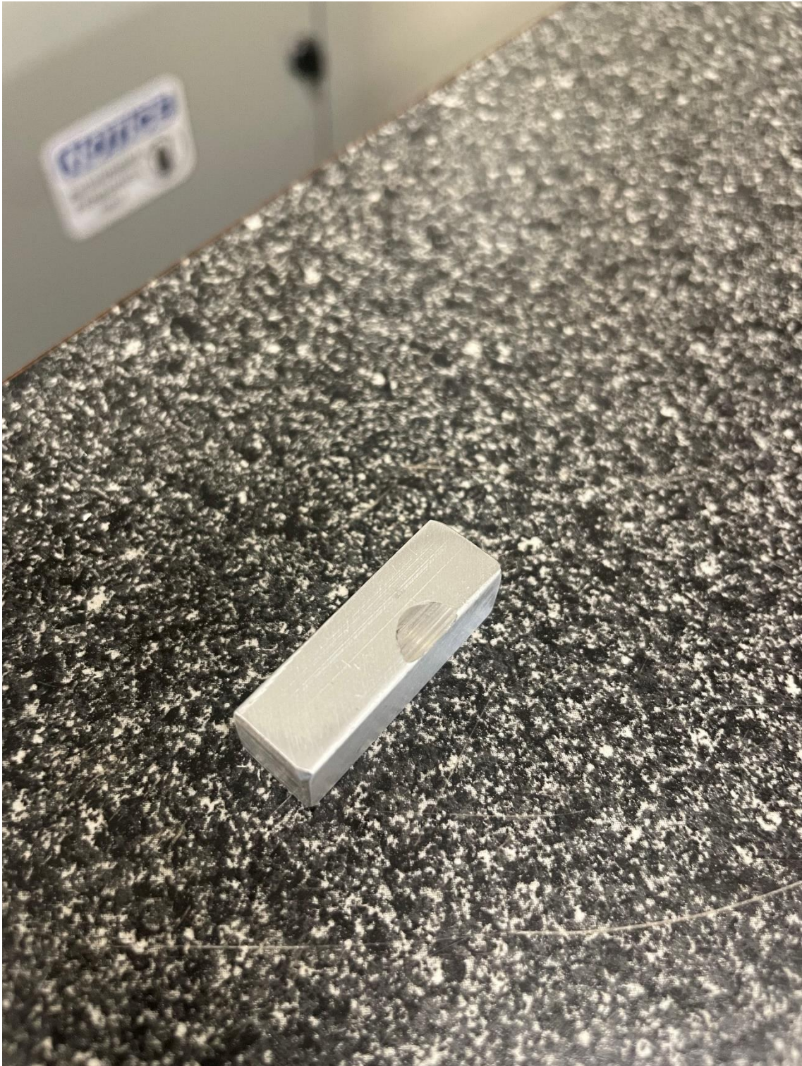
Figure 48: A typical wear scar left after testing in the tribology machine
