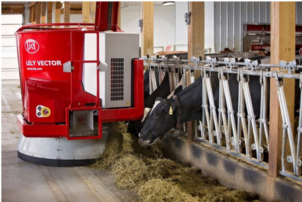
Figure 9: Autonomous Feed Robot - Lely Vector in action - (Lely, n.d.)
