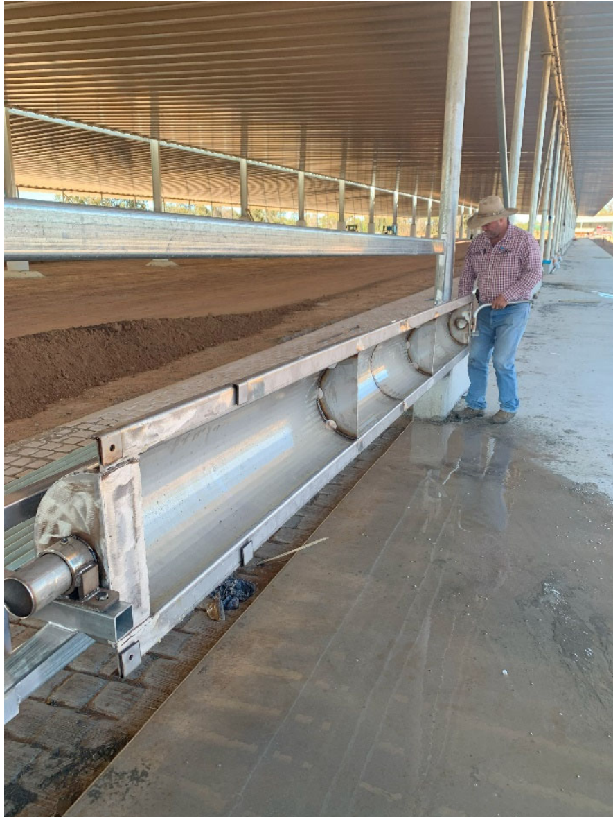
Figure 76: First prototype - Tipping mechanism in action
