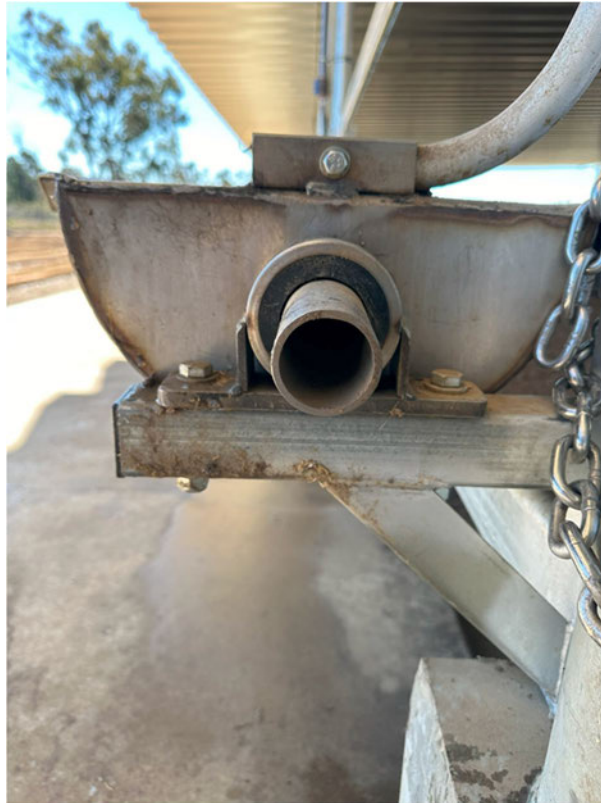
Figure 91: Final prototype water trough – Axle and axle hub
