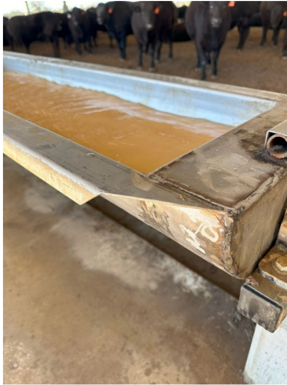
Figure 93: Final prototype water trough - Construction and welds
