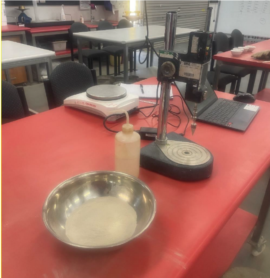
Figure 50: Equipment used for liquid limit test (Cone Penetrometer).
