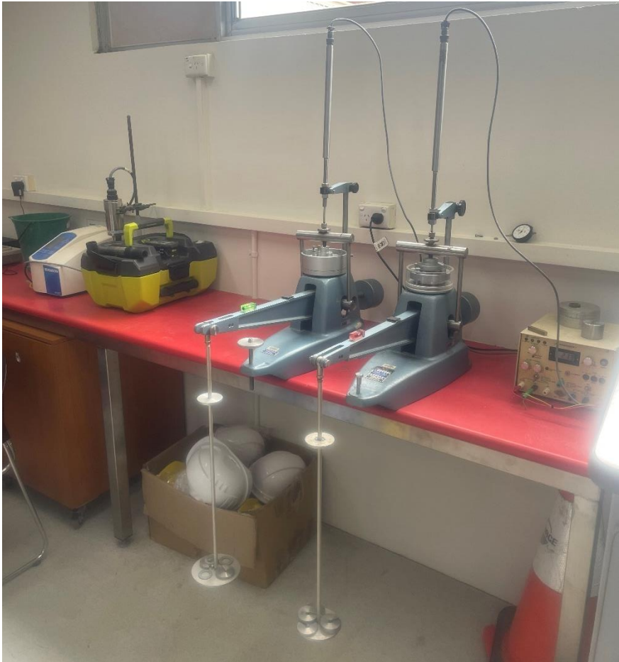
Figure 55: Soil consolidation test set up with consolidation cells loading and weights applied.
