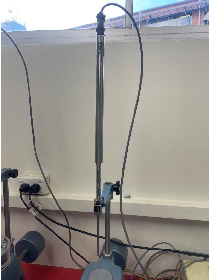
Figure 57: LVDT (Linear variable displacement transformer) connected to soil consolidation testing equipment.
