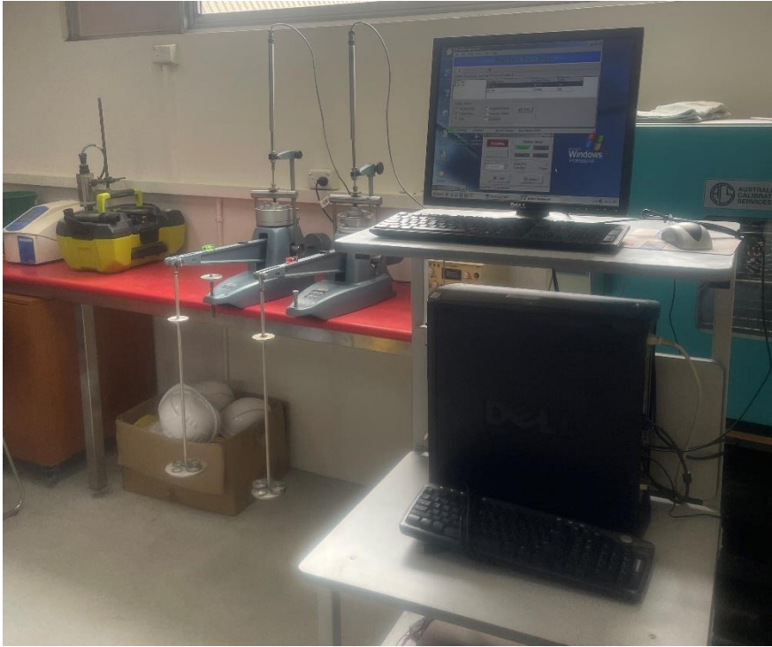
Figure 56: Complete recording set up for soil consolidation tests including LVDT and Vishay system 5000 data logger.
