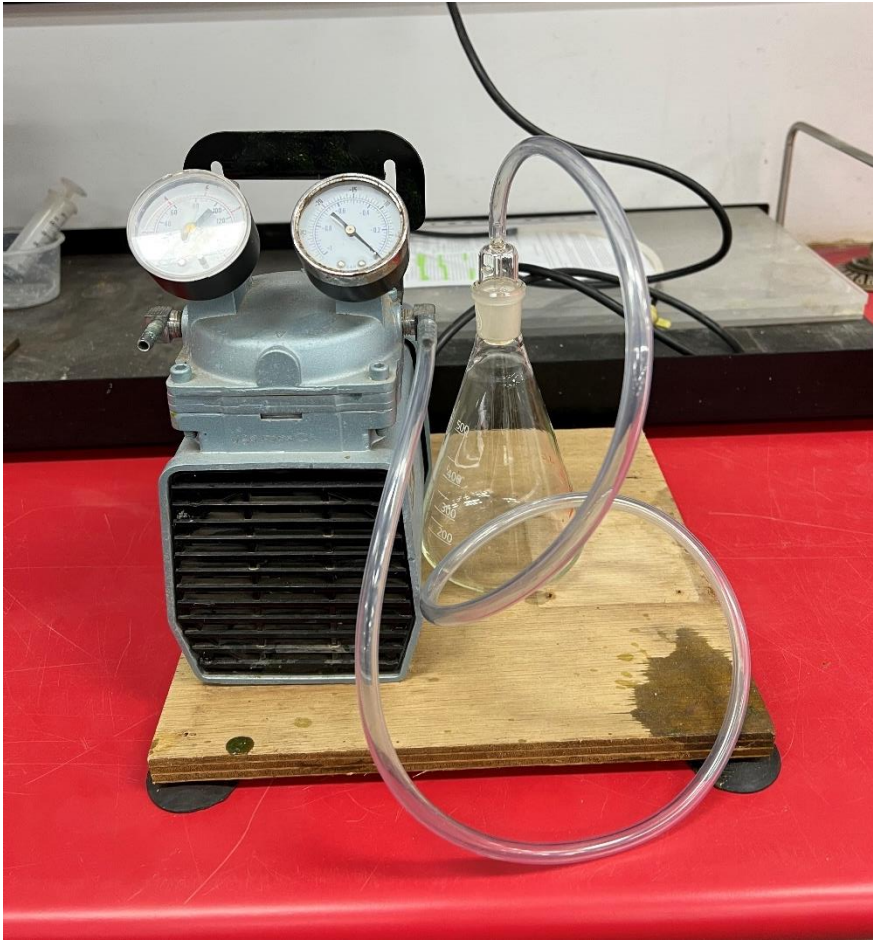
Figure 52: Vacuum pump used for specific gravity testing.
