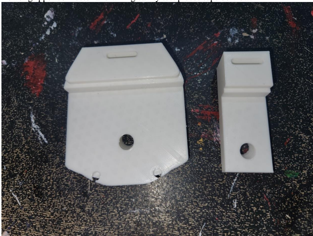
Lower gripper connector and wiring cavity test pieces topside view.
