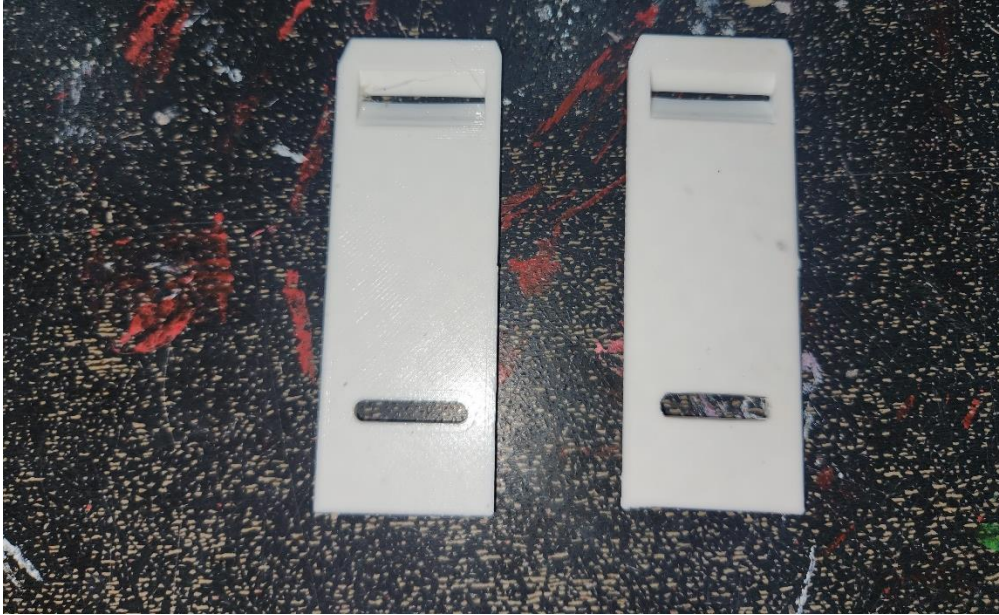
Attachment connector and gripper indentation alignment test piece.
