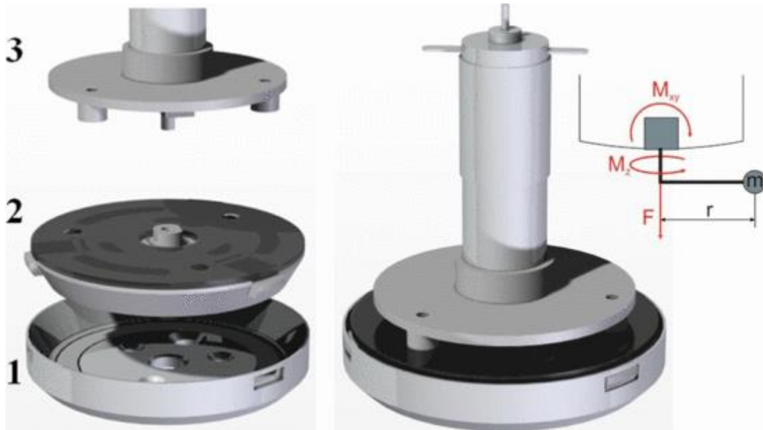
Figure 8 1) Tool base plate, 2) Master side, 3) Servo drive (Gyimothy & Toth 2011 pp. 1046-1051)
