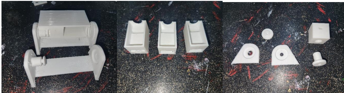
Figure 15 Jaw axle test (left), Servo top cavity test (middle), Jaw pivot tests (right)
