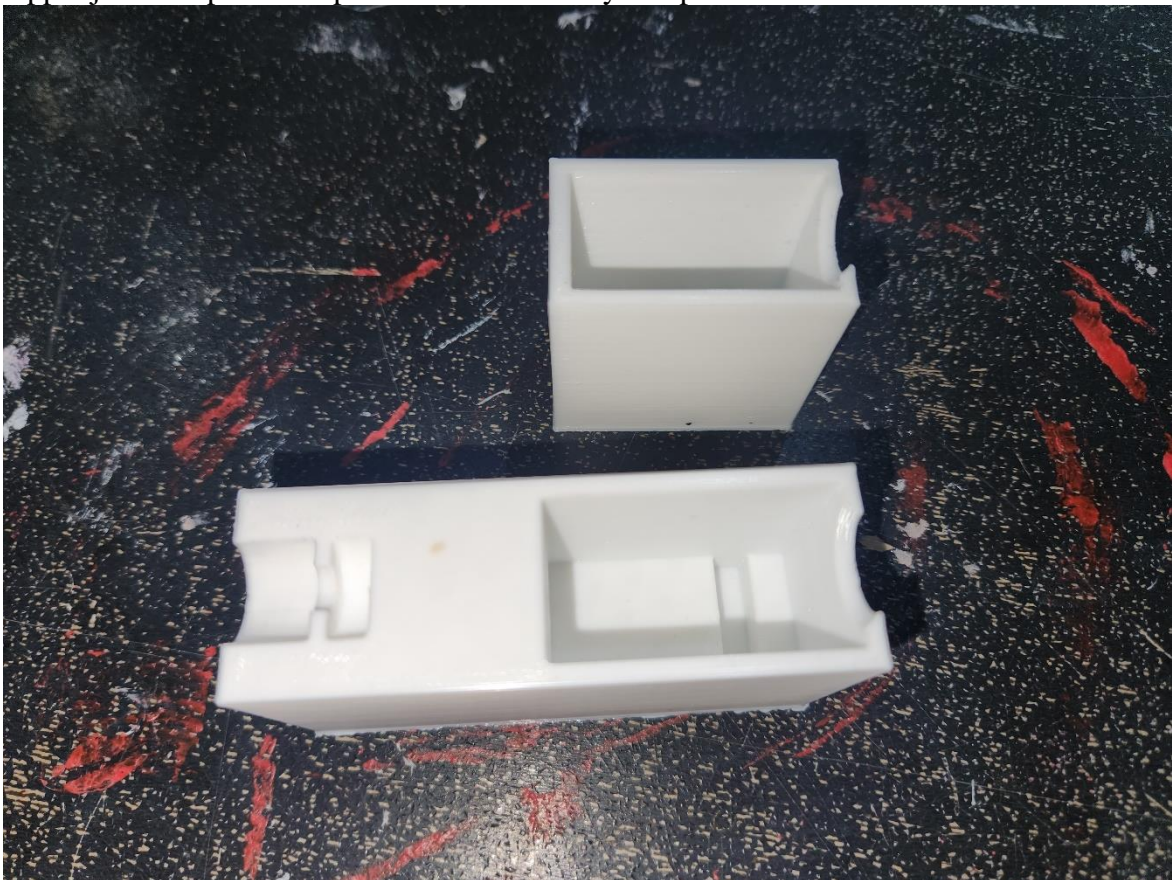
Upper jaw axle pivot test piece and servo cavity test piece.
