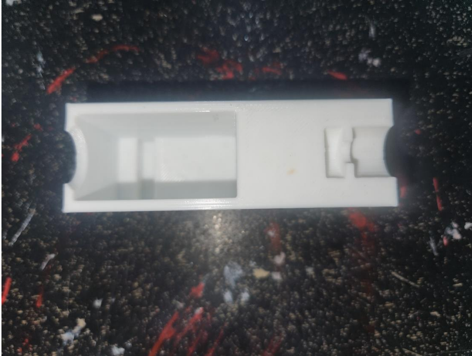
Upper jaw axle pivot test piece. Servo hole on the left, axle cavity on the right.
