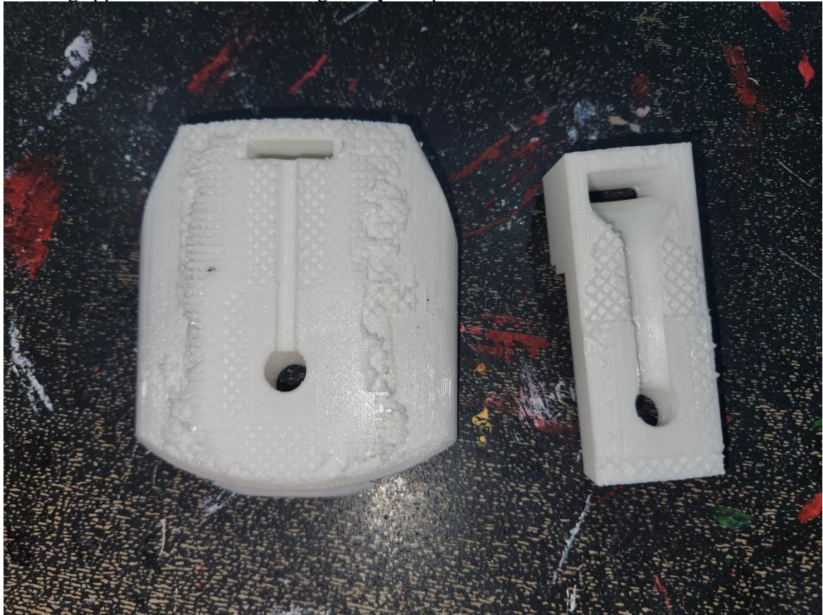
Lower gripper connector and wiring cavity test pieces underside view.
