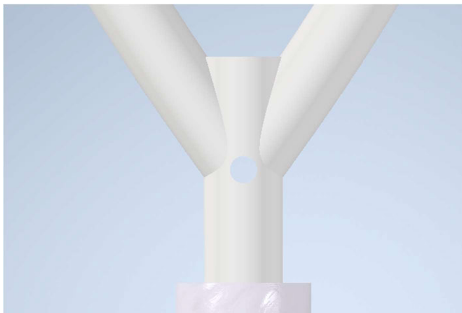
Figure 24: Example of the Single-Axis Point of Pivot – Pin Locked (Close Top View)
