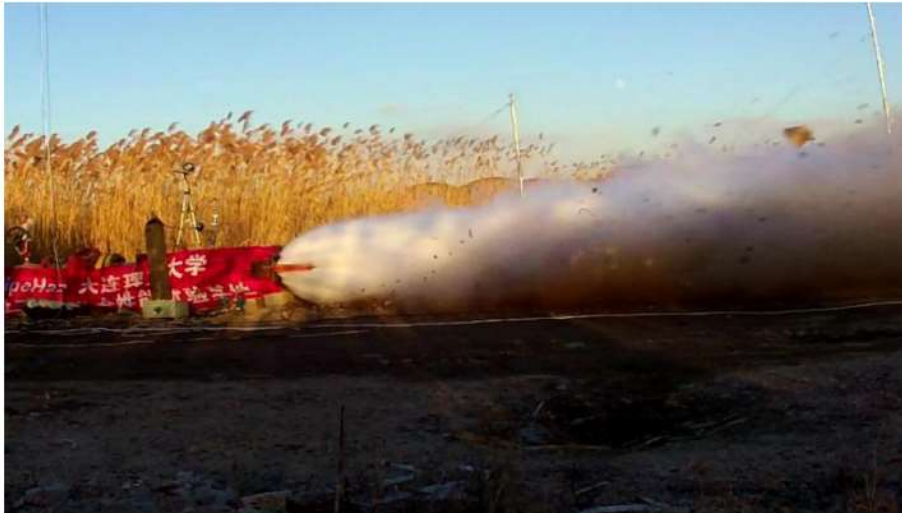
Figure 7 - CO 2 PipeHaz project, a high-velocity CO 2 jet resulting from a complete rupture release test (Woolley, Fairweather, Wareing, Falle, et al. 2014).
