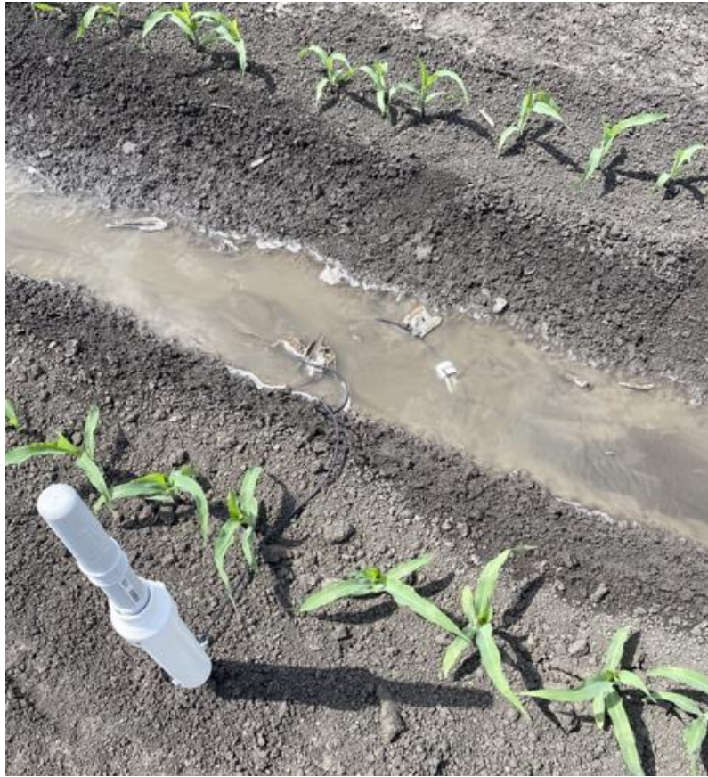
Figure 4.18 A submerged moisture probe attached to the advance sensor housing unit to measure and record water movement.
