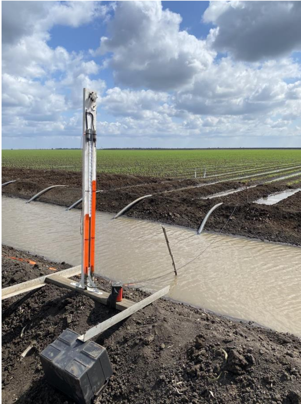
Figure 4.11 Using concepts of hydraulic head in measuring instrumentation to calculate flowrate for each furrow.
