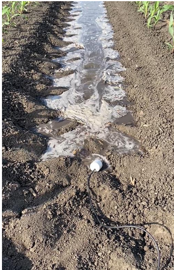
Figure 4.17 Moisture sensor probe being submerged by the advance wave during the field trial.
