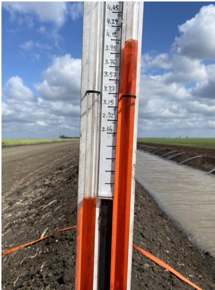
Figure 4.12 Image of the difference in head for a furrow to calculate the individual flowrate.
