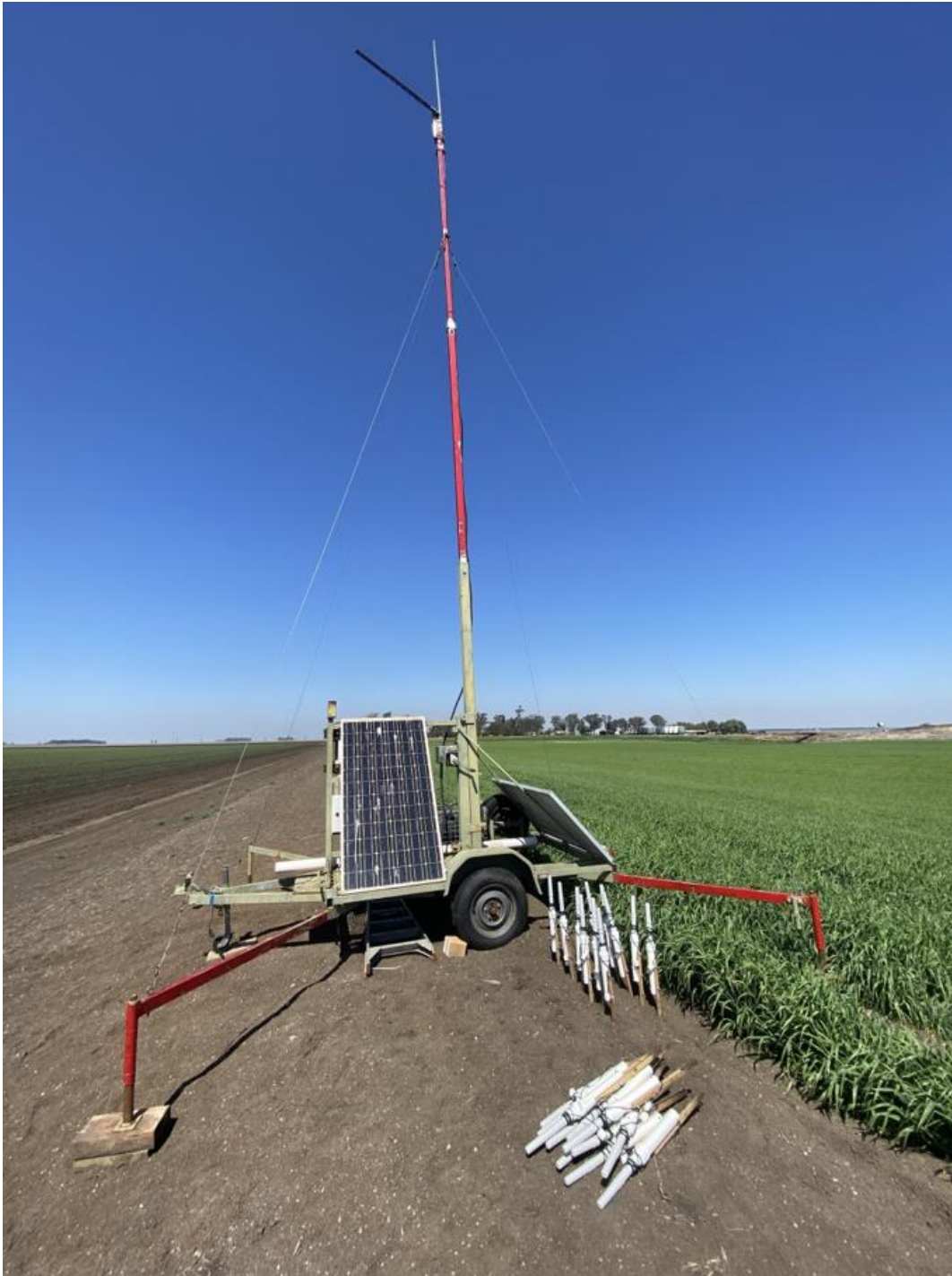
Figure 4.13 Taggle tower unit setup at Struanville Farming Co to receive and transmit advance data.
