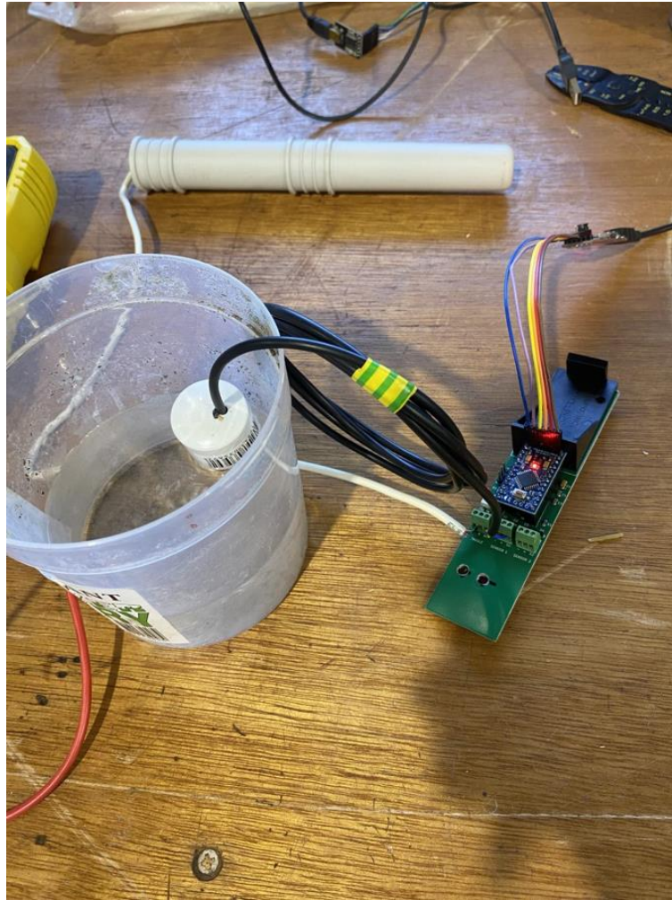
Figure 3.3 Uploading of Arduino code to control moisture sensor from computer and testing device for response in a container of water.
