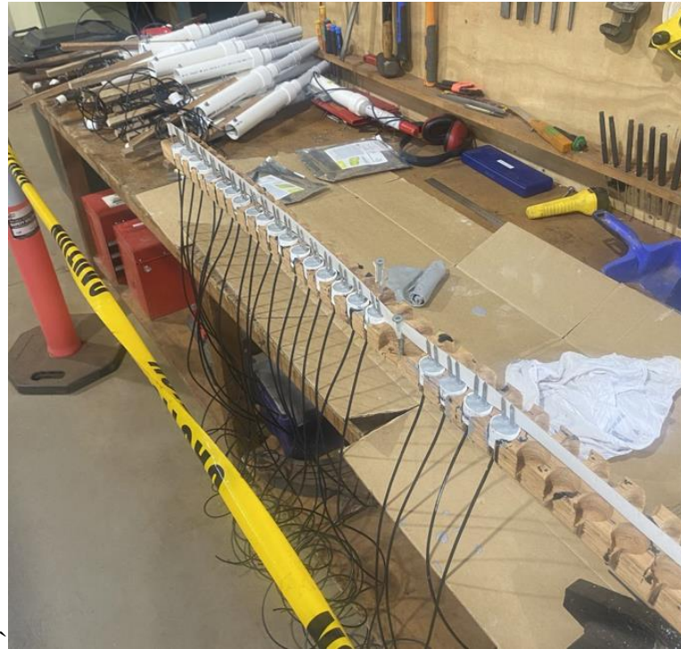
Figure 3.1 Visual depiction of integrating moisture probes into PVC casing for advance furrow sensors.
