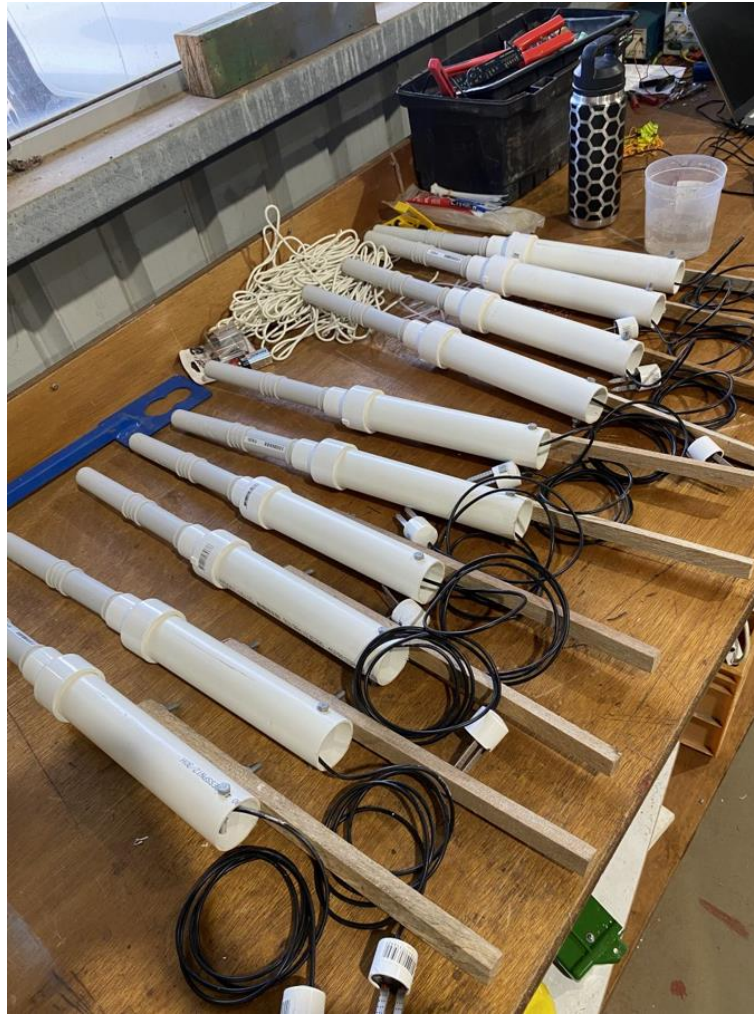
Figure 3.4 Final encasing of electronic components in a PVC housing unit connected to a wooden stake to position in the field.
