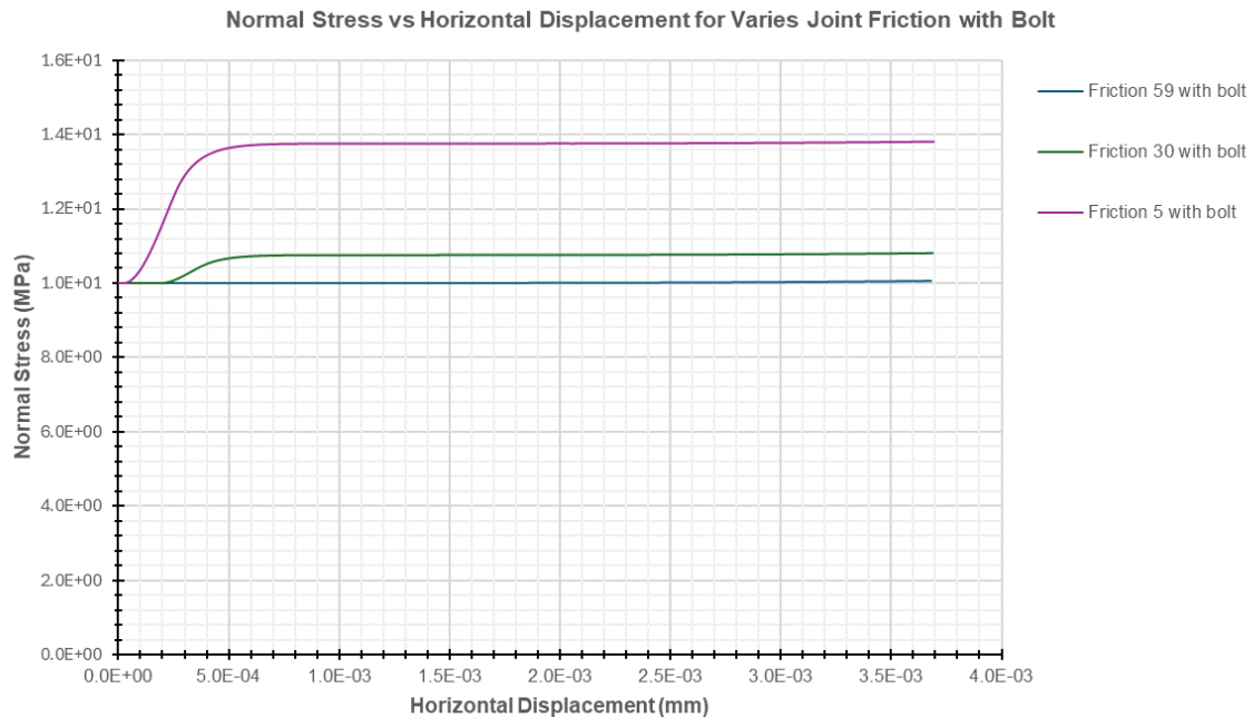
Figure 81: Presents the graph of Normal Stress vs the Horizontal Displacement for varies Joint Friction
