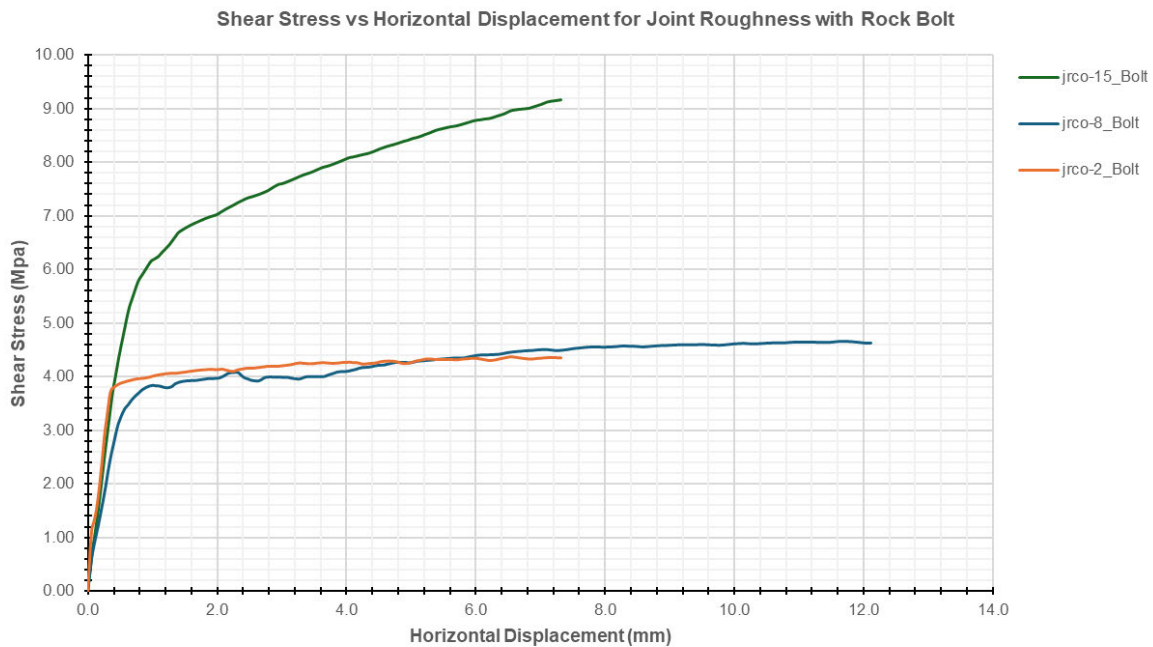
Figure 84: Presents the graph of Shear Stress vs the Horizontal Displacement for varies Joint Roughness
