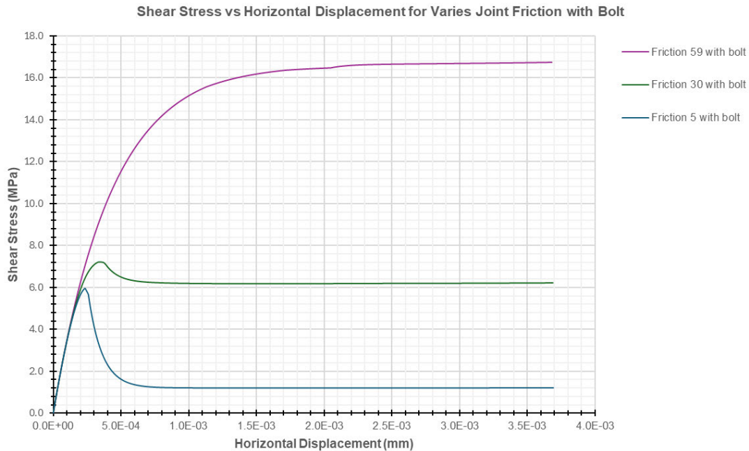
Figure 80: Presents the graph of Shear Stress vs the Horizontal Displacement for varies Joint Friction
