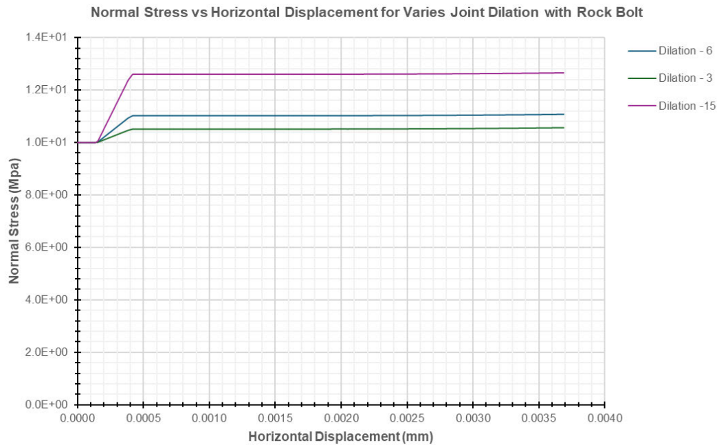
Figure 73: Presents the graph of Normal hear Stress vs the Horizontal Displacement for varies Joint Dilation
