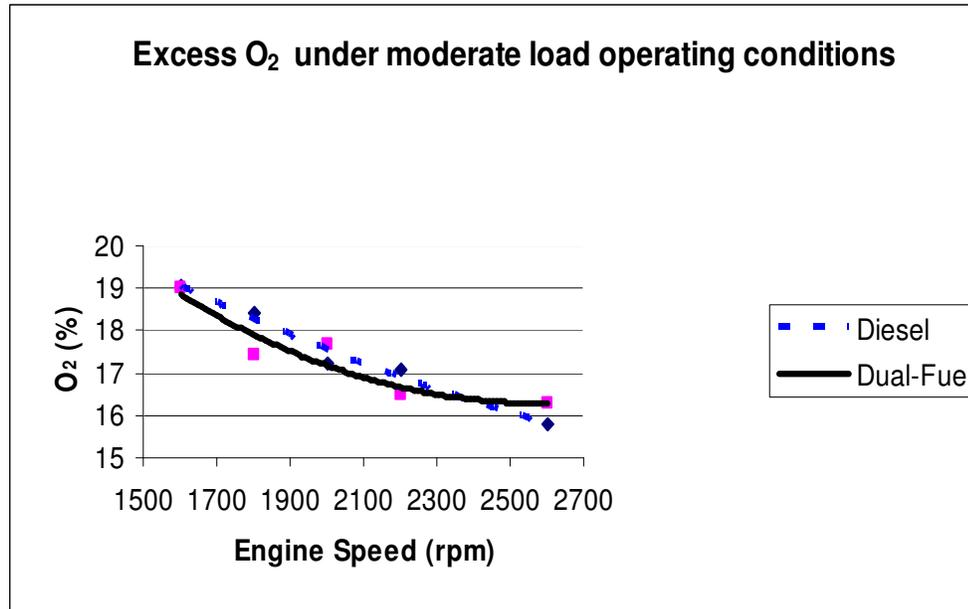
**Figure 6.22:** *Excess of O<sub>2</sub> under moderate load operating conditions*
