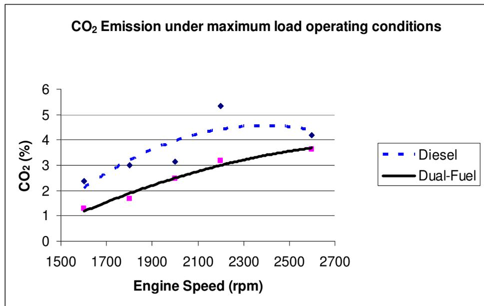
**Figure 6.10:** Emission of CO<sub>2</sub> under maximum load operating conditions
