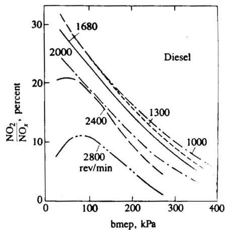
**Figure 4.2:** Ratio of NO<sub>2</sub> to NO in diesel exhaust for varying engine load and speed (Heywood, 1988)
