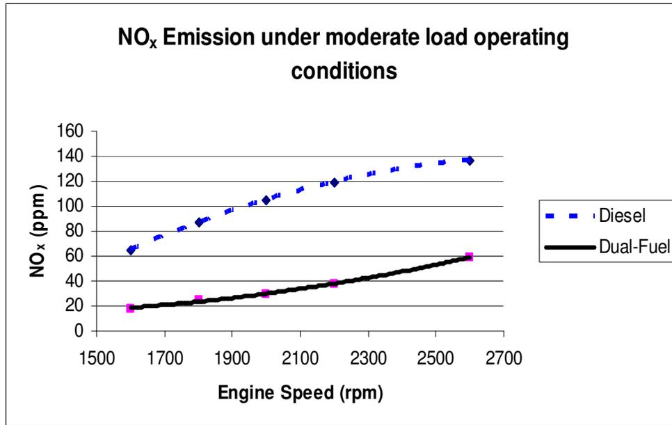
**Figure 6.20:** Emission of NO<sub>x</sub> under moderate load operating conditions
