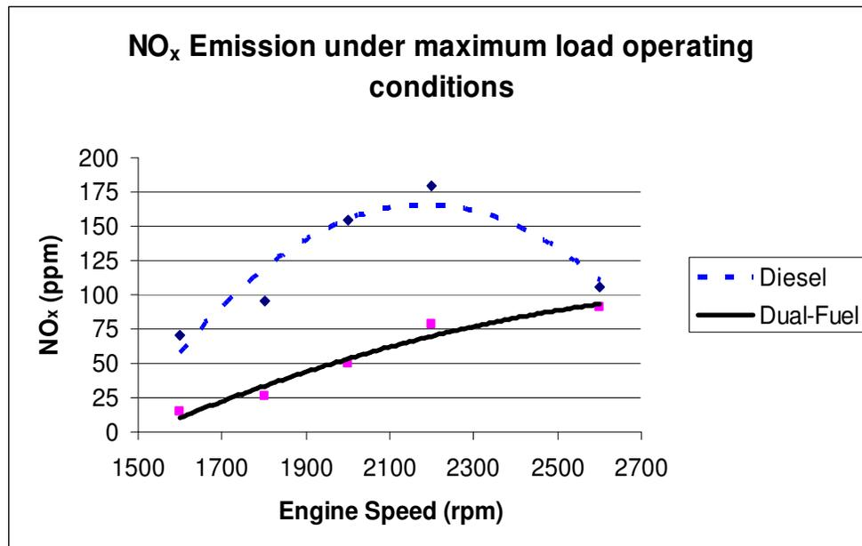
**Figure 6.9:** Emission of NO<sub>x</sub> under maximum load operating conditions
