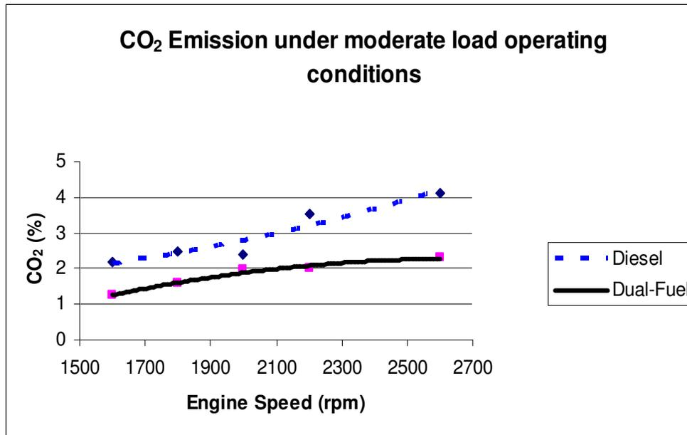
**Figure 6.21:** Emission of CO<sub>2</sub> under moderate load operating conditions
