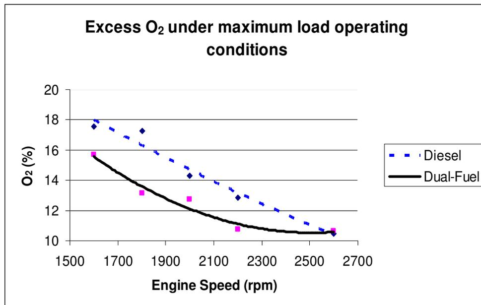
Figure 6.11: Excess of O<sub>2</sub> under maximum load operating conditions
