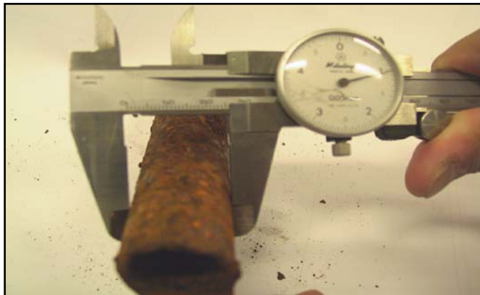
Figure 4..3.4.3 : Specimen Corrosion Thickness Measurement for Boiler # 2
