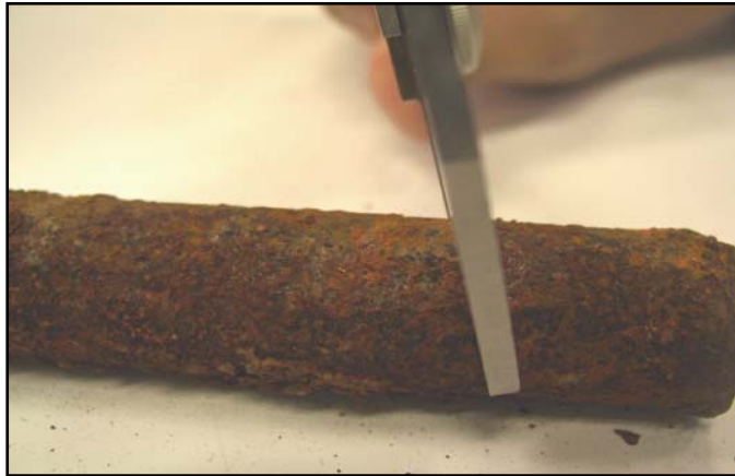
Figure 4.3.4.2 : Specimen Corrosion Thickness Measurement for Boiler # 1
