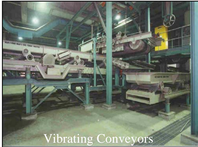
Figure 1.3.2.1A: Overview of ashes and scraps are separated and transported to the respective pit before loading onto the truck by overhead crane.
