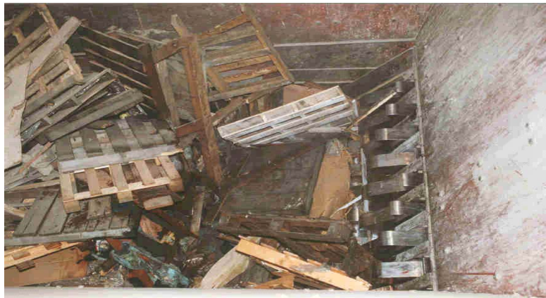
Figure 1.3.1.4 b: Rotary and Cutter Shear cut and crush bulky wastes
