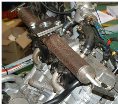
Figure 6.32 Prototype log type intake manifold.
