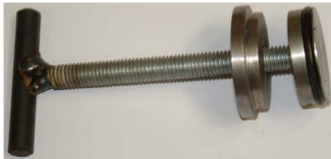
Figure 6.33 Prototype intake manifold buffer end adjuster.
