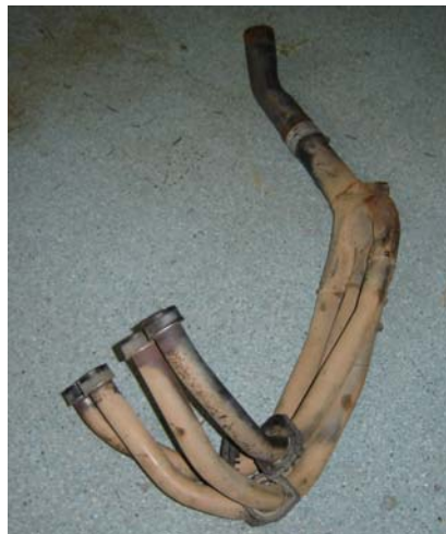
Figure 6.47 The original FZR extractor system.
