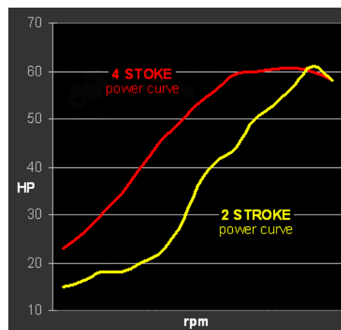
Figure 4.4 Comparison of two-stroke and four-stroke power curves.
