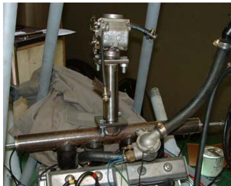
Figure 6.45 The Formula SAE induction system,
